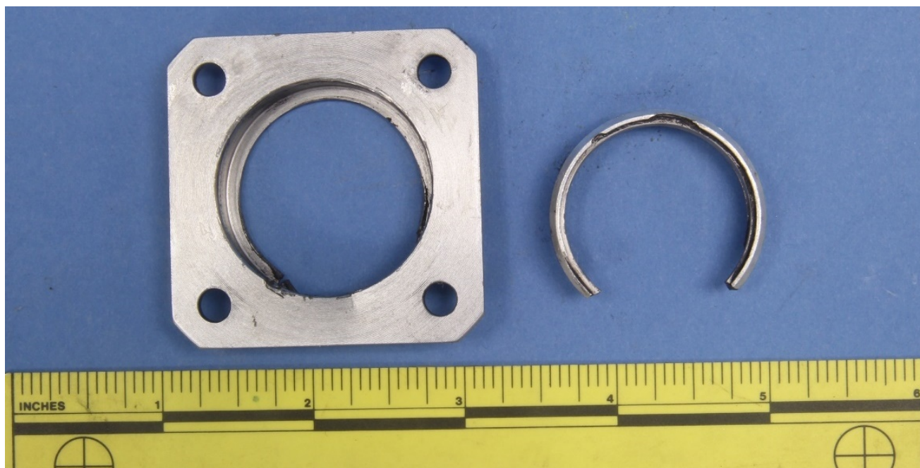
Figure 41 – The bearing liner and race, viewed from the faces opposite those in Figure 40.
