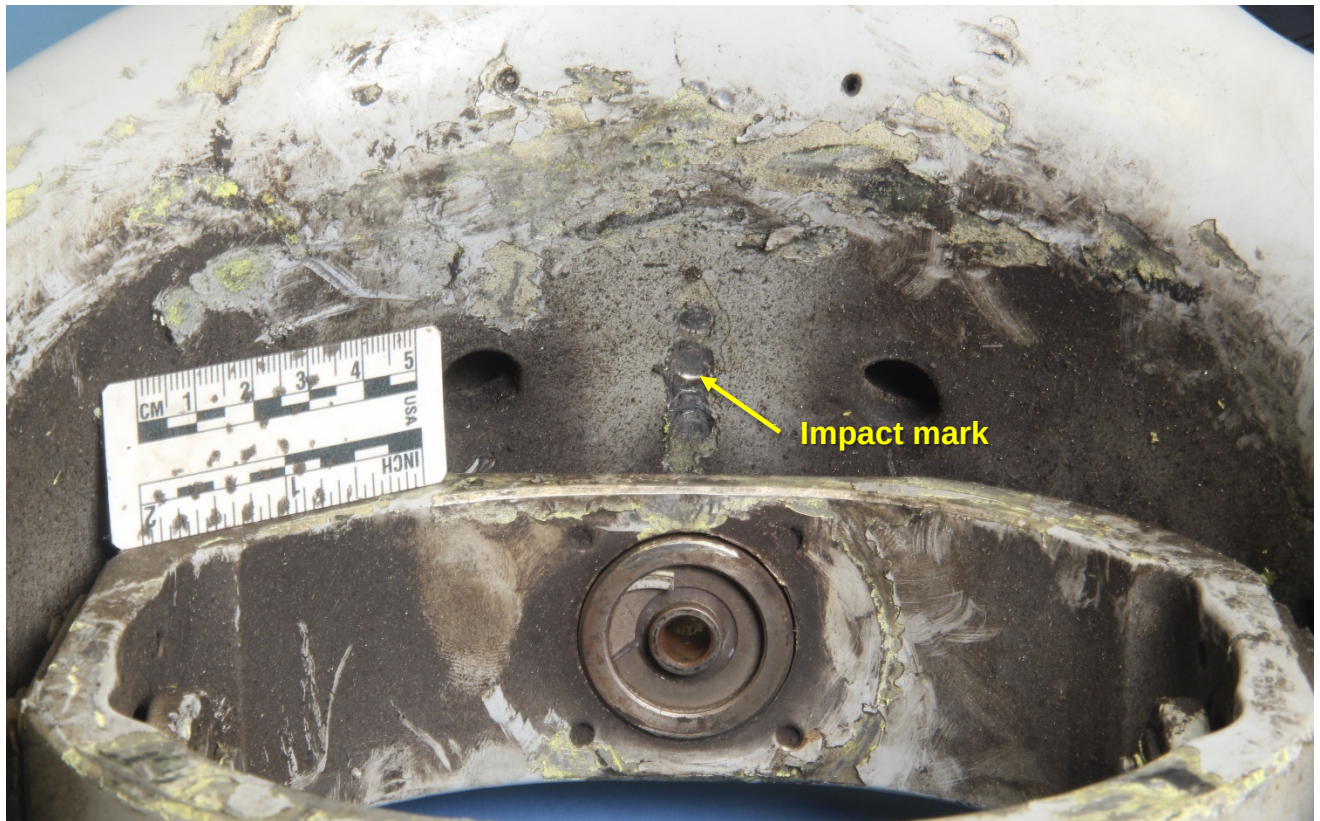
Figure 8 – View of the area in Figure 5, after removal of the bolt and clevises. With the gimble ring pushed down, impact marks were present on the inner surface of the swashplate housing.
