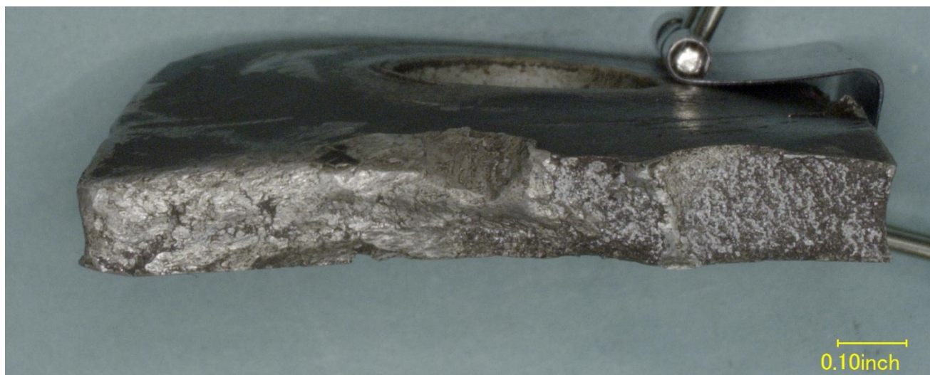
Figure 29 – View of the fracture surface of the fractured support clevis 3.
