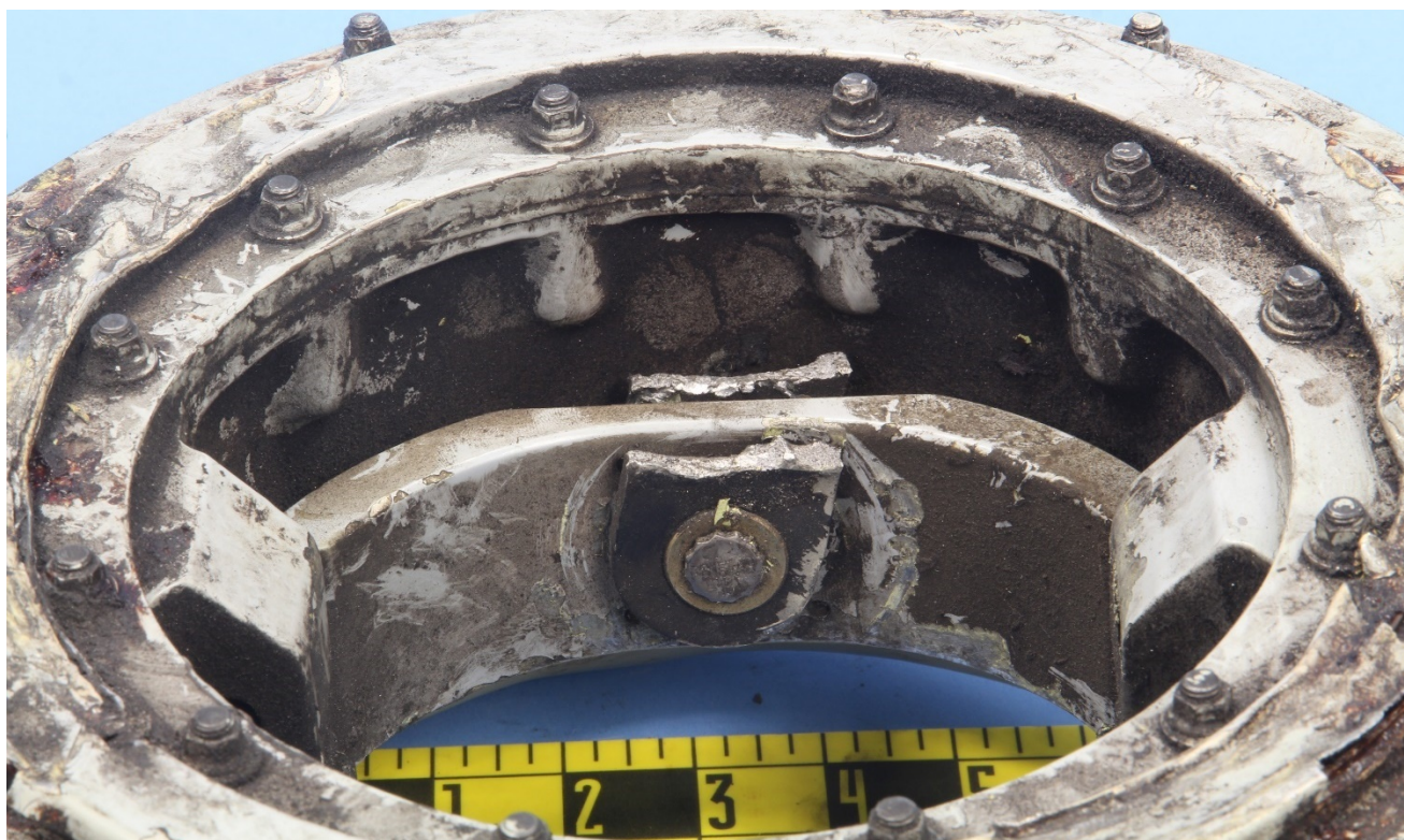
Figure 6 – View of two of the fractured clevises from the collective support, attached to the swashplate assembly through the gimbal ring assembly, as received.
