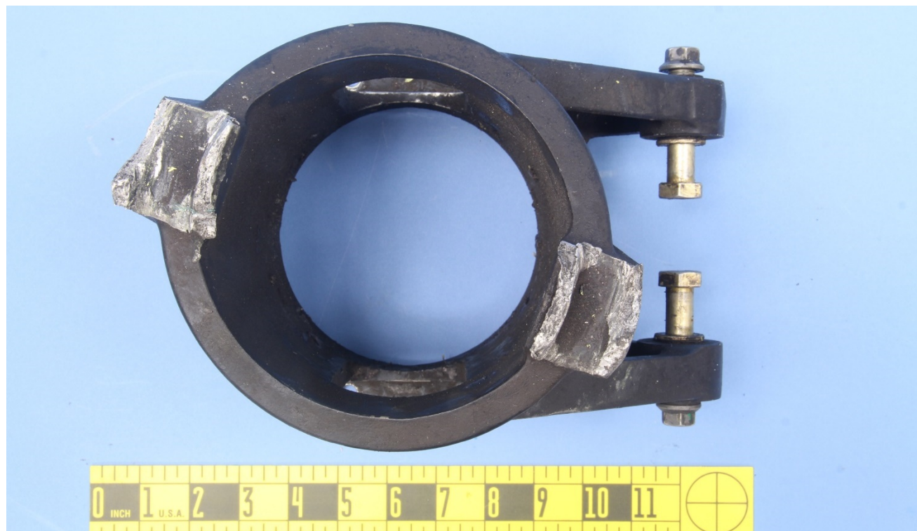
Figure 13 – A topside view of the support, showing the fractured attachment clevises.
