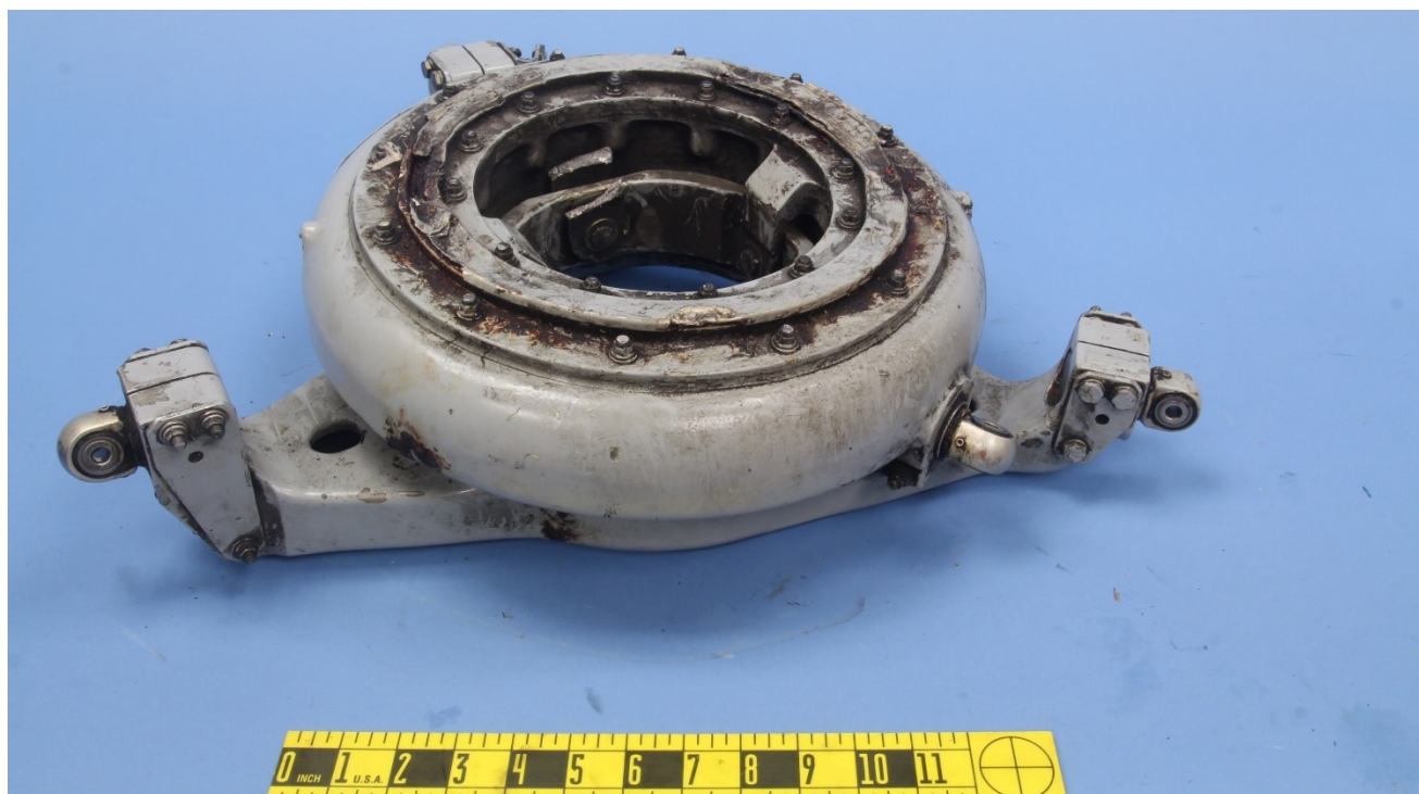
Figure 4 – Angled view of the swashplate assembly, rotated 180° from Figure 3.
