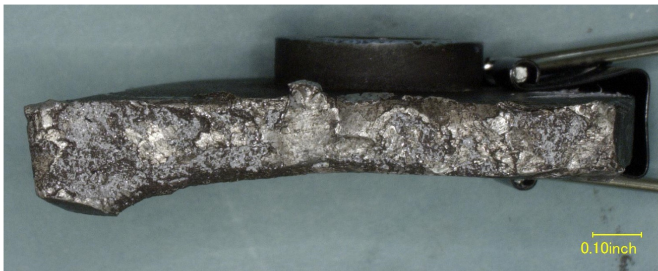
Figure 32 – View of the fracture surface of the fractured support clevis 4.
