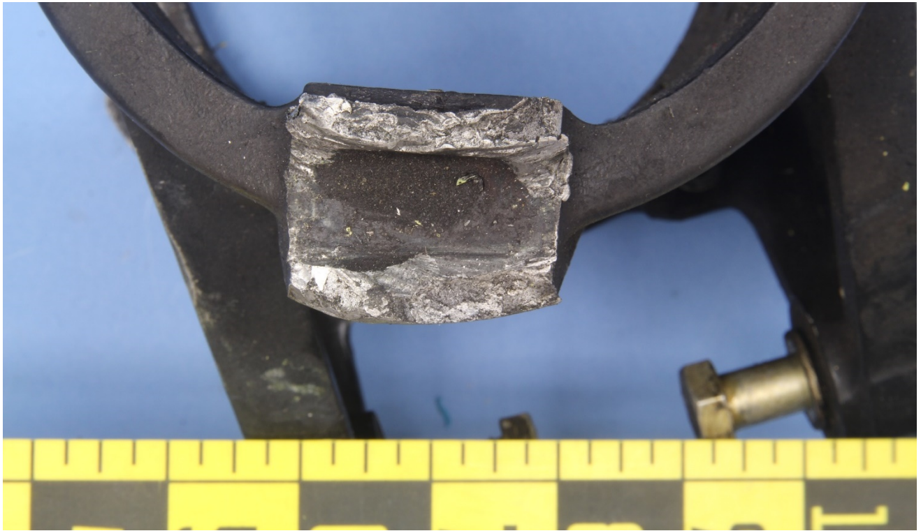
Figure 14 – The forward gimble ring seat of the support, which fractured on the attachment clevis.
