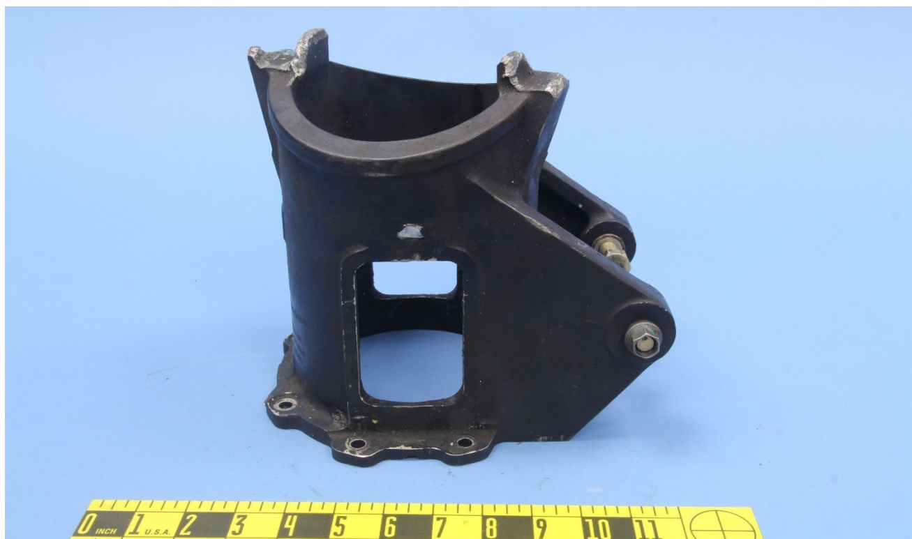
Figure 10 – The collective support, viewed from the right side, showing fractured attachment clevis remnants and an impact mark.
