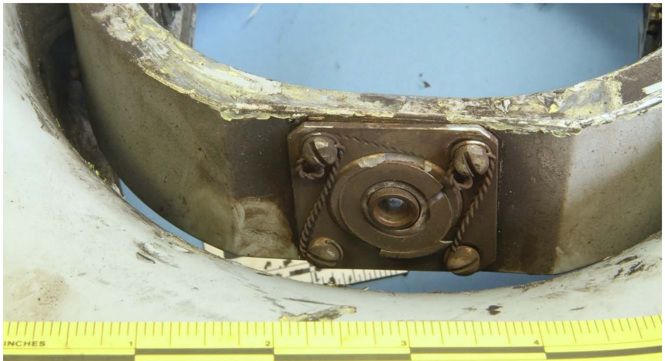
Figure 9 – View of the fractured bearing and liner on the gimble ring opposite Figure 8.
