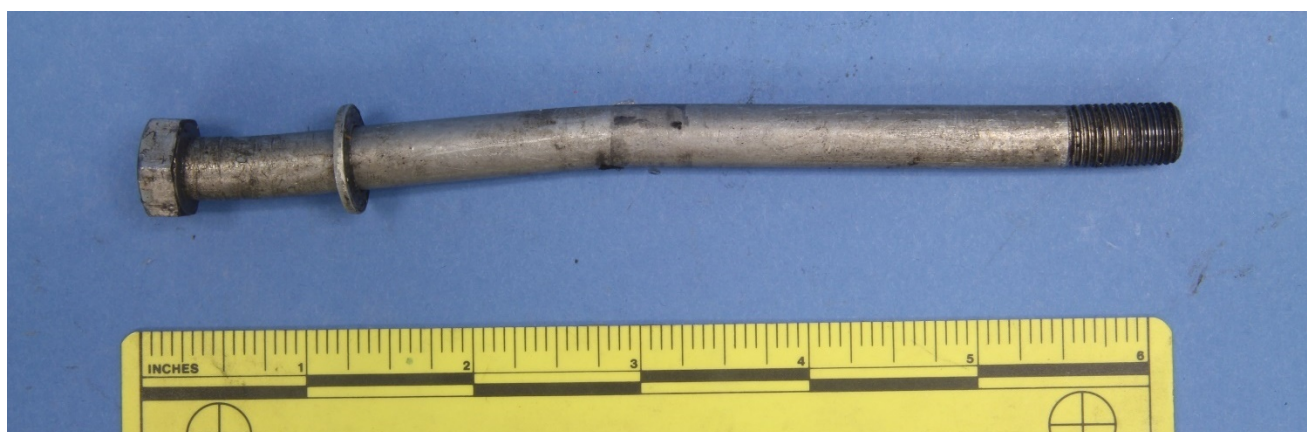
Figure 44 – View of the attachment bolt, after disassembly, showing the bend in the shaft.
