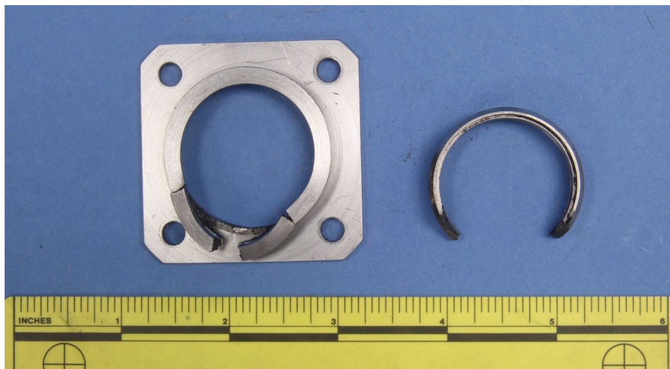
Figure 40 – The fractured bearing liner and bearing race, after cleaning and grease removal.
