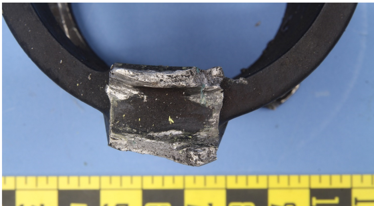
Figure 17 – The aft gimble ring seat of the support, which fractured on the attachment clevis.
