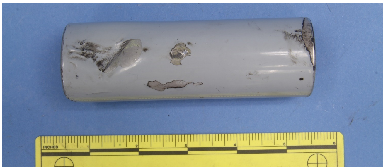
Figure 43 – View of the spacer, after disassembly and cleaning, showing a dent on the side.
