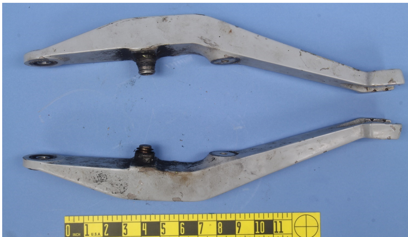
Figure 37 – The collective lever arms, as received.
