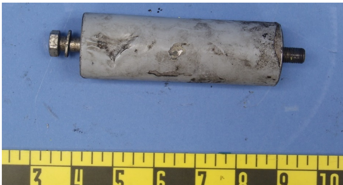
Figure 42 – The attachment bolt and spacer, as received.
