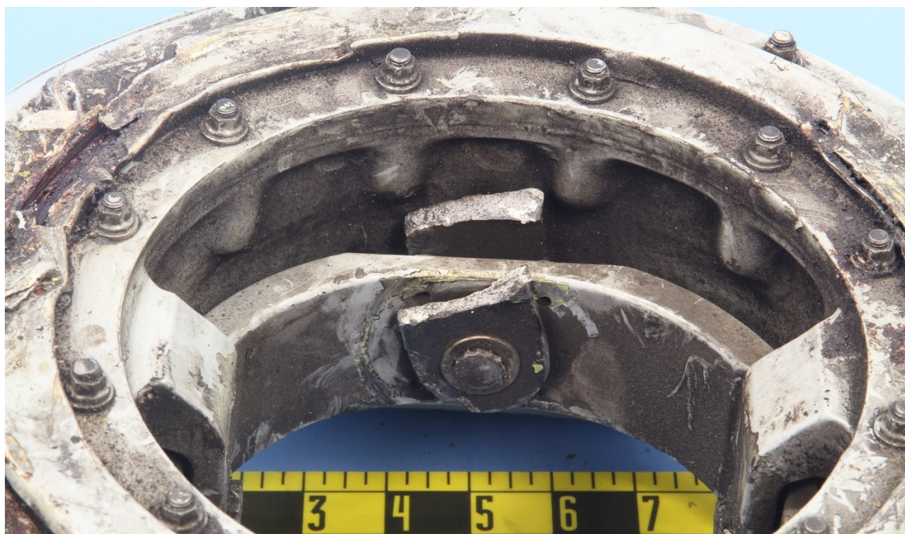
Figure 5 – View of two of the fractured clevises from the collective support, attached to the swashplate assembly through the gimbal ring assembly, as received.
