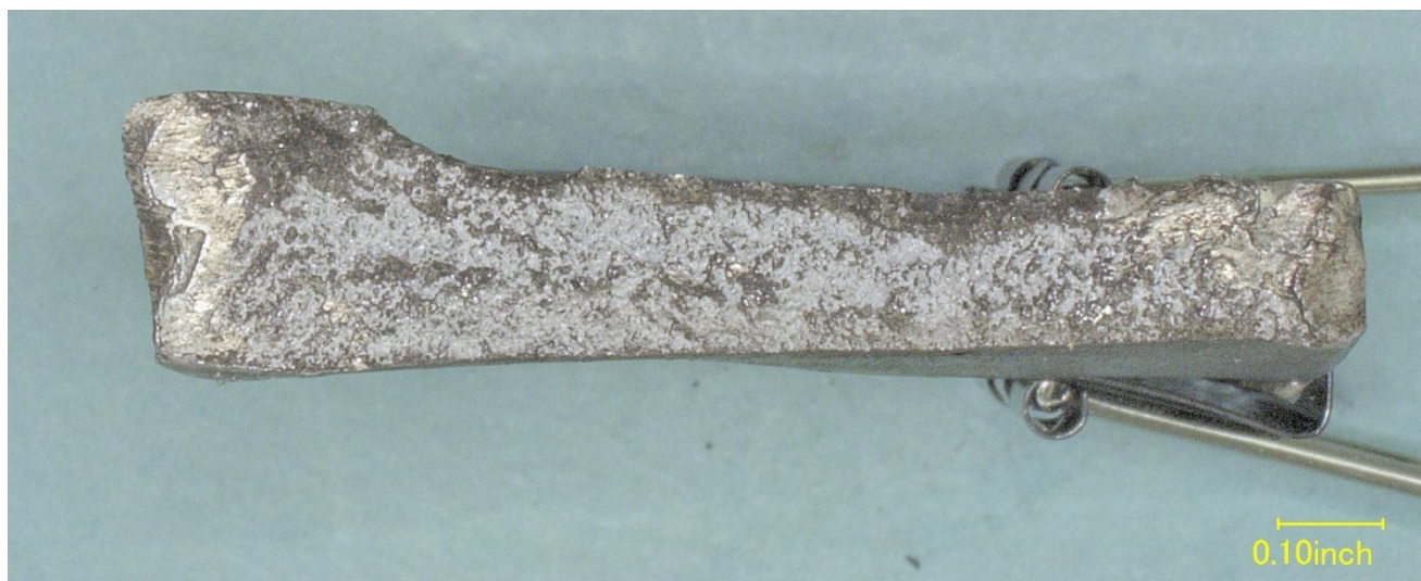
Figure 26 – View of the fracture surface of the fractured support clevis 2.
