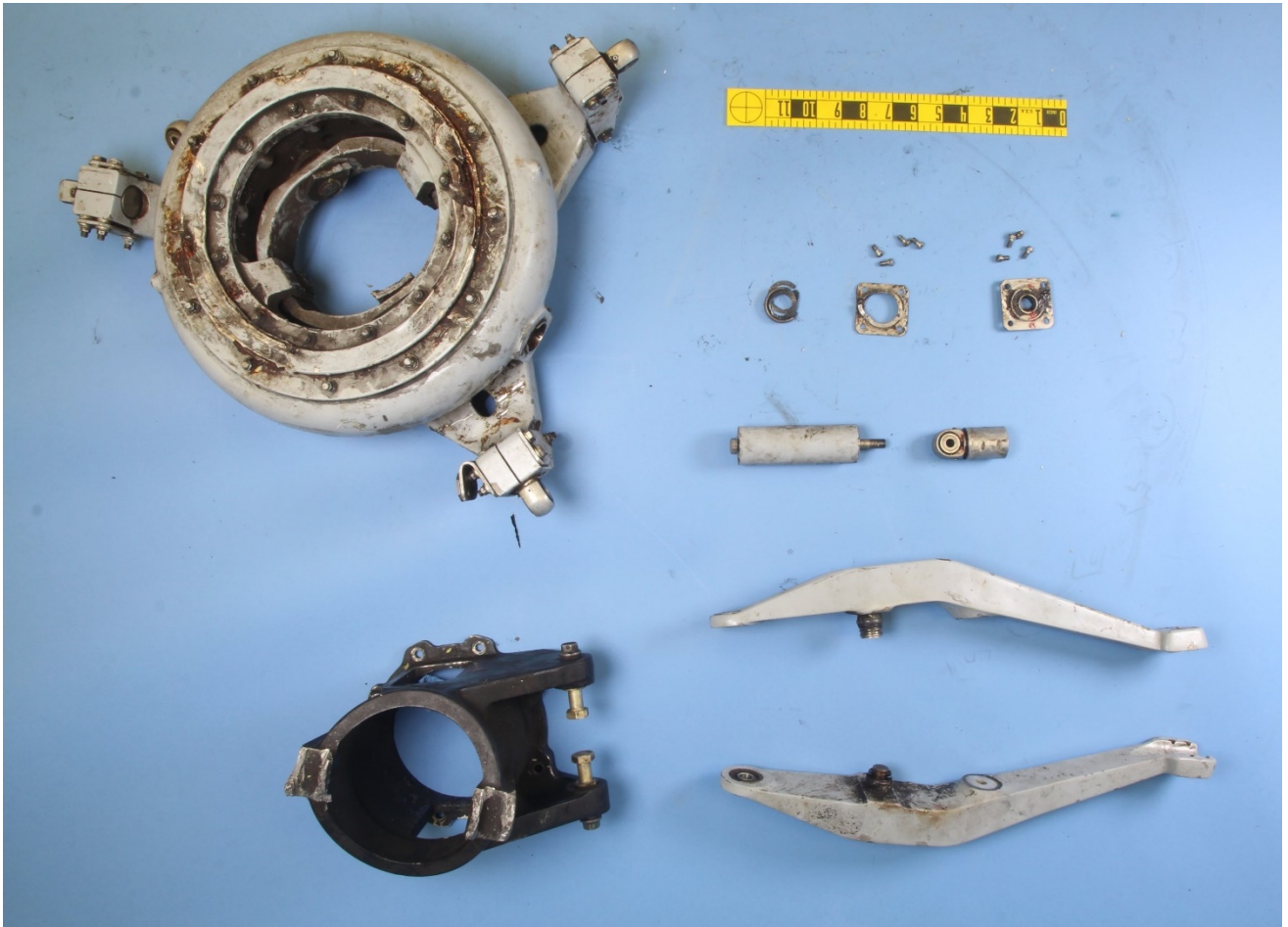
Figure 1 – The components from the swashplate and sleeve assembly, as received.
