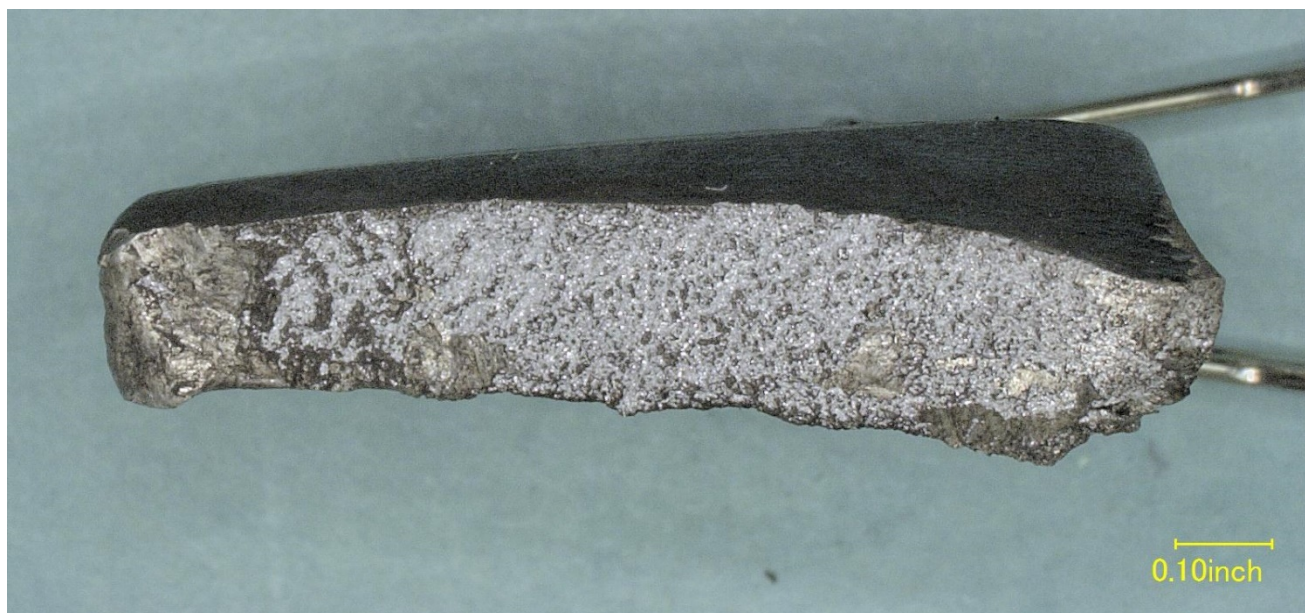
Figure 21 – View of the fracture surface of the fractured support clevis 1.
