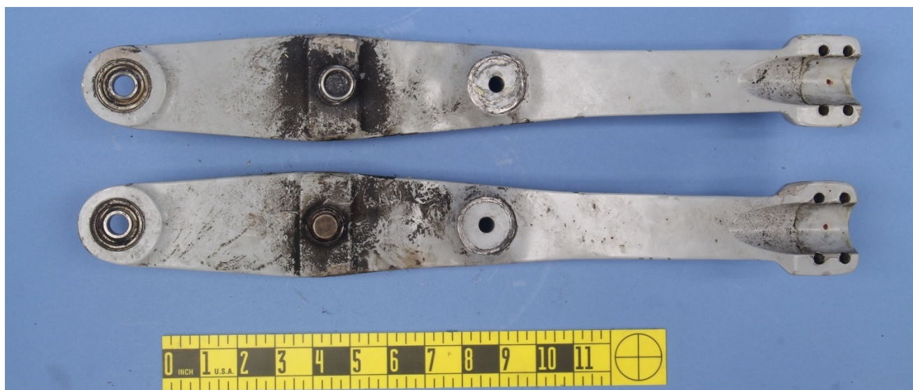
Figure 38 – The faying surfaces of the collective lever arms, as received.
