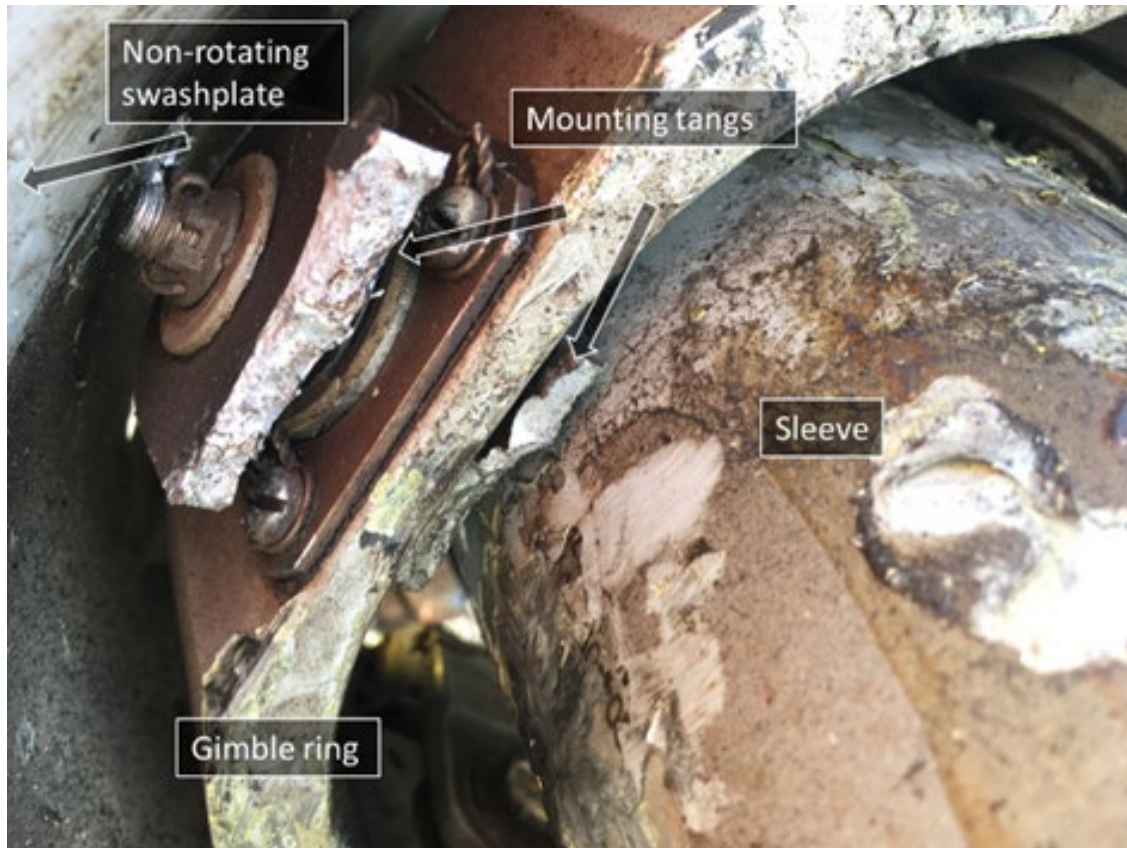
Figure 7. Image showing one side of the gimble ring and the attached swashplate support tangs. The contact marks on the collective sleeve are in view. Photo FAA
