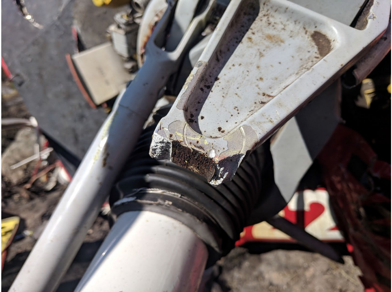
Figure 6. Image showing swashplate drive link A and the area of the missing tangs. Photo US Forest Service.
