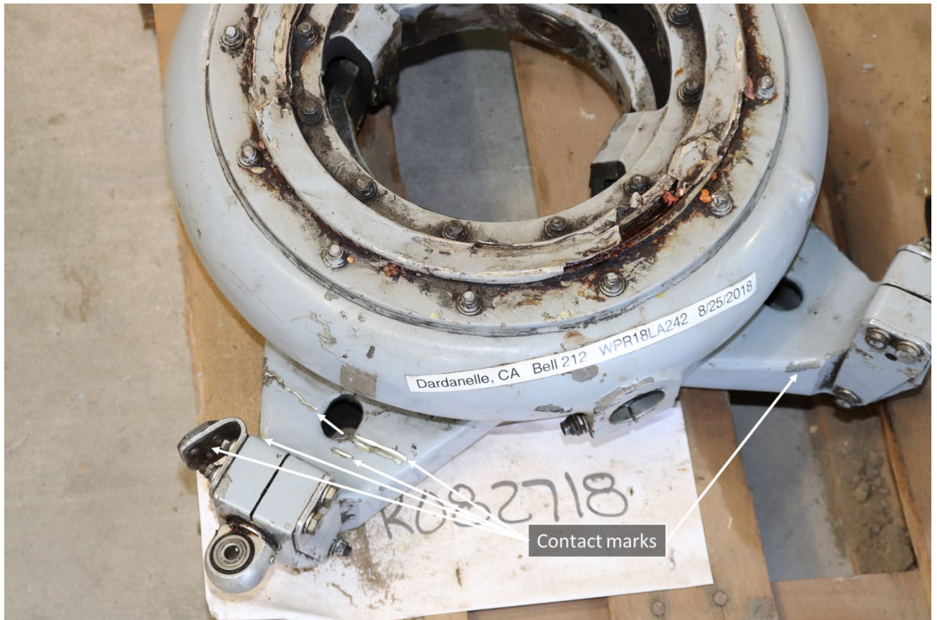
Figure 14. Image showing contact marks made to the non-rotating swashplate arms.
