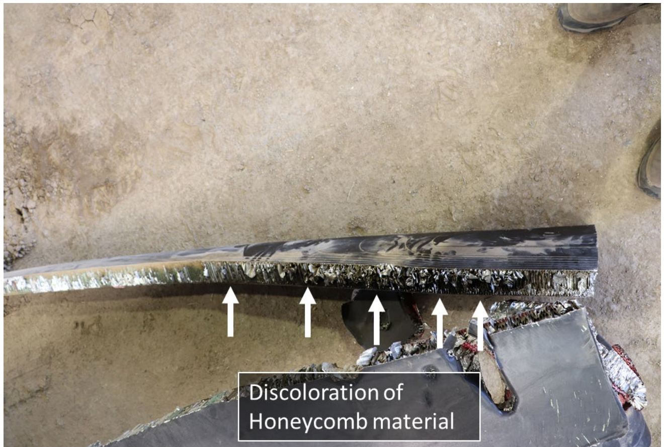
Figure 20. Image showing a darkened area of the aluminum honeycomb from blade A.
