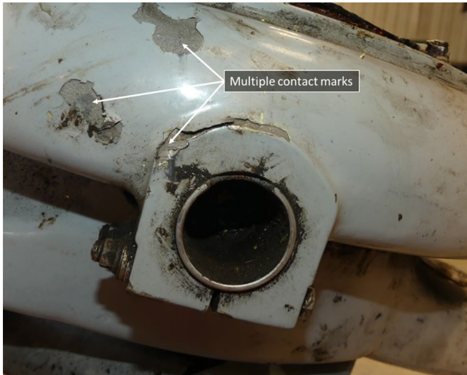
Figure 15. Image showing contact marks made to the rotating swashplate. The trunnion bearing A outer sleeve is visible.
