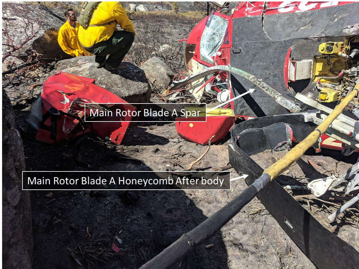
Figure 17. Image showing how Blade A separated into two long halves, a spar half, and a honeycomb after body half. Photo US Forest Service.
