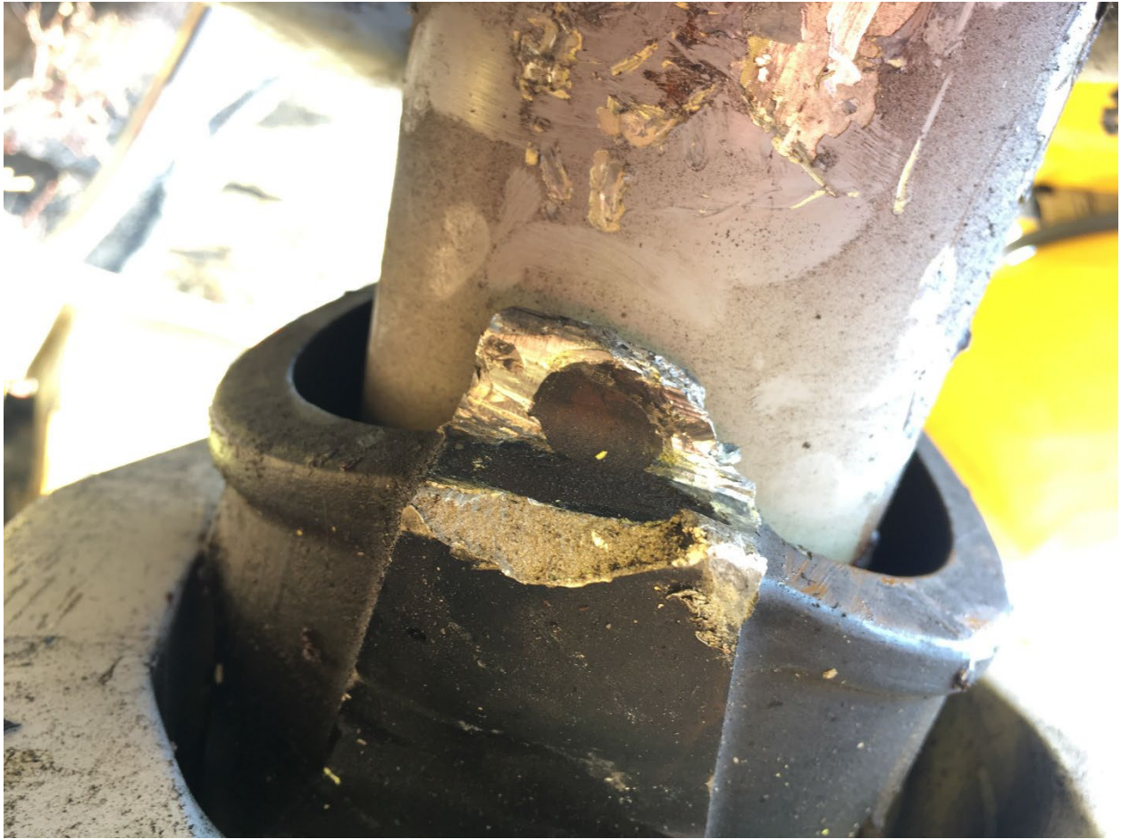
Figure 9. One side of the swashplate support, showing the area of the missing tangs and smearing of the fractured metal. The contact marks to the collective sleeve are in view at the top. Photo FAA.
