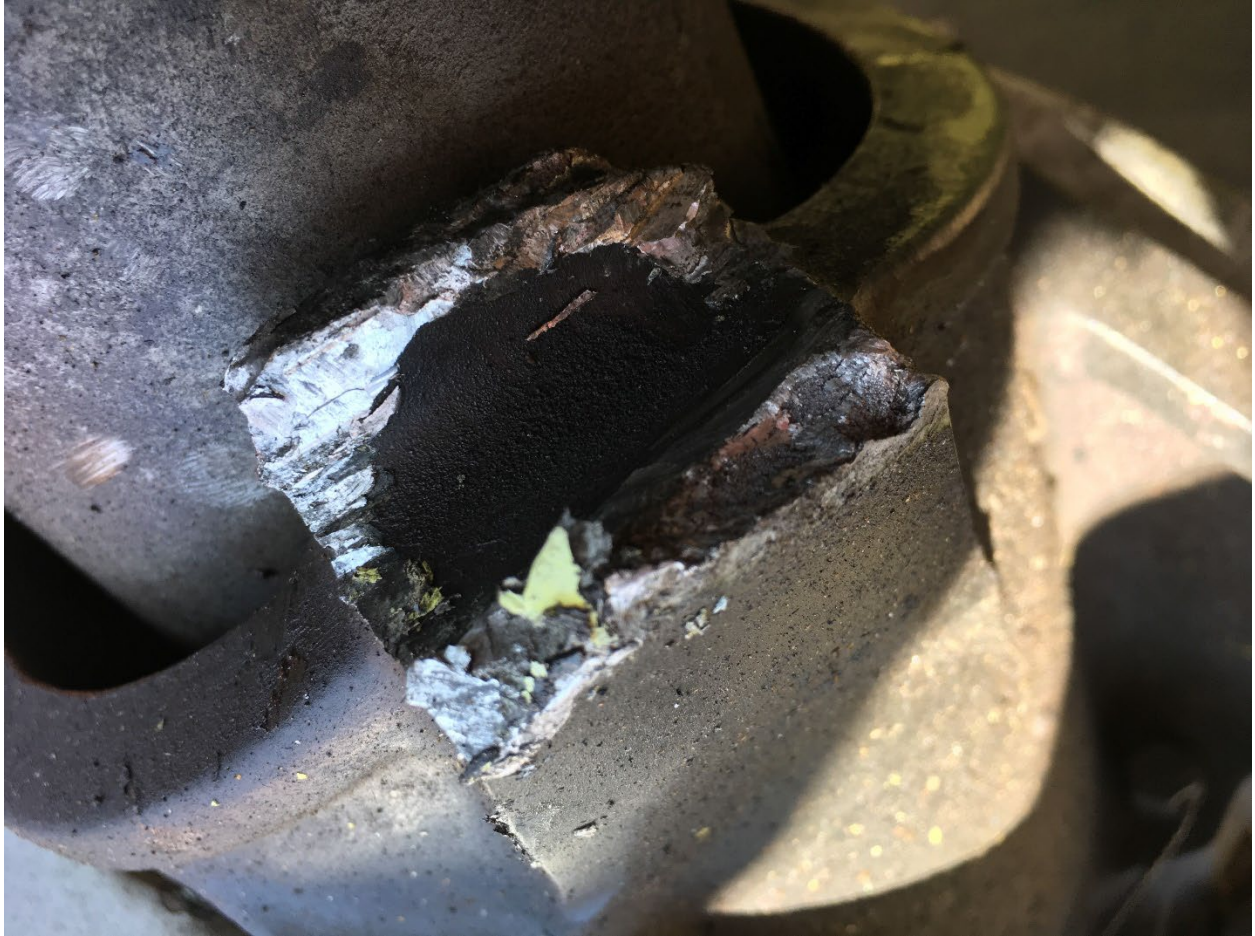
Figure 10. The other side of the swashplate support showing the area of the missing tangs and smearing of the fractured metal. Photo FAA.
