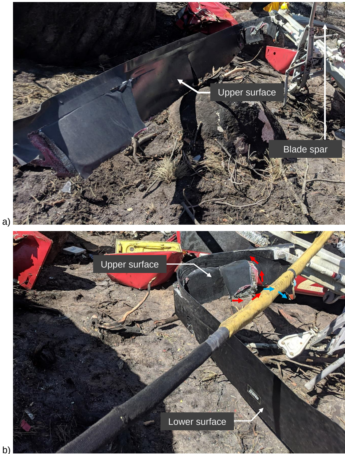
Figure 6: Images of the main rotor blade afterbody at the crash site: a) image showing the afterbody upper surface and b) image showing the root end of the blade with the upper surface visible in the background and lower surface visible in the foreground. The afterbody did not appear to exhibit the same upward bending as the spar.
