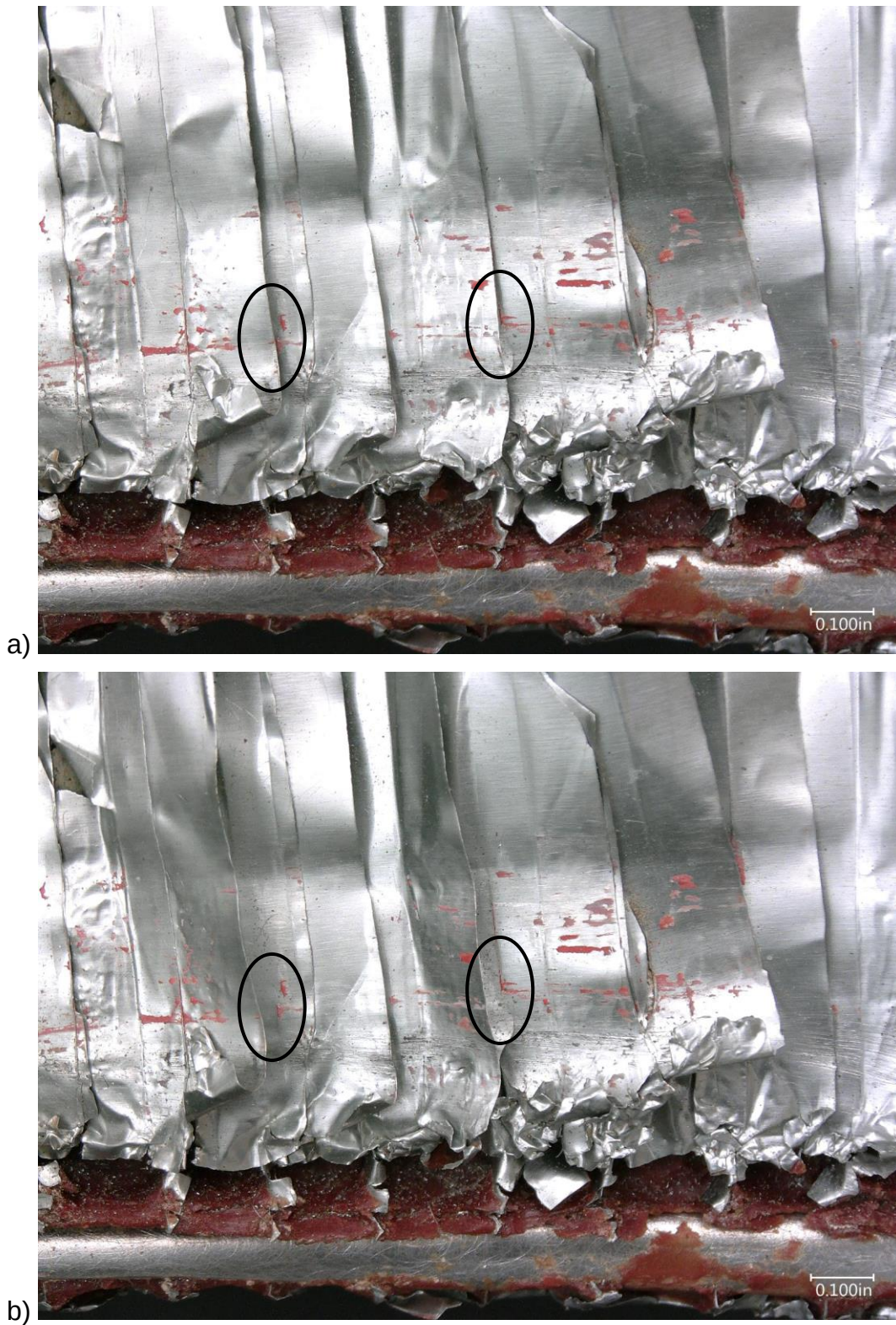
Figure 10: Images of the flattened honeycomb core : a) image showing smeared red adhesive on the cell walls and b) two of the cell wall lifted showing no adhesive under the folds.
