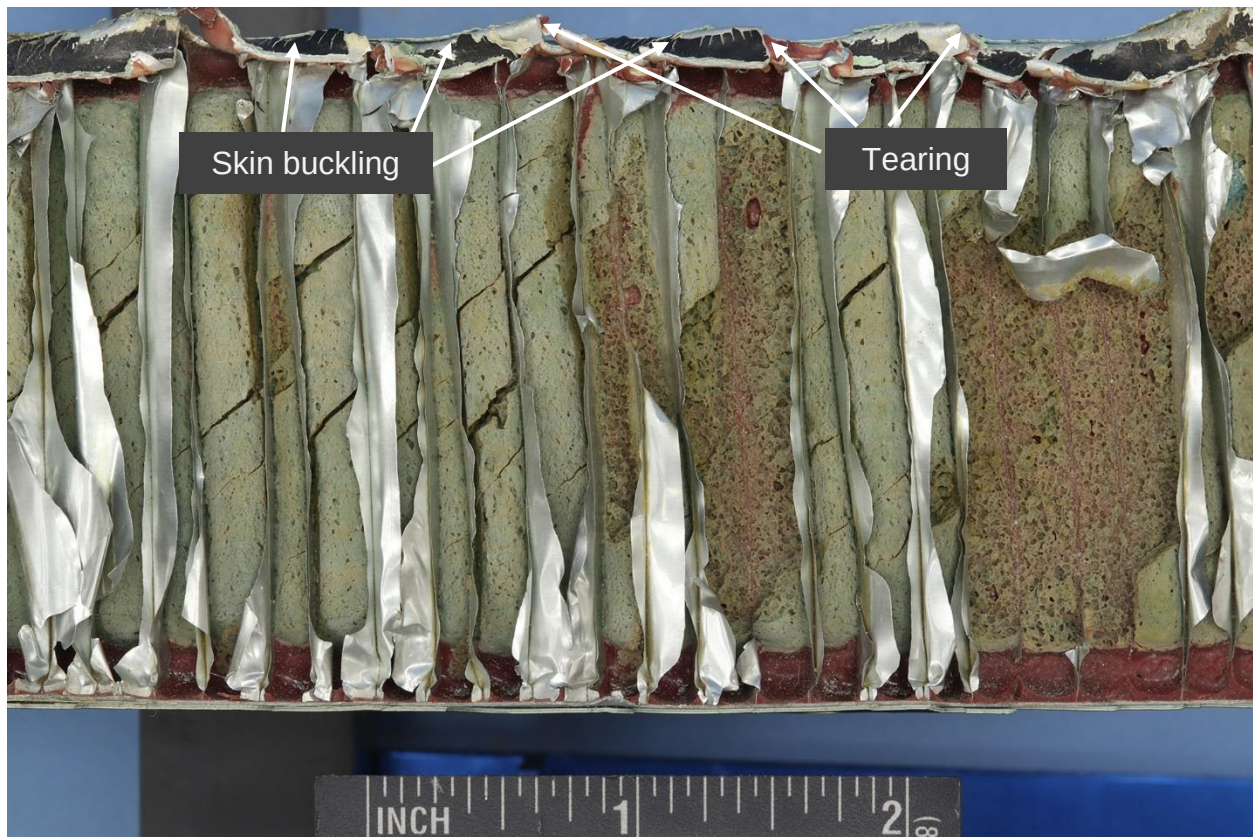
Figure 5: Image of the main rotor blade spar aft face shown the construction of the spar to afterbody transition as well as skin bending/buckling and tearing features along the upper skin. See figure 2b for location information.
