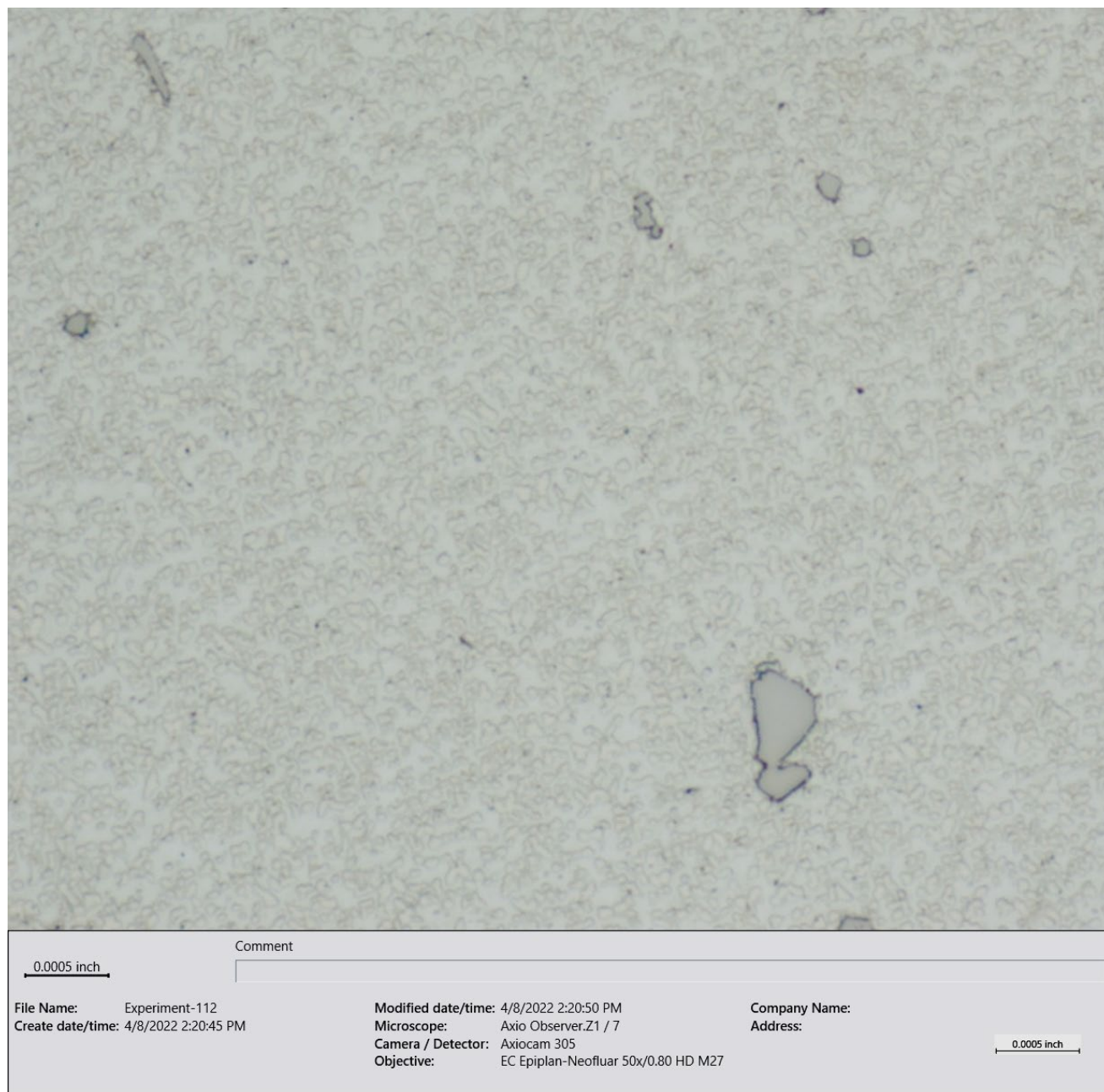
Figure 22 – BF optical micrograph showing a typical view of the dovetail microstructure in Blade D, showing primary carbides and the small, semi-cuboidal \gamma' phases (~1000X, etched Kallings Reagent #2).
