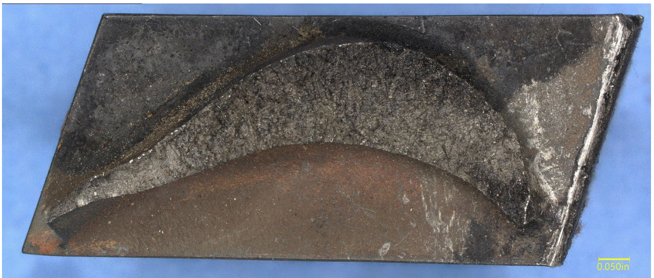
Figure 6 – The fracture surface of Blade 7.
