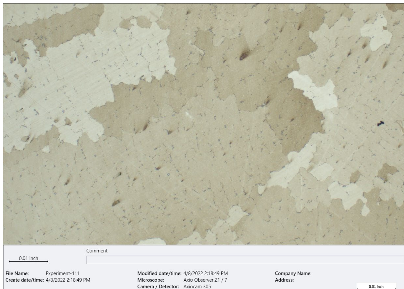
Figure 20 – Bright-field (BF) optical micrograph of a typical cross section of the Blade D dovetail (~50X, etched Kallings Reagent #2).
