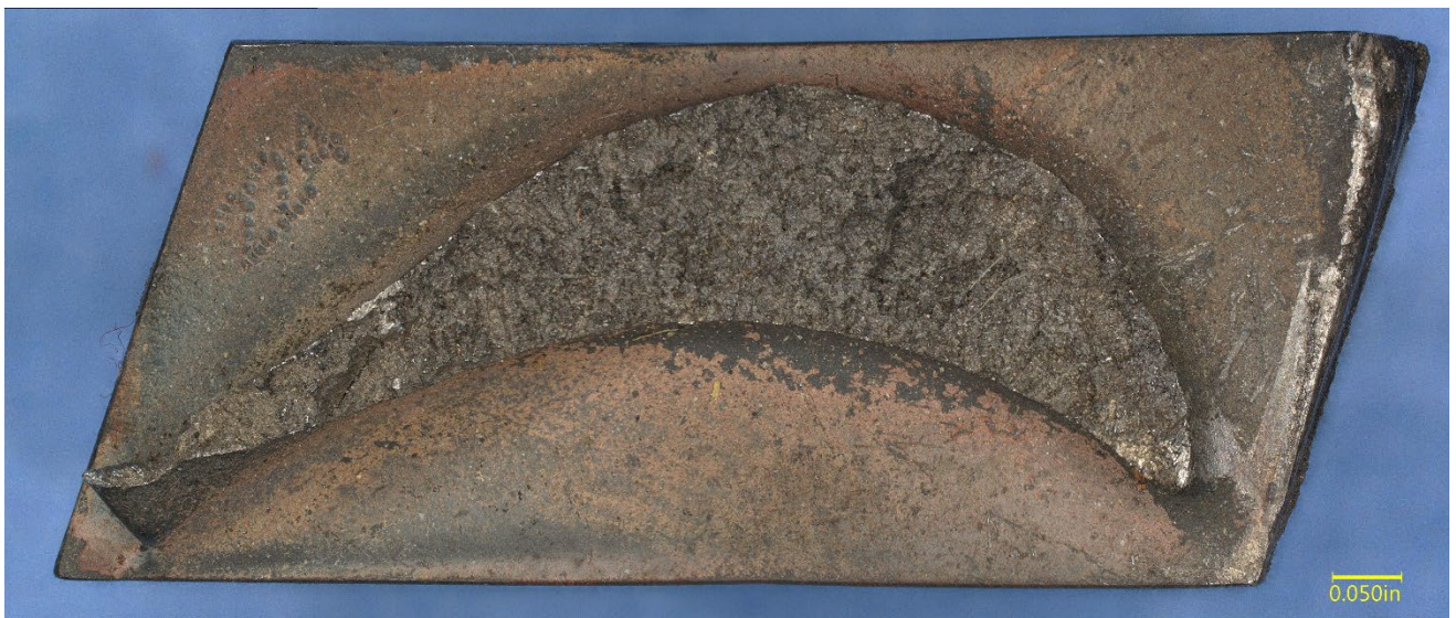
Figure 10 – The fracture surface of Blade 10.
