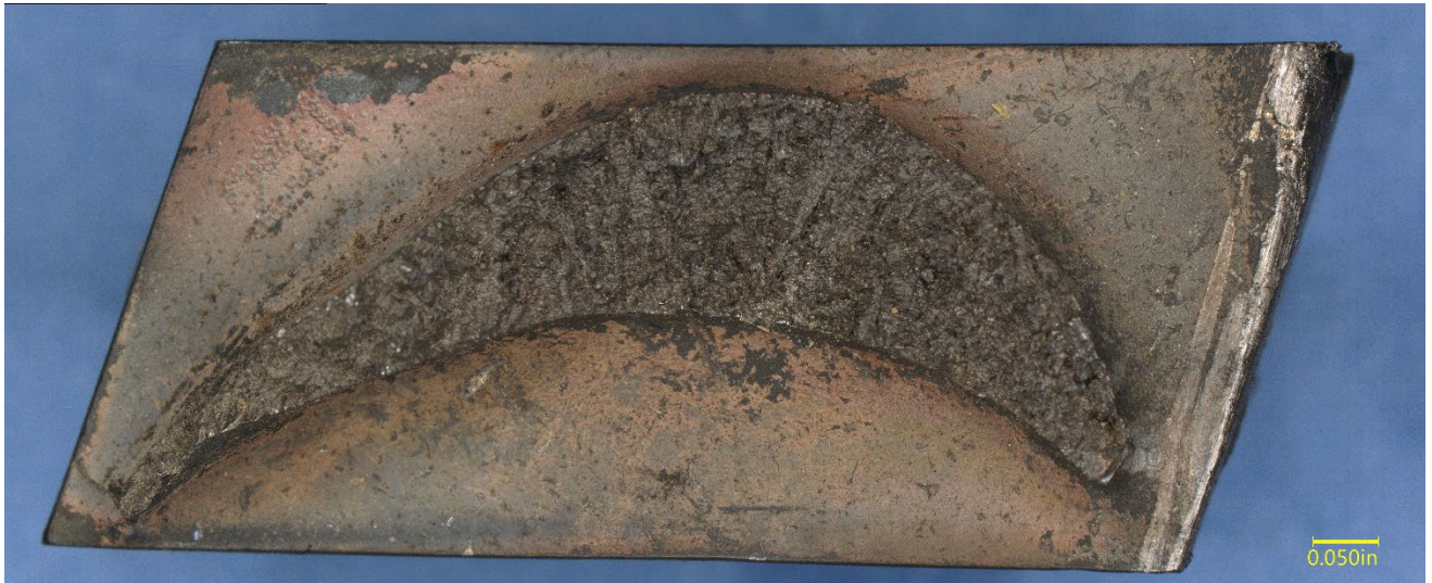
Figure 3 – The fracture surface of Blade 8.
