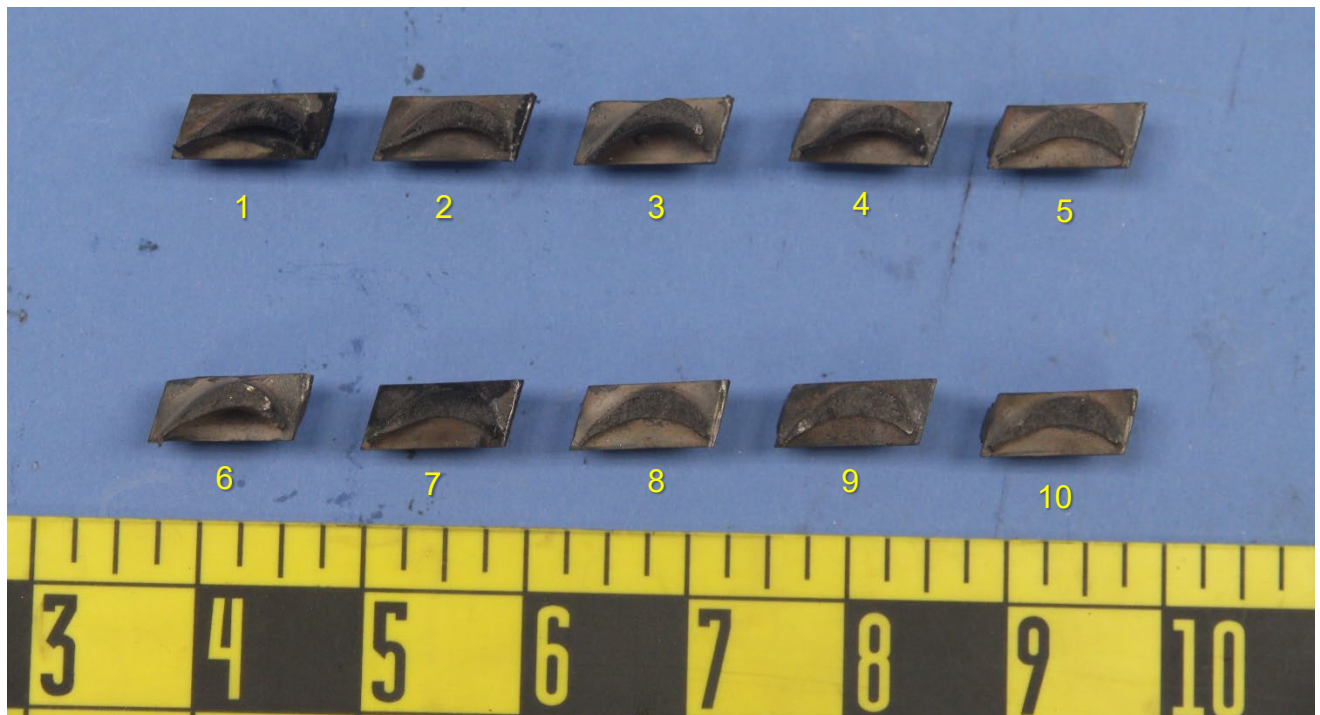
Figure 2 – Views of the fracture surfaces of the shortest blade remnants, on the left in Figure 1.
