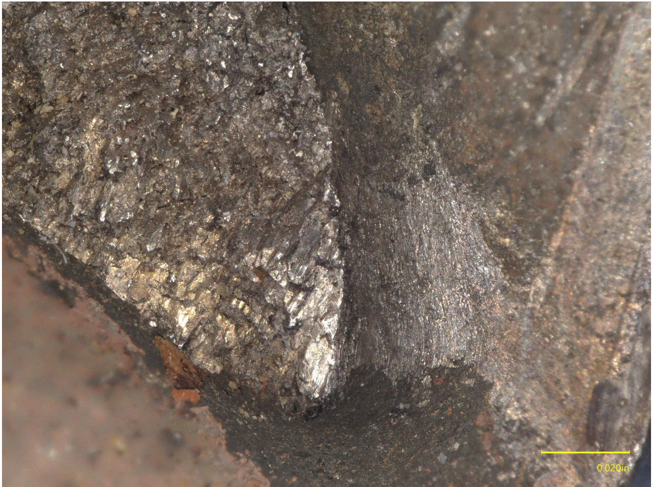
Figure 11 – Closer view of the leading edge of the Blade 10 fracture surface.
