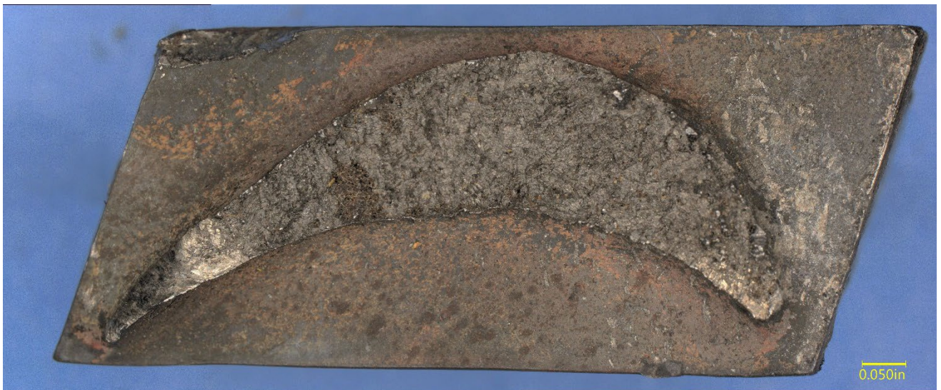
Figure 8 – The fracture surface of Blade 9.
