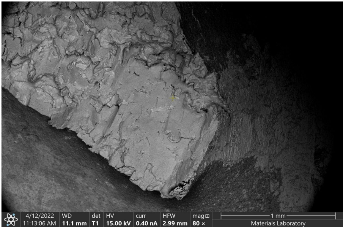
Figure 12 – Backscattered electron (BE) micrograph of the leading edge of the Blade 7 fracture surface.
