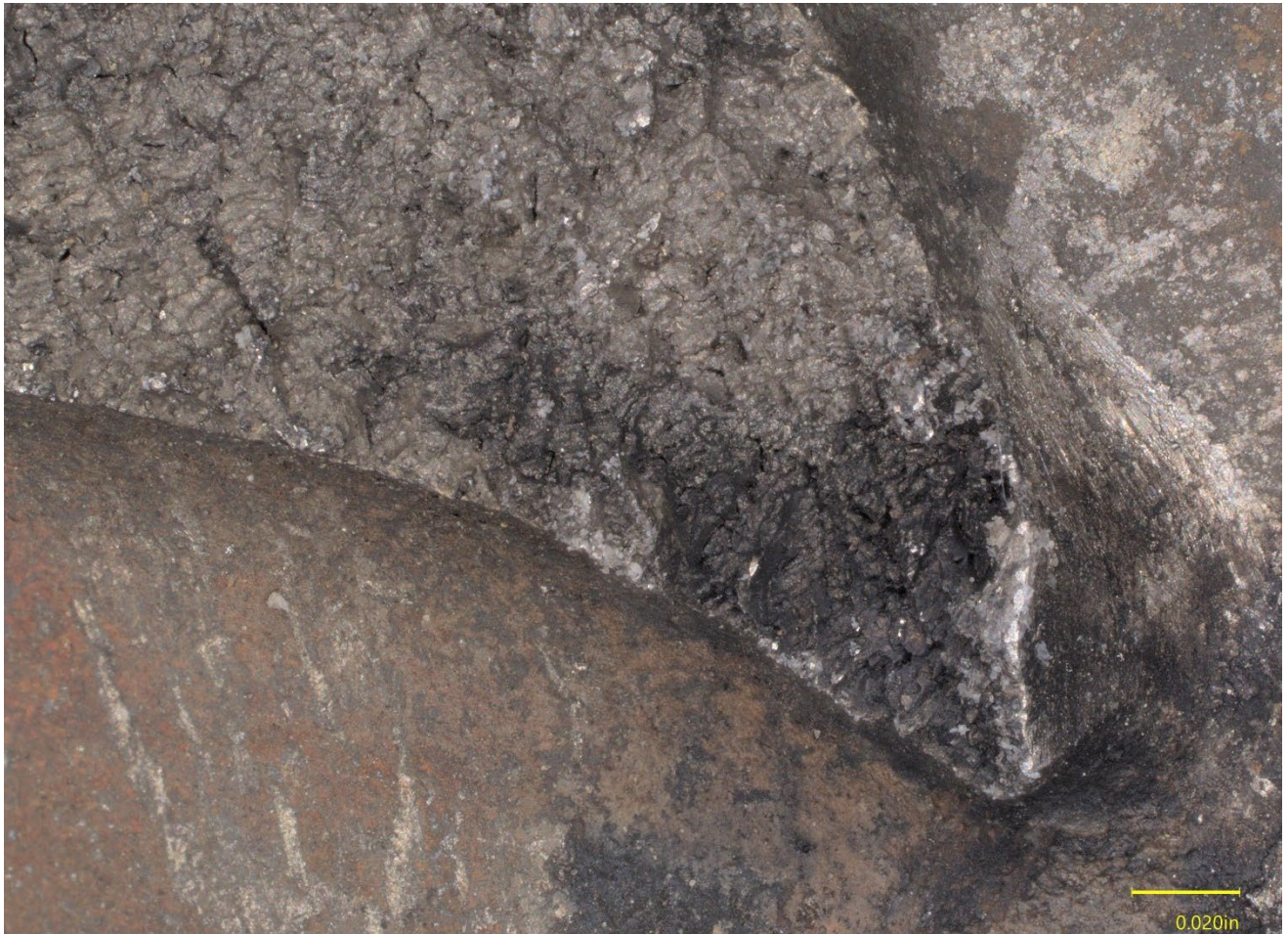
Figure 7 – Closer view of the leading edge of the Blade 7 fracture surface.
