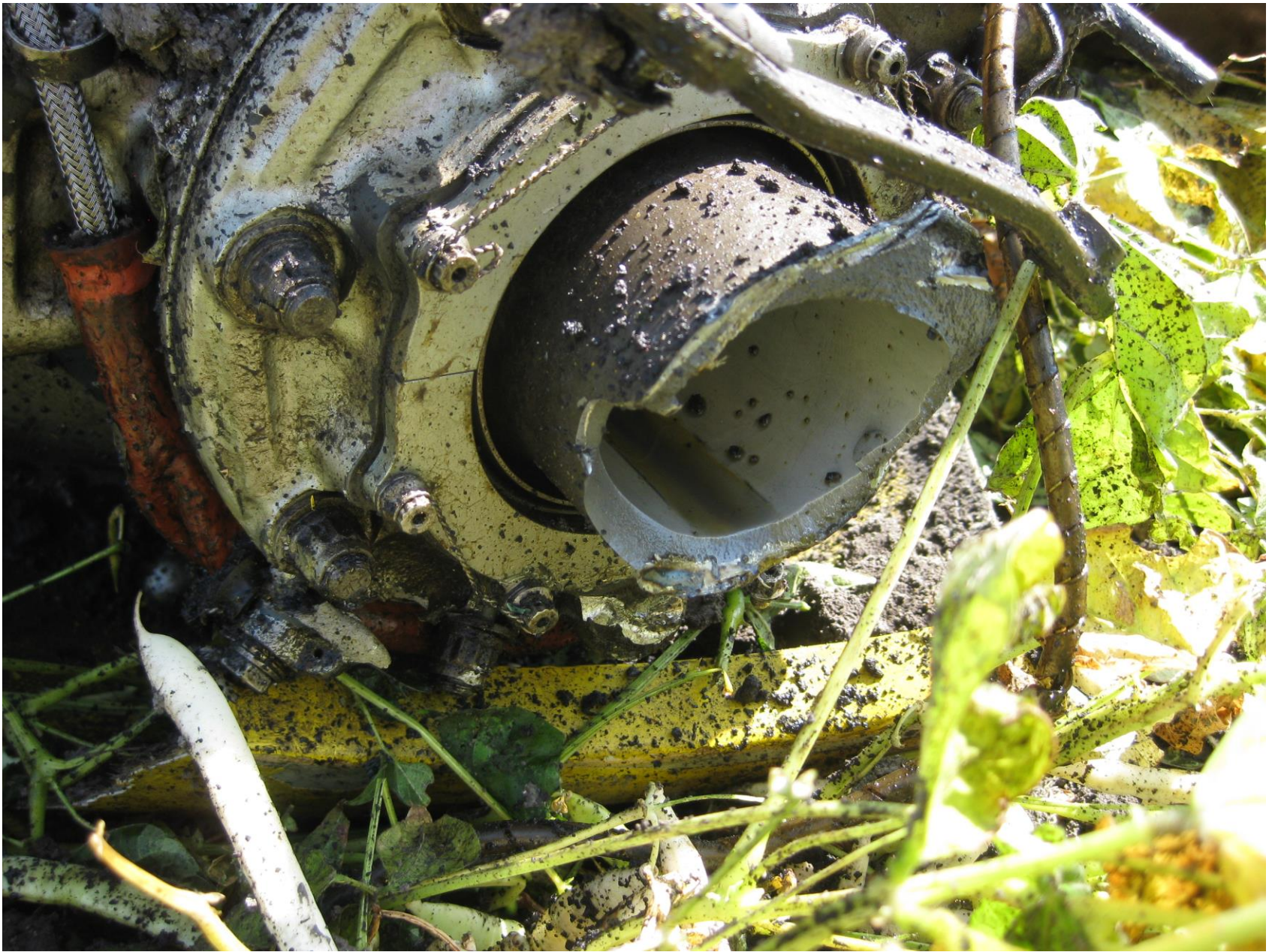
Photo 14 - Accident site, drive shaft separation. (Courtesy of first responders)
