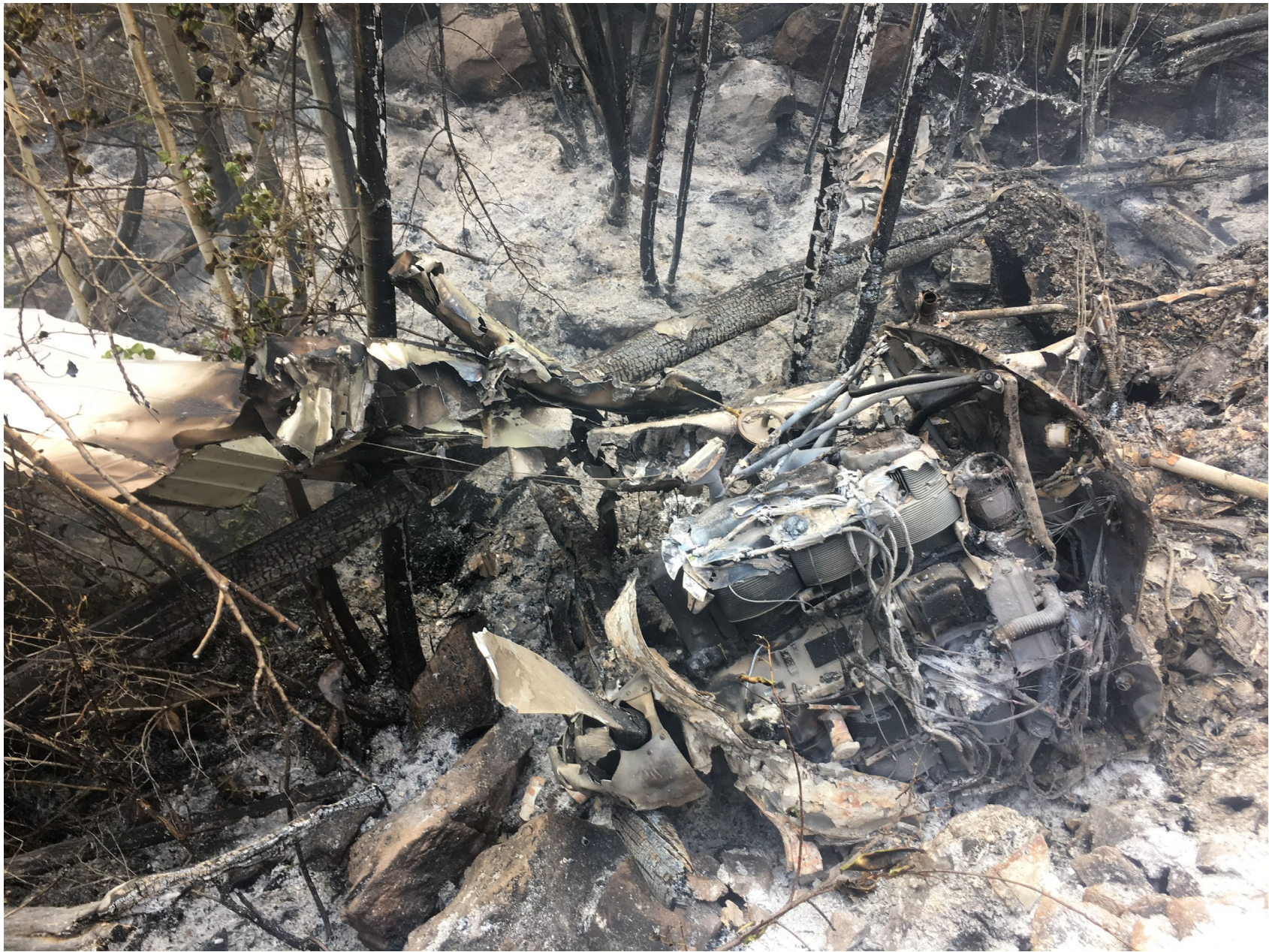
Photo 4 – onsite view of engine, firewall and propeller (courtesy of Salmon-Challis Forest Service)
