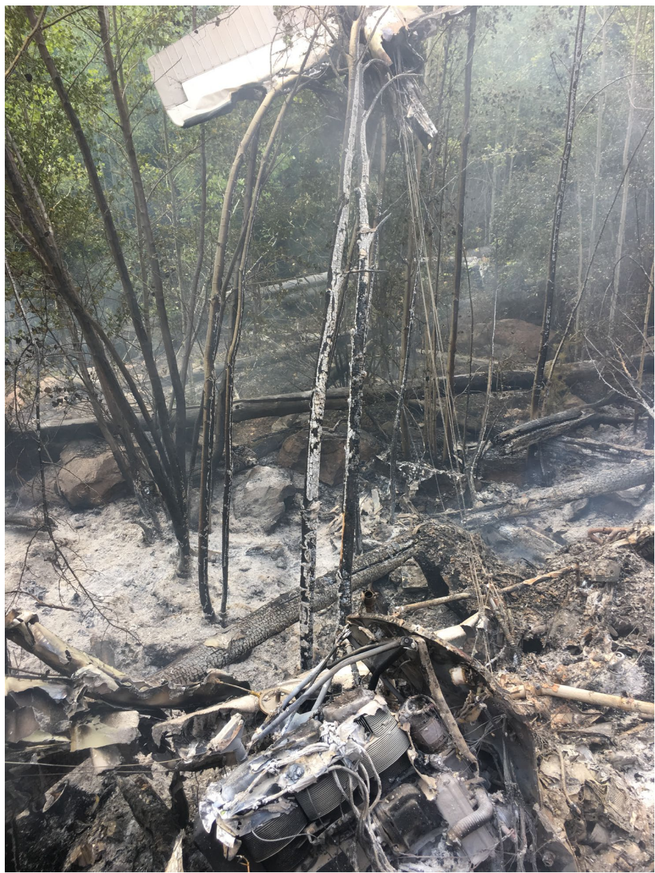
Photo 5 – onsite view of engine and empennage wedged in tree (courtesy of Salmon-Challis Forest Service)
