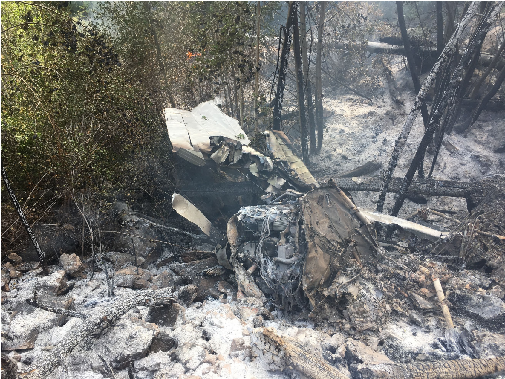
Photo 3 – onsite view of wreckage, including cabin/cockpit area, firewall, engine, propeller, bottom of right wing and aileron (courtesy of Salmon-Challis Forest Service)
