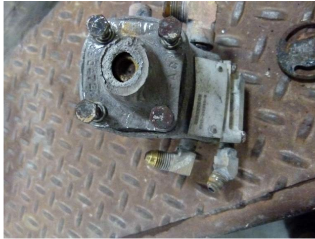
Figure 7 - photo of fuel pump
