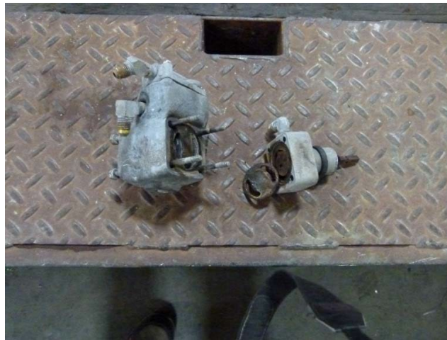
Figure 8 - photo of fuel pump
