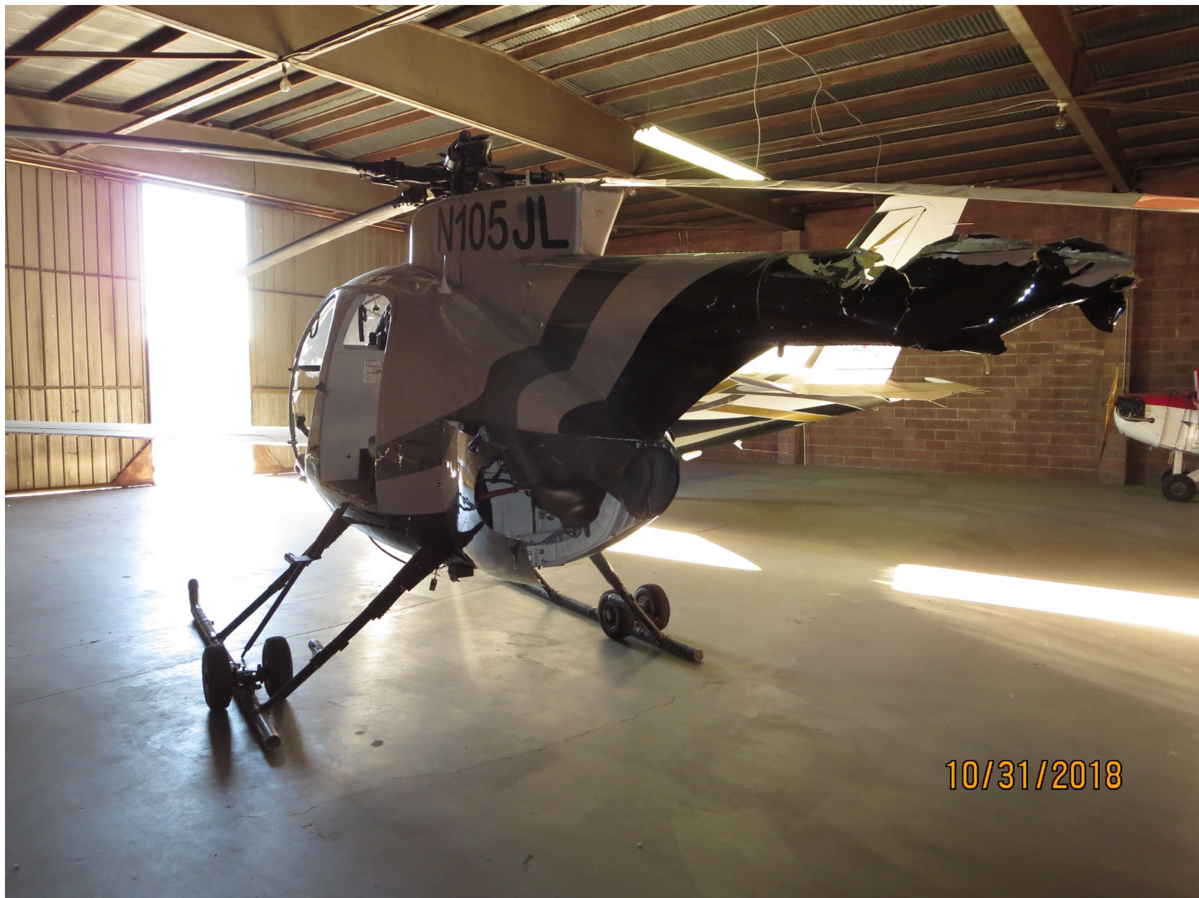
Photo 2 – view of damage to left rear of helicopter
