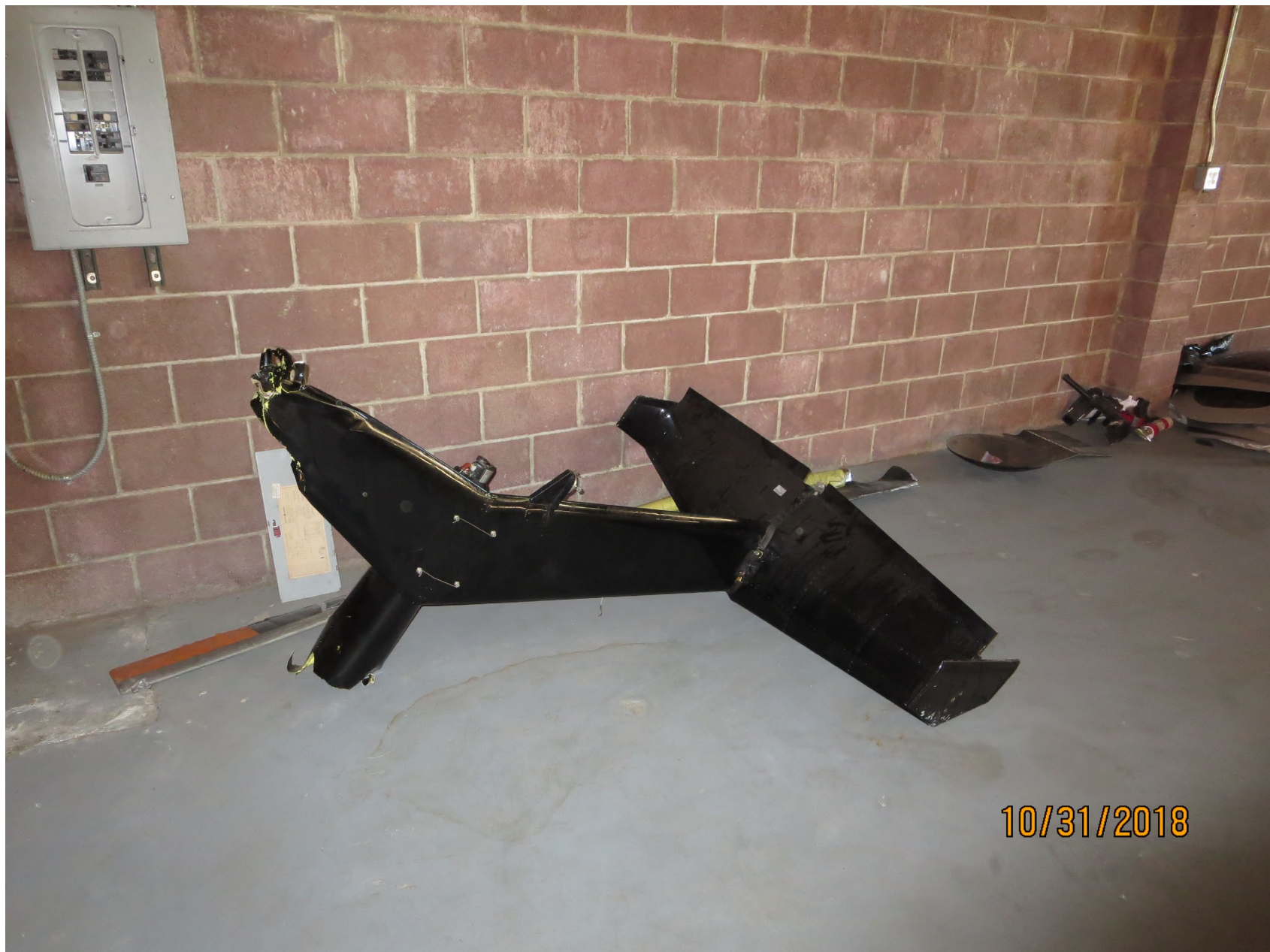
Photo 3 – view of damage to separated tail section of helicopter
