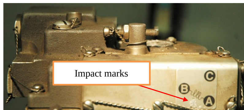
Figure 10 CSU impact marks
