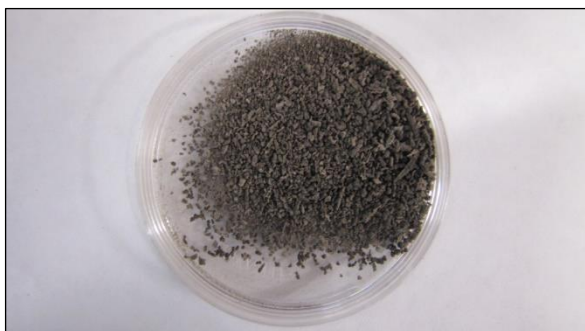
Picture 3: Debris from combustion chamber inner liner (S#2)
