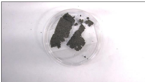
Picture 5: Debris from PT1 vane ring
