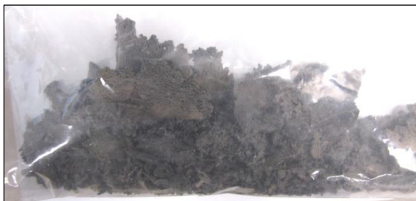
Picture 1: Debris from combustion chamber outer liner (S#1)
