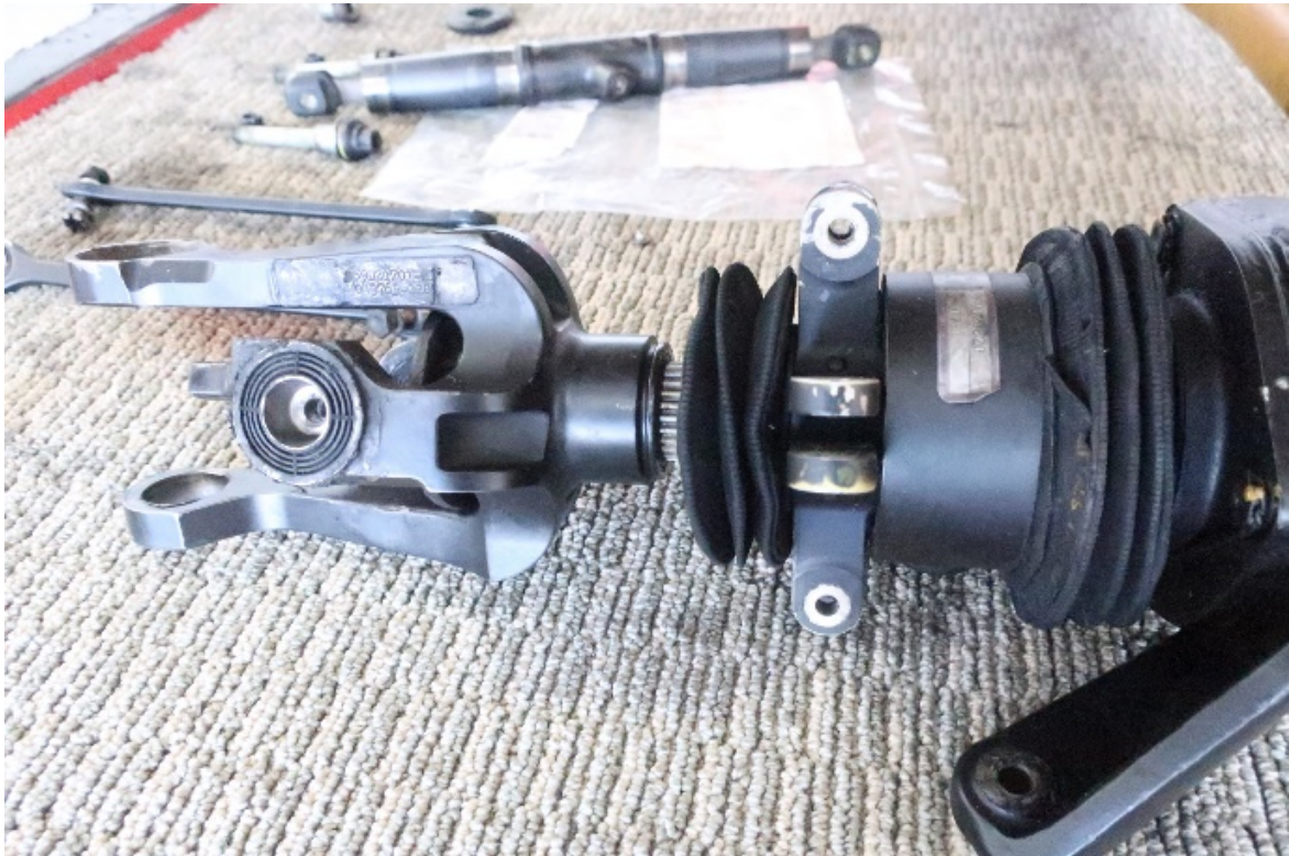
Figure 6 - Tail Rotor Fork
