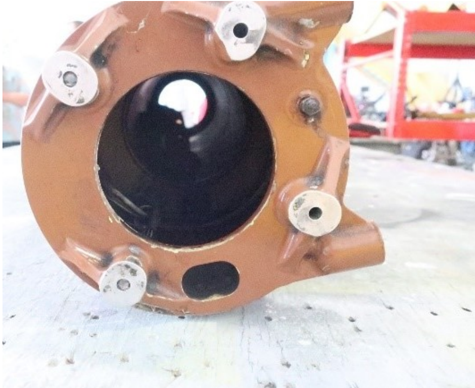
Figure 3 - Tailboom Tail Rotor Gearbox Mounting Fixture
