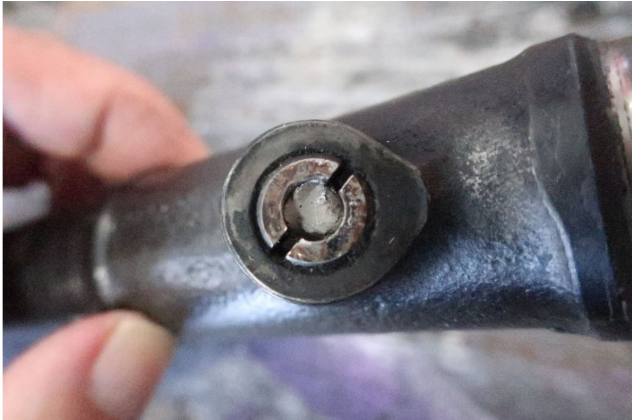
Figure 8 - Outer Tail Rotor Hinge Bolt (exhibiting fracture face)
