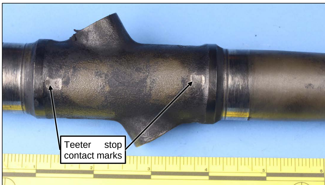
Figure 16. Inboard face of the inboard tail rotor hub showing contact marks corresponding to contact with the teeter stop.
