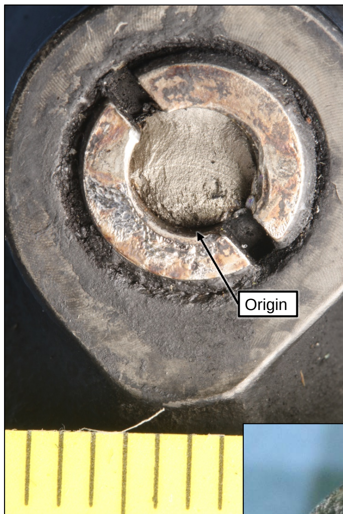
Figure 18. Outboard teeter bolt fracture surface before removal from the hub.
