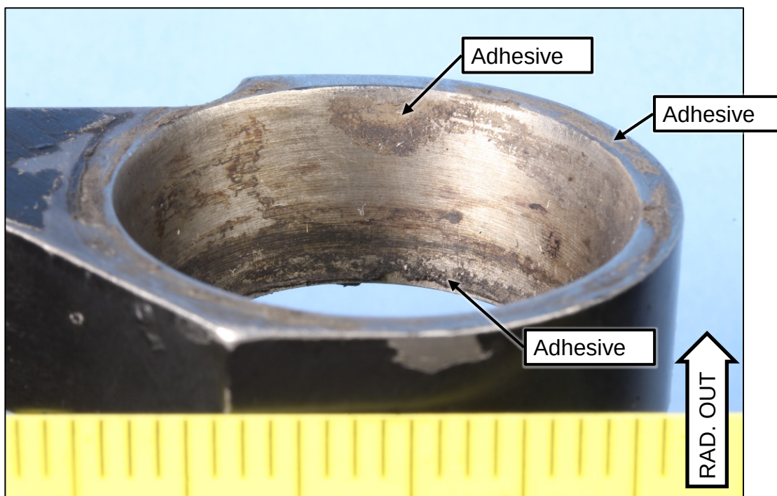
Figure 12. Fork assembly showing the seat for the missing outboard teeter bearing. Remnants of adhesive on the mating surfaces are indicated.
