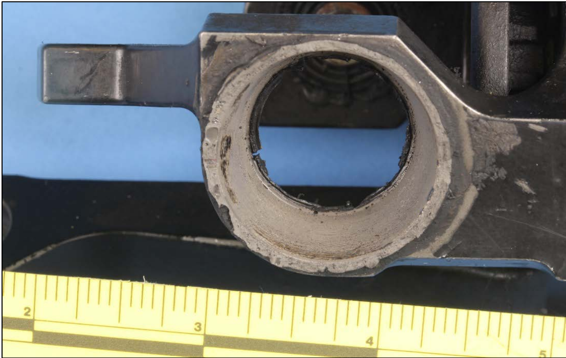
Figure 14. Inboard teeter bearing seat after the teeter bearing was removed. Gray adhesive covered the seat surface.
