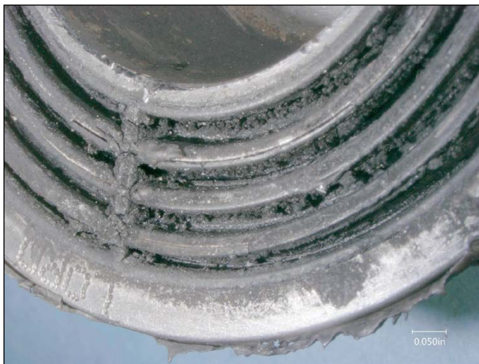
Figure 11. Close view of the radially outward side of the recovered outboard teeter bearing.
