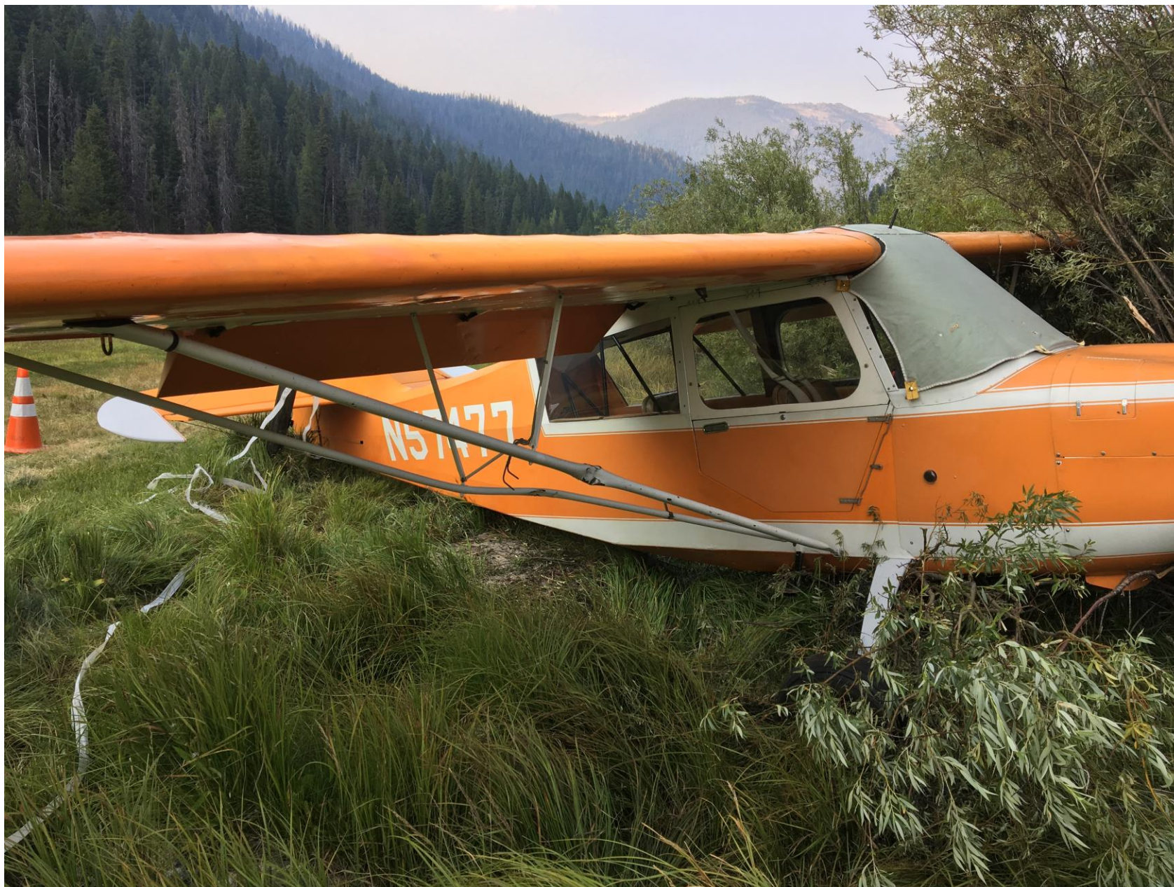
Photo 3 – N57477 showing substantial damage to right wing struts
