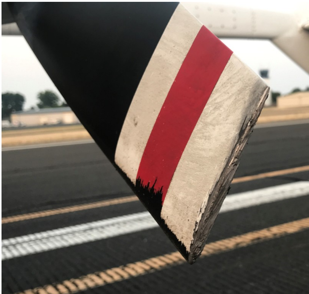
Figure 8 - Rear Propeller Tip Damage
