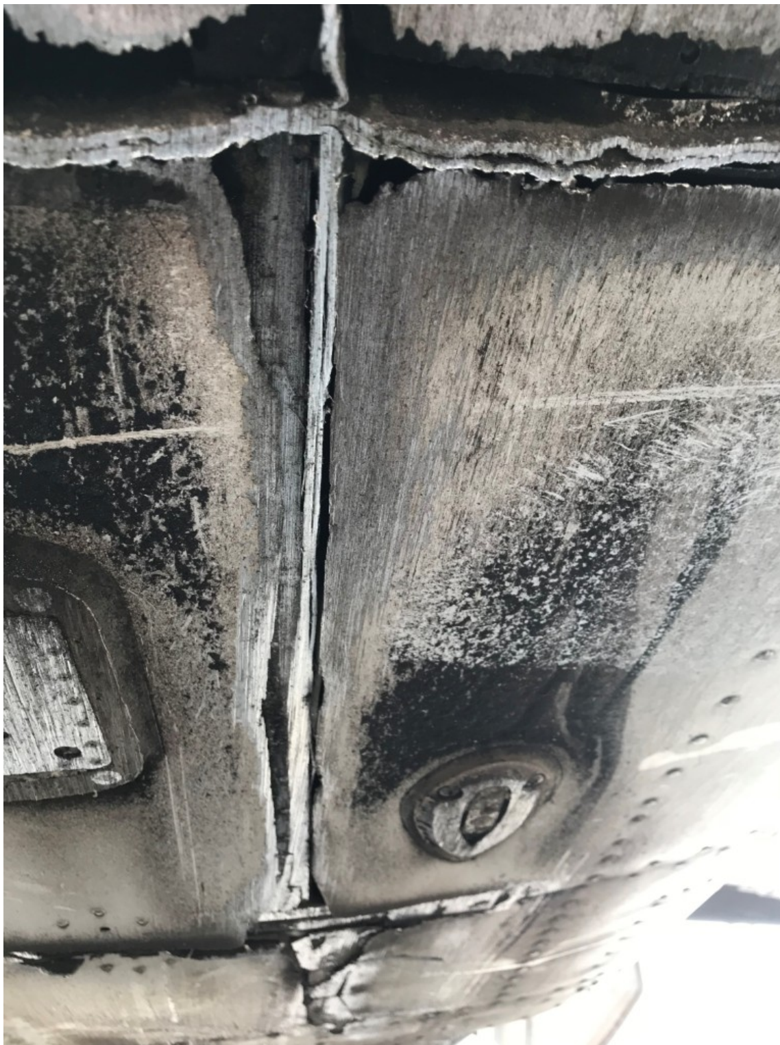
Figure 7 - Fuselage Lower Skin Damage
