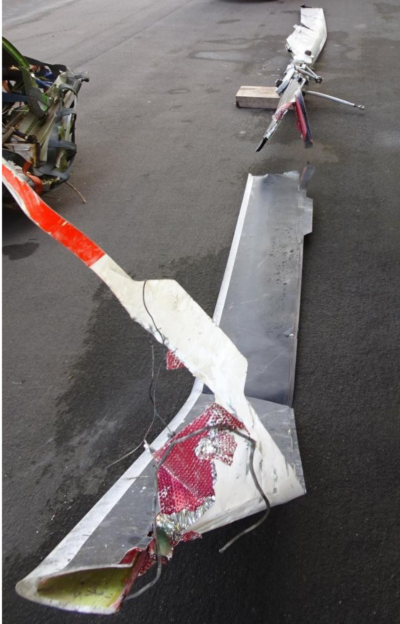
Figure 7 - Damaged Main Rotor Blade
