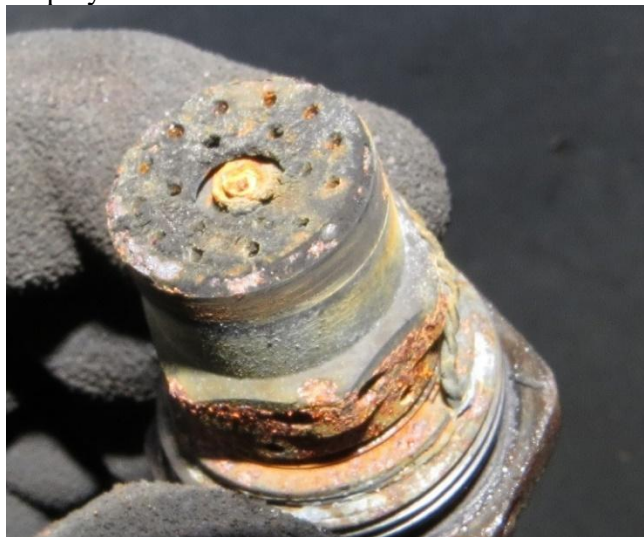
Figure 22 - Fuel Spray Nozzle Face
