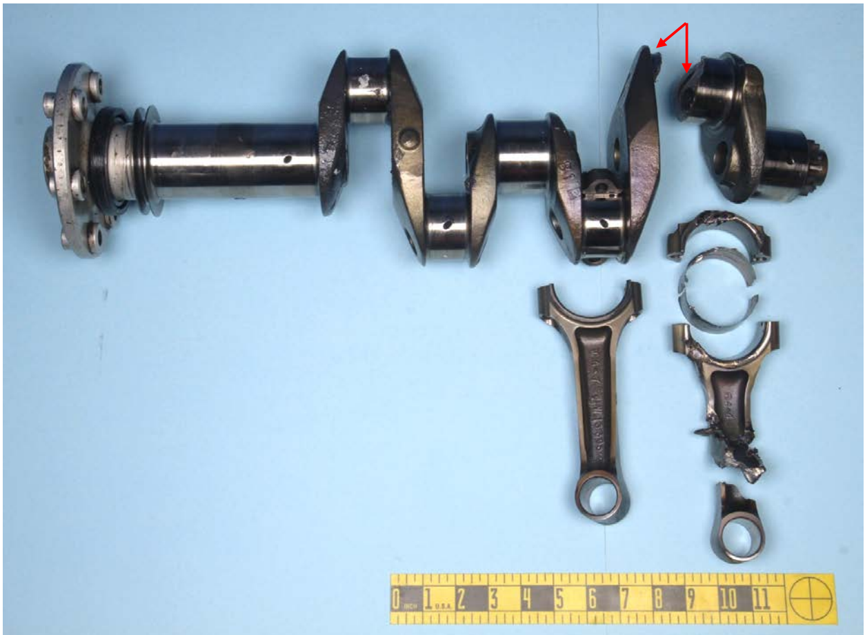
Figure 1: Overall photo showing the crankshaft and mating no. 3 and no. 4 connecting rods. The crankshaft had separated through the no. 4 bearing journal.
