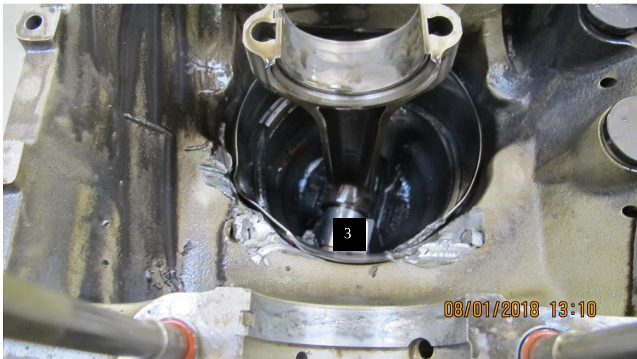
Figure 6-No. 3 Connecting Rod and Cylinder Bay Area
