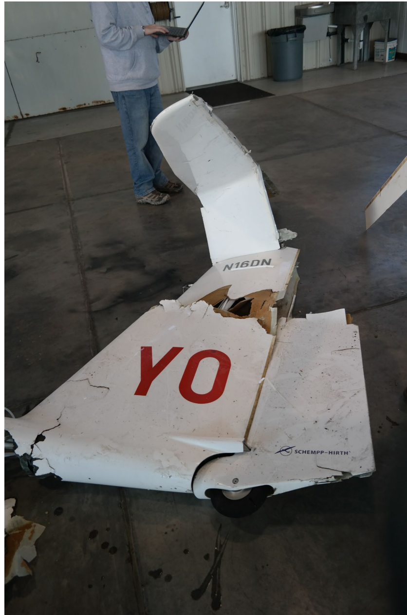
Photo 1 – Recovered tail section. Photo courtesy of Schempp-Hirth
