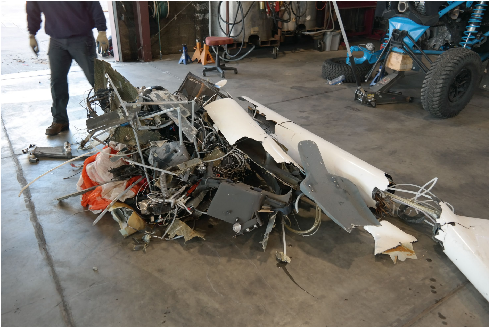
Photo 2 – Recovered fuselage. Photo courtesy of Schempp-Hirth
