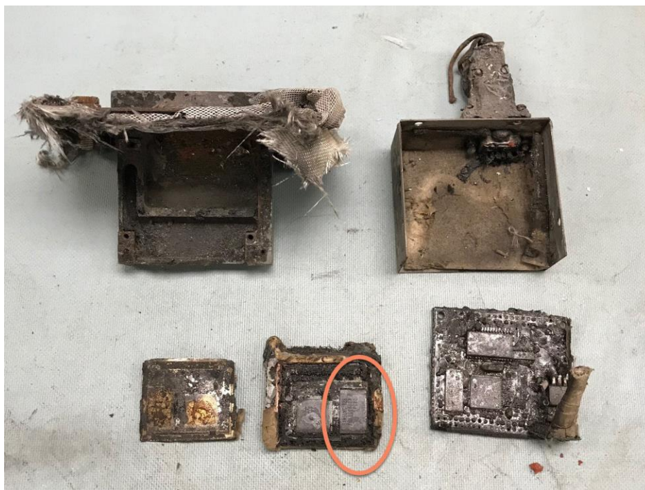
Figure 2. Photo of damaged unit opened, the NVM chip is circled in orange.
