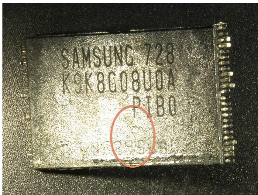
Figure 3. Photo of internal memory chip after removal and cleaning. The photo was taken at an angle to highlight the damage to the packaging. A crack on the surface of the chip packaging is circled in orange.
