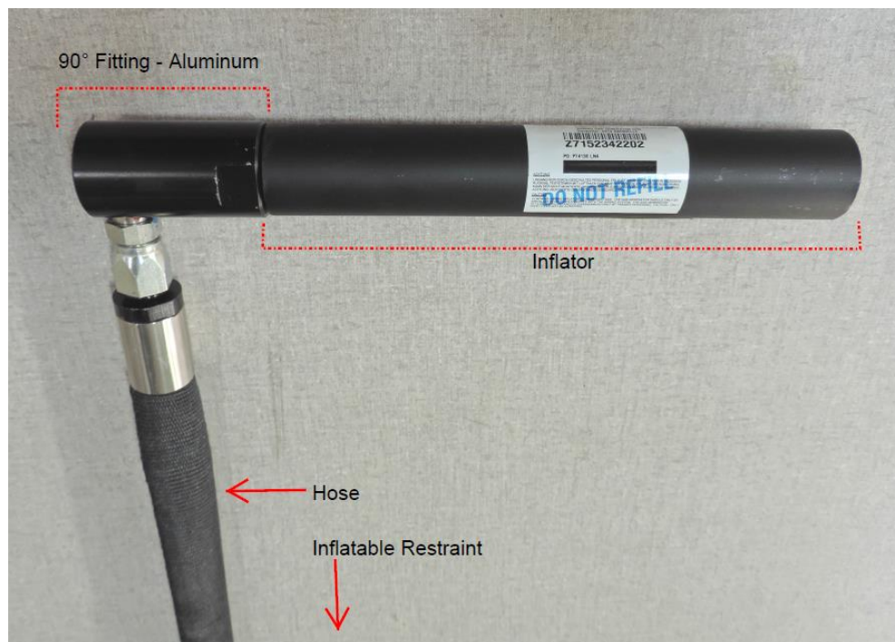
Figure 9-For Reference- Inflator interfaced and assembled to inflatable restraint
