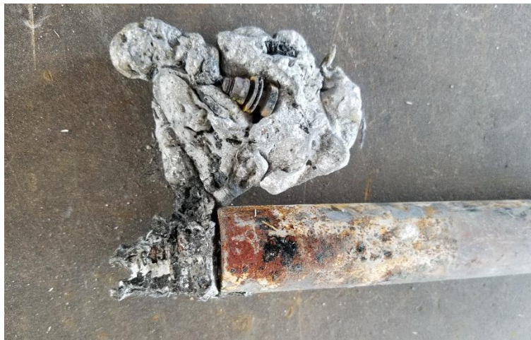
Figure 5 Inflator "2" Output End view (threaded diffuser, interface to Inflatable Restraint)
