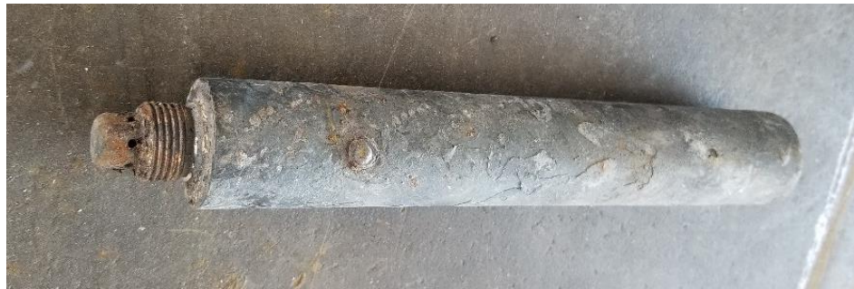
Figure 2 Inflator "1" Output End view (threaded diffuser, interface to Inflatable Restraint)
