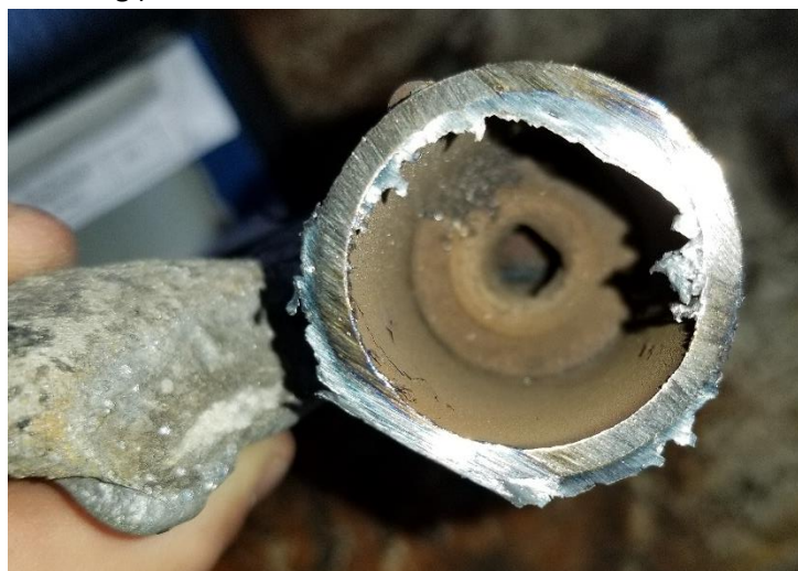
Figure 11 Inside inflator “2” body, looking at Burst Disk exit into Diffuser
