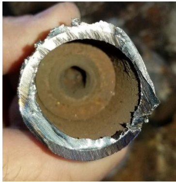
Figure 10 Inside inflator “1” body, looking at Burst Membrane exiting into Diffuser
