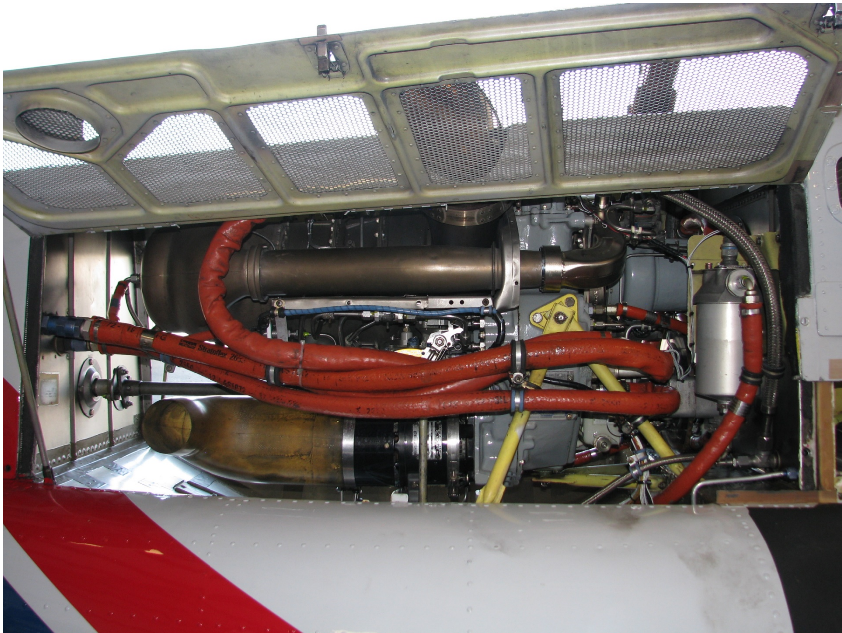
Photo 5 -Right-side view of the engine bay, showing the airframe-mounted fuel filter. Photo courtesy of the FAA.
