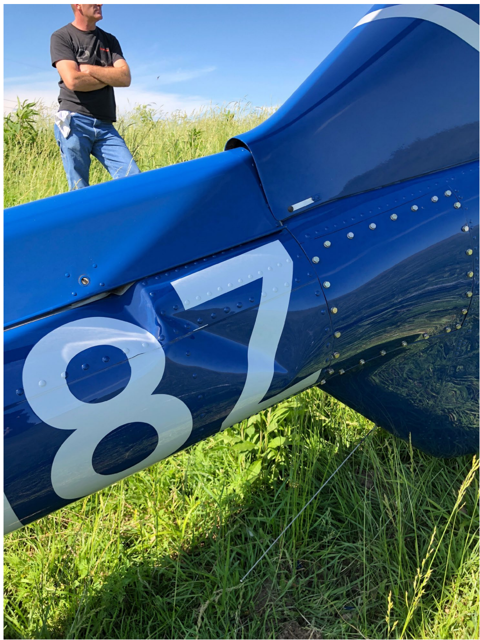
Photo 2 - View of tail boom damage. Photo courtesy of the FAA.
