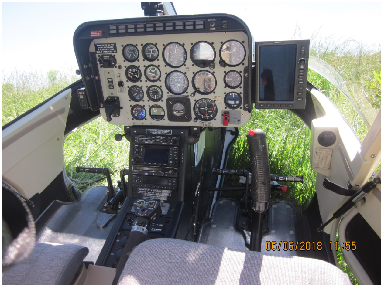
Figure 4. N518Z, instrument panel. Photo courtesy of the FAA.
