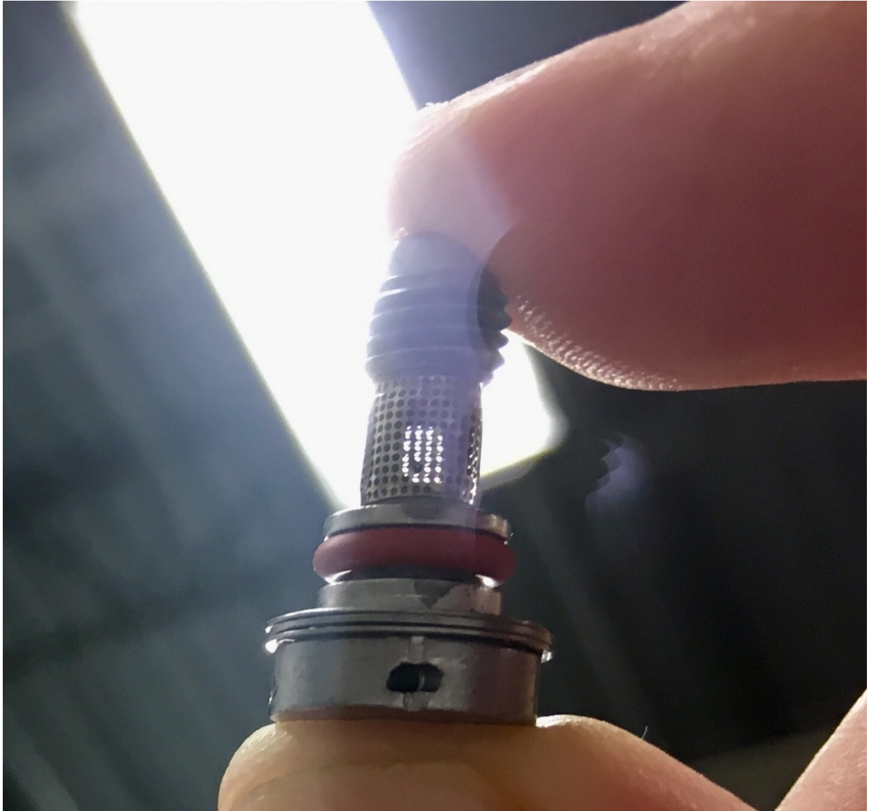
Figure 9. Debris noted in the restrictor and filter assembly.
