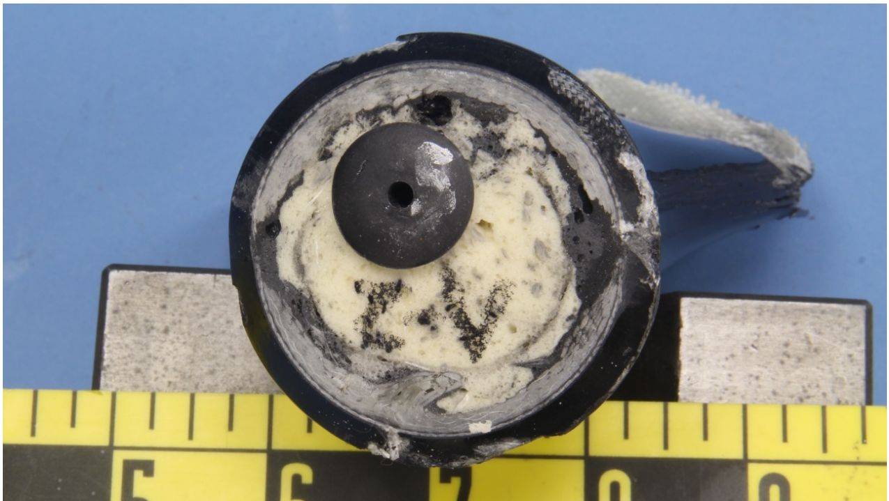
Figure 3 – The base of the fractured propeller blade, showing chatter marks on the seat ridge.
