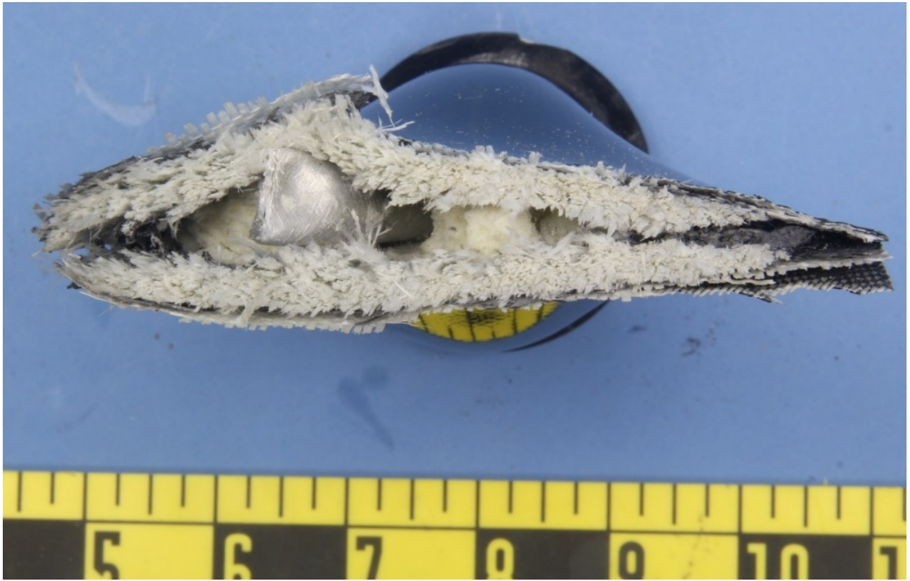
Figure 2 – The transverse fracture surface of the propeller blade, showing fiber fraying and pullout, with tearing of the skin and internal foam core.
