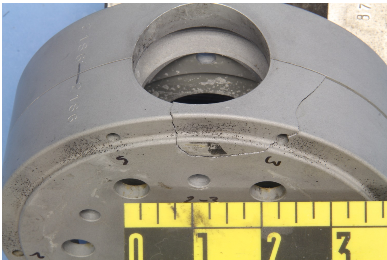
Figure 7 – View of the cracked hub from the 2-3 blade seat position, viewed from the aft side.
