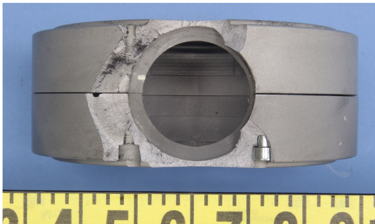
Figure 5 – View of the fracture surface from the blade seat in position 1-2.
