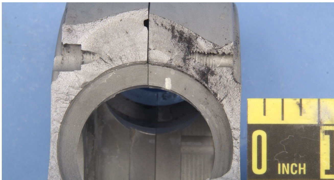
Figure 6 – View of the progressive region of the 1-2 fracture, showing crack arrest and ratchet marks.
