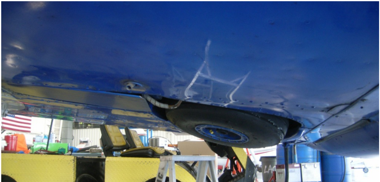
Figure 4 - RMLG Retracted by Normal System Operation
