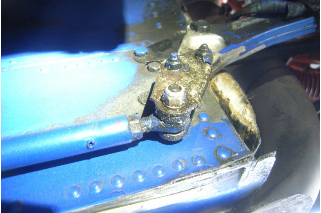
Figure 3 - NLG Actuating Rod with Adjustable Rod End
