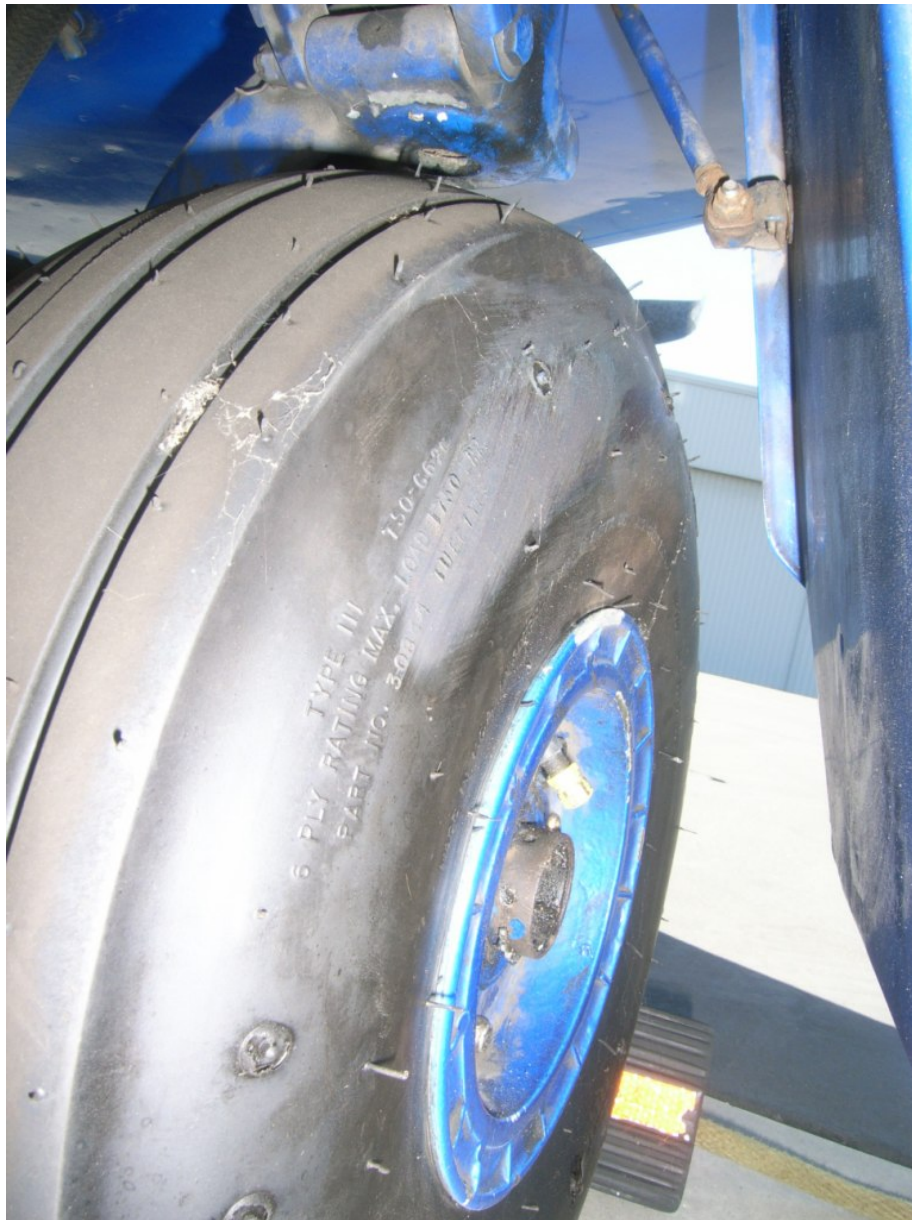
Figure 4 - RMLG Tire and Wheel Scuff Marks
