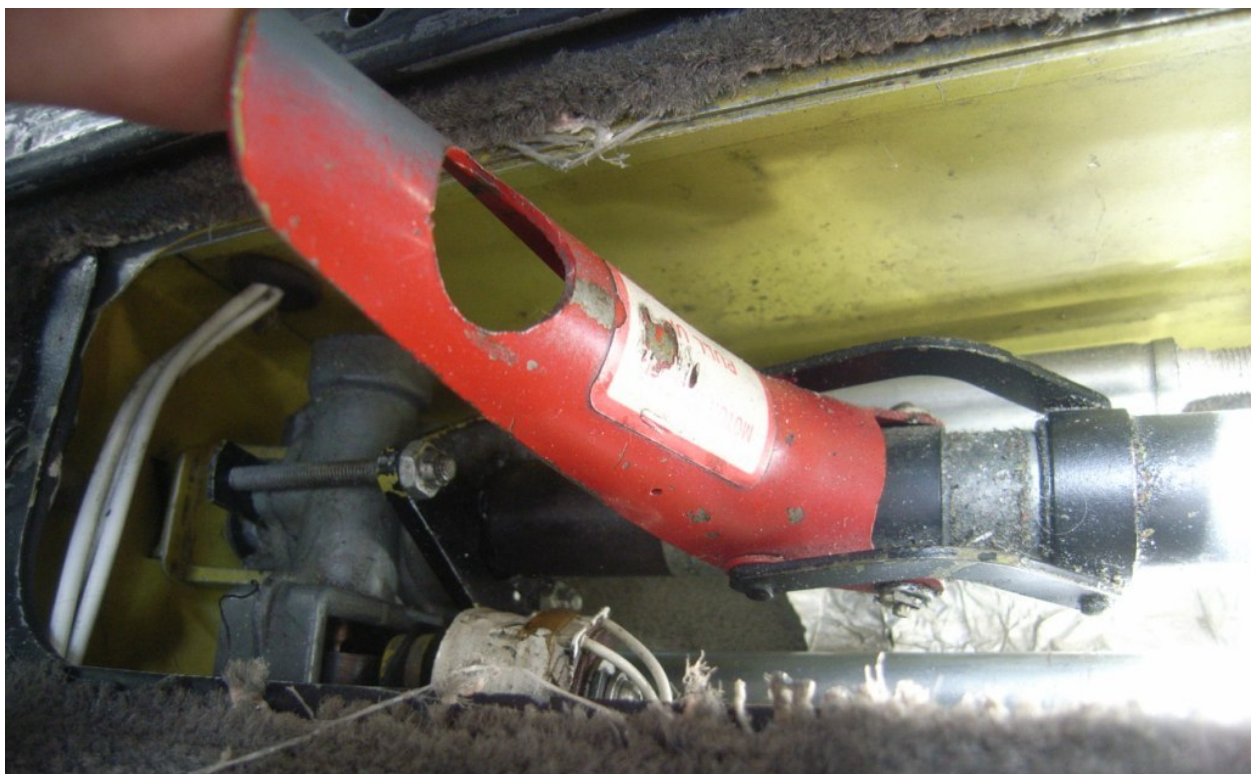
Figure 3 - Close Up of Release Handle (lifted but not actuated)
