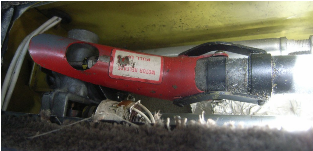
Figure 2 - Close Up of Release handle (rest position)
