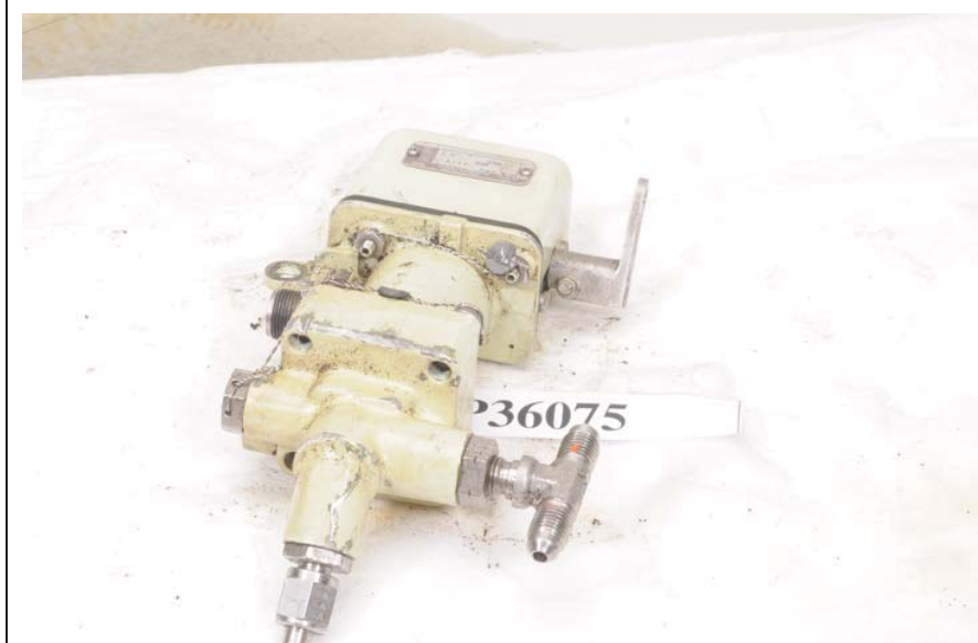
Figure 180. Fuel Shutoff Valve
