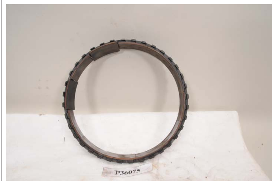
Figure 142. First Stage Turbine Shroud
