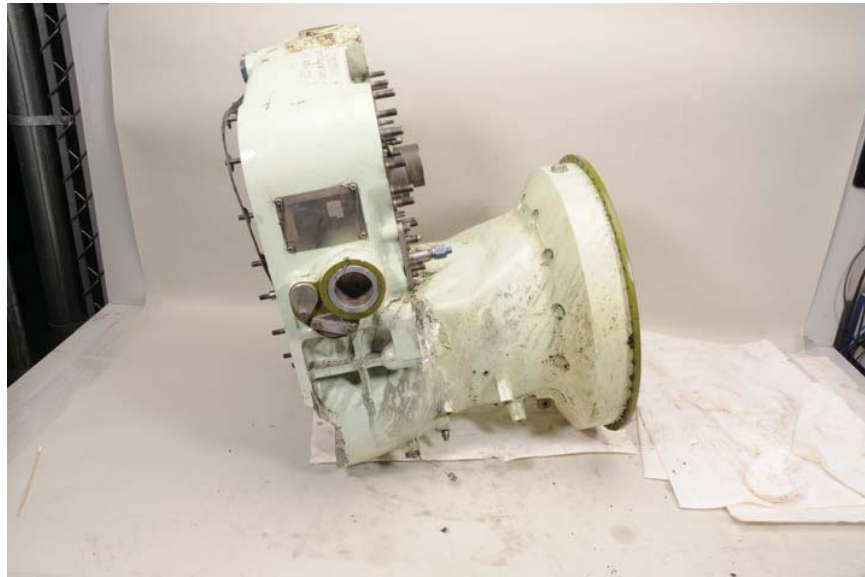
Figure 69. Gearcase Housing (Exterior)
