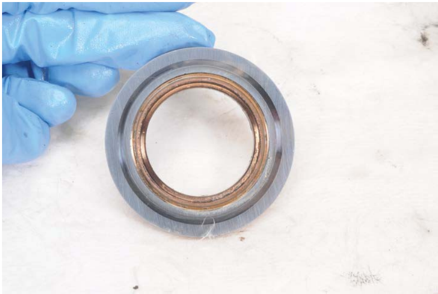
Figure 84. Compressor Carbon Seal Rotor
