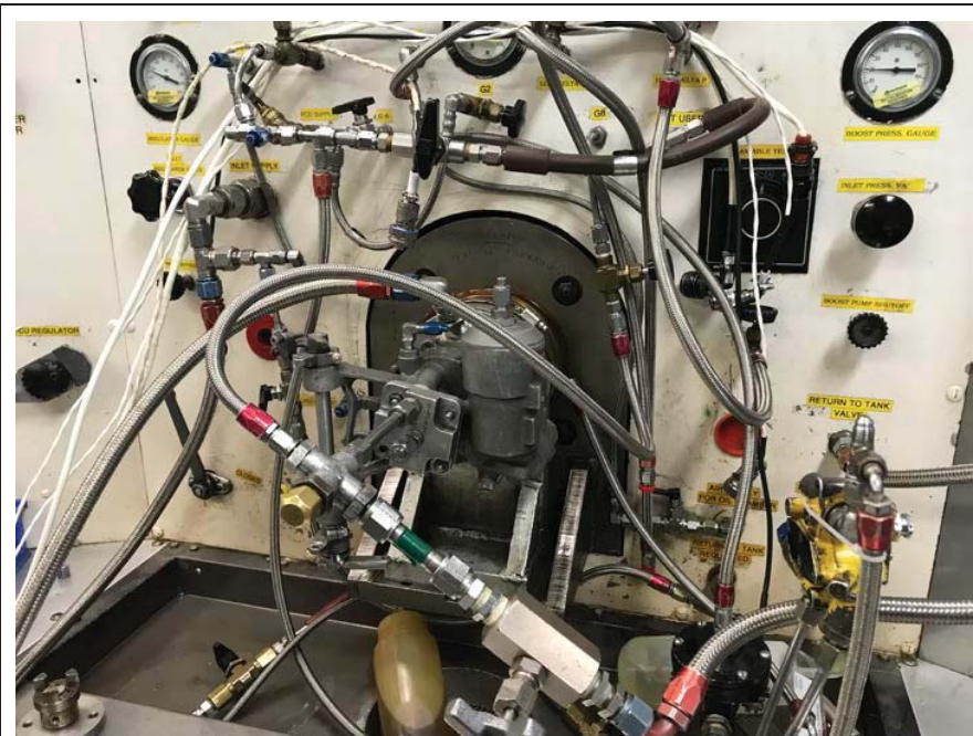
Figure 217. Functional Testing of Fuel Pump Assembly
