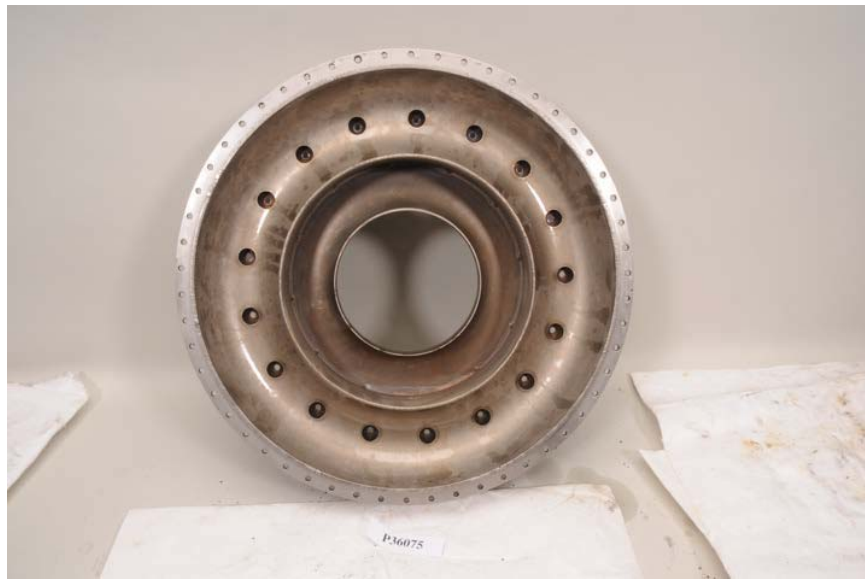
Figure 121. Second-Stage Compressor Housing
