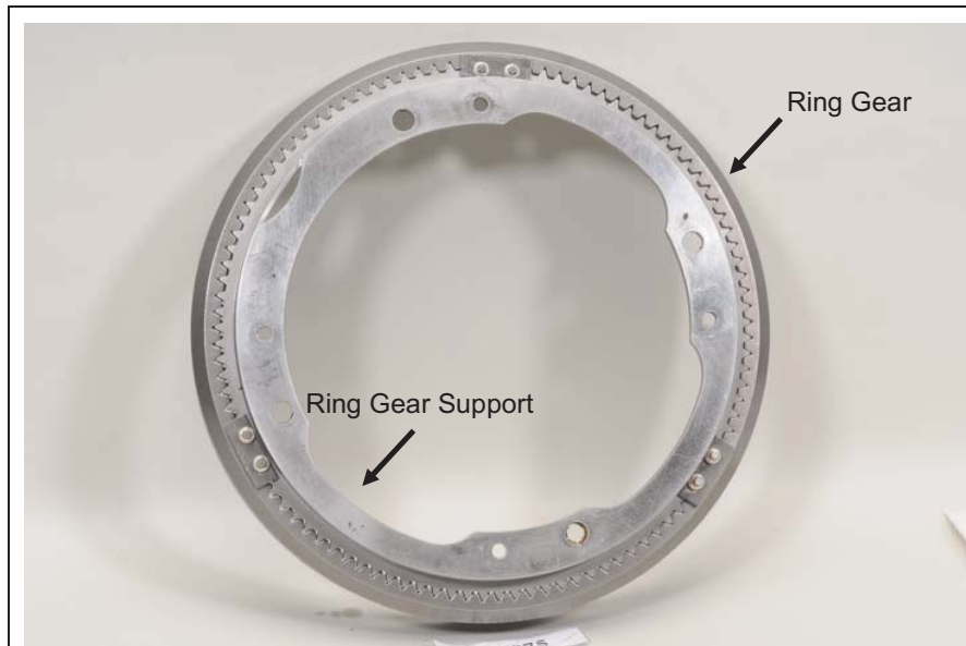
Figure 39. Ring Gear / Ring Gear Support
