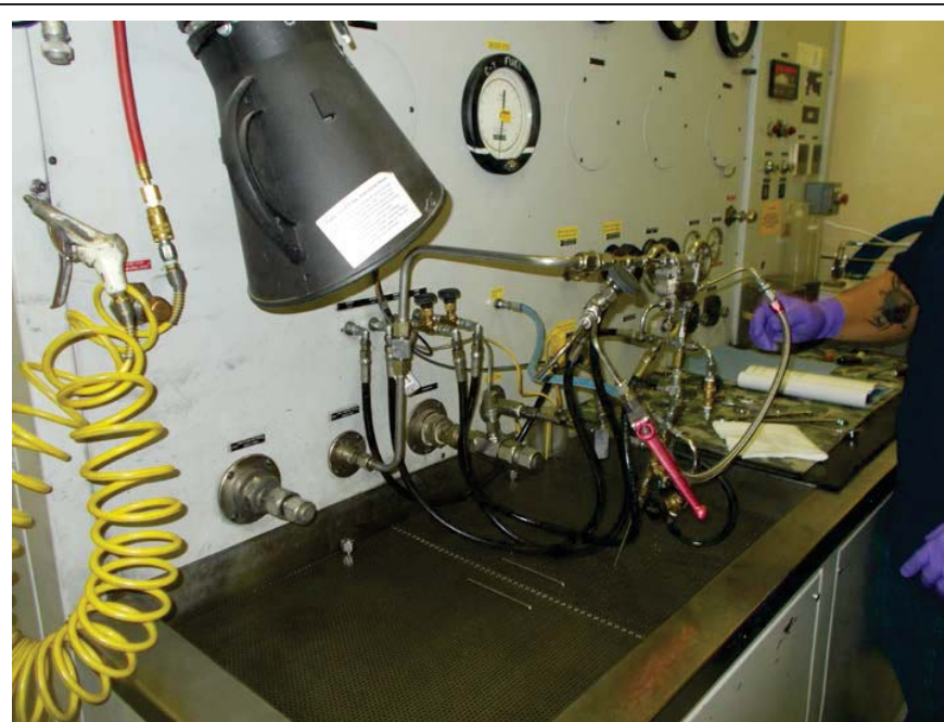
Figure 219. Functional Testing of Fuel Flow Divider Valve
