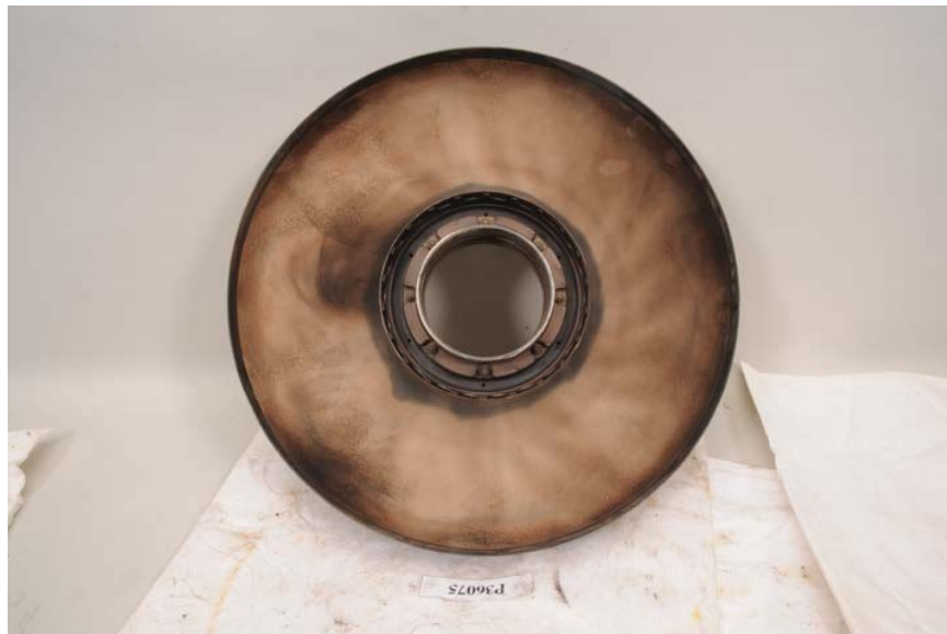
Figure 133. Outer Transition Liner
