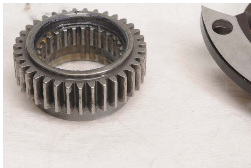
Figure 105. Main Shaft Gear
