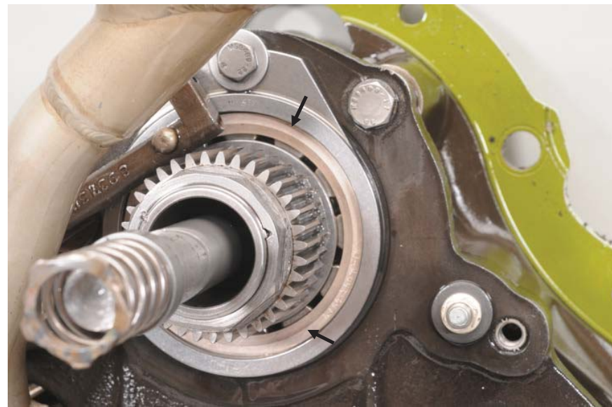
Figure 54. Aft High-Speed Pinion Bearing
