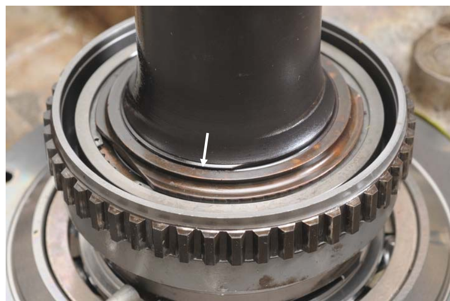
Figure 31. Propeller Shaft Lock Nut
