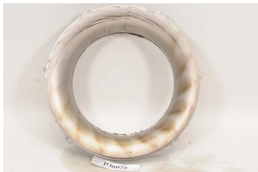
Figure 109. First-Stage Compressor Impeller Shroud
