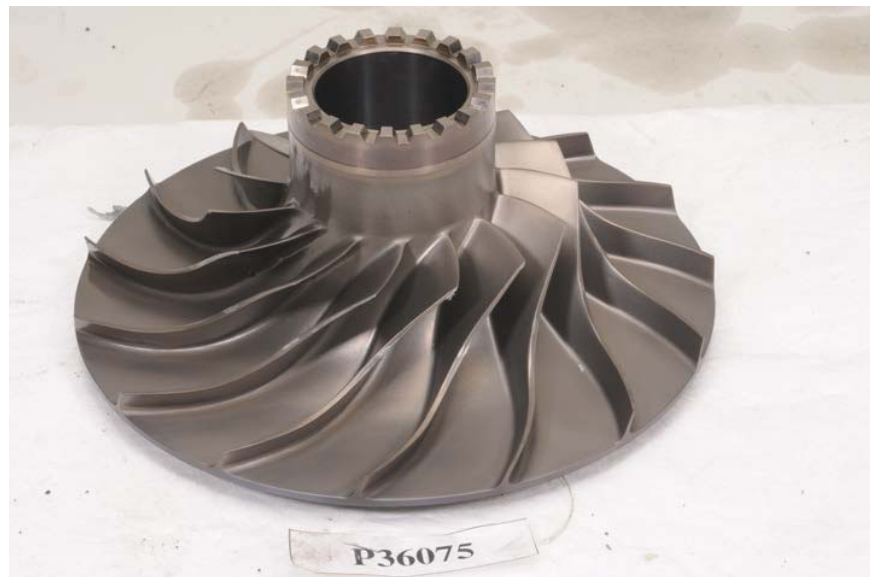
Figure 126. Second-Stage Compressor Impeller
