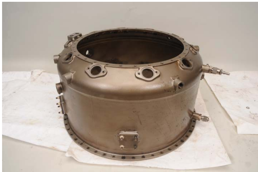
Figure 130. Combustor Plenum Case
