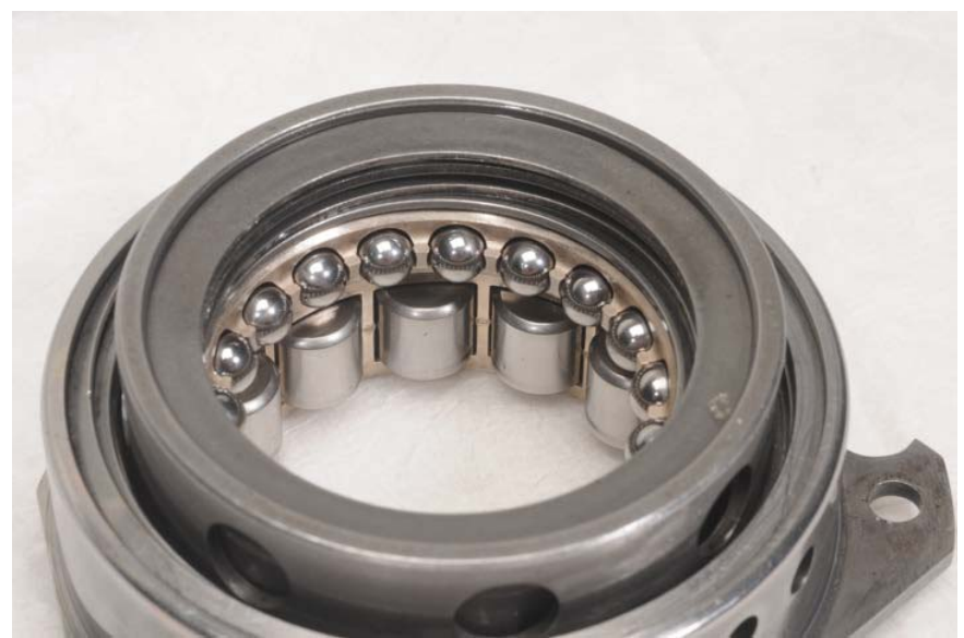
Figure 76. Propeller Shaft Aft Ball Bearing
