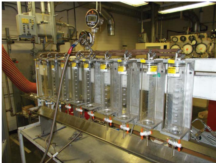
Figure 222. Functional Testing of Fuel Manifold and Nozzle Assembly
