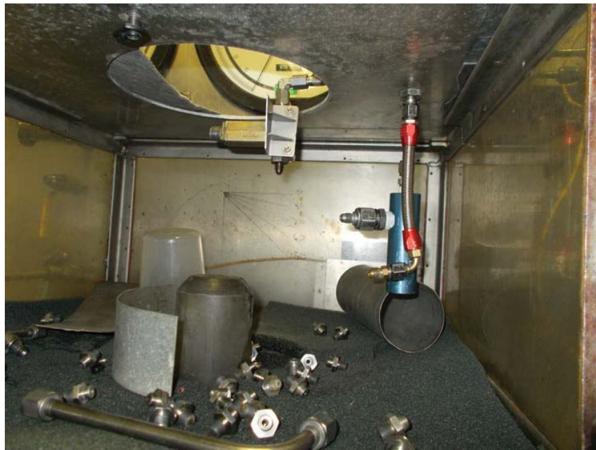
Figure 221. Functional Testing of Fuel Enrichment Solenoid
