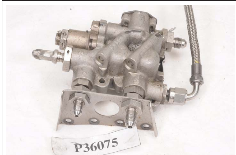
Figure 190. Fuel Flow Divider
