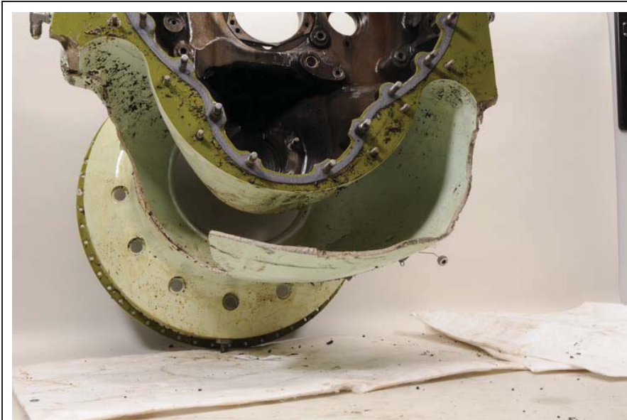
Figure 71. Gearcase Housing (Exterior)
