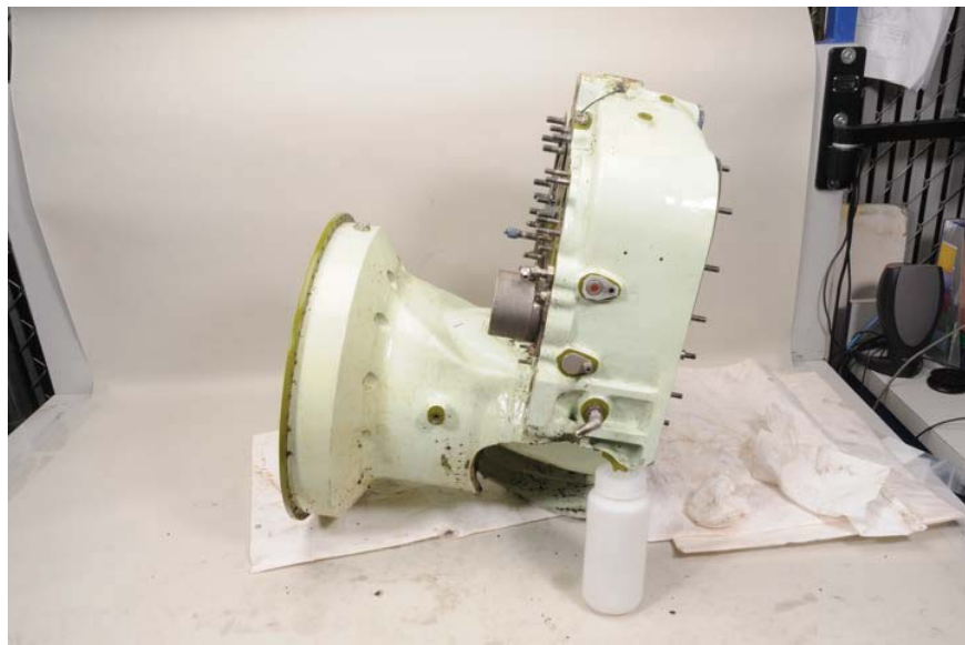
Figure 68. Gearcase Housing (Exterior)
