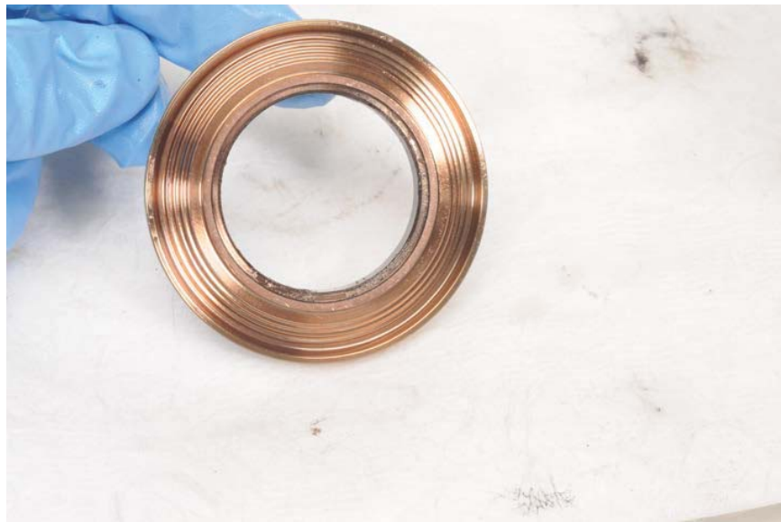
Figure 85. Compressor Carbon Seal Rotor
