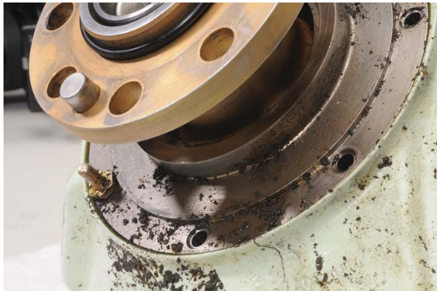
Figure 29. Forward Propeller Shaft Bearing Mount Bolts
