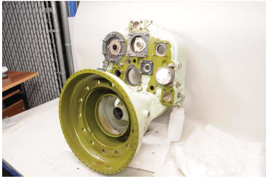
Figure 67. Gearcase Housing (Exterior)
