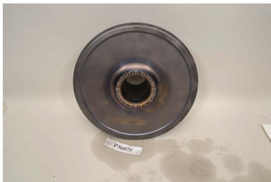
Figure 125. Second-Stage Compressor Impeller
