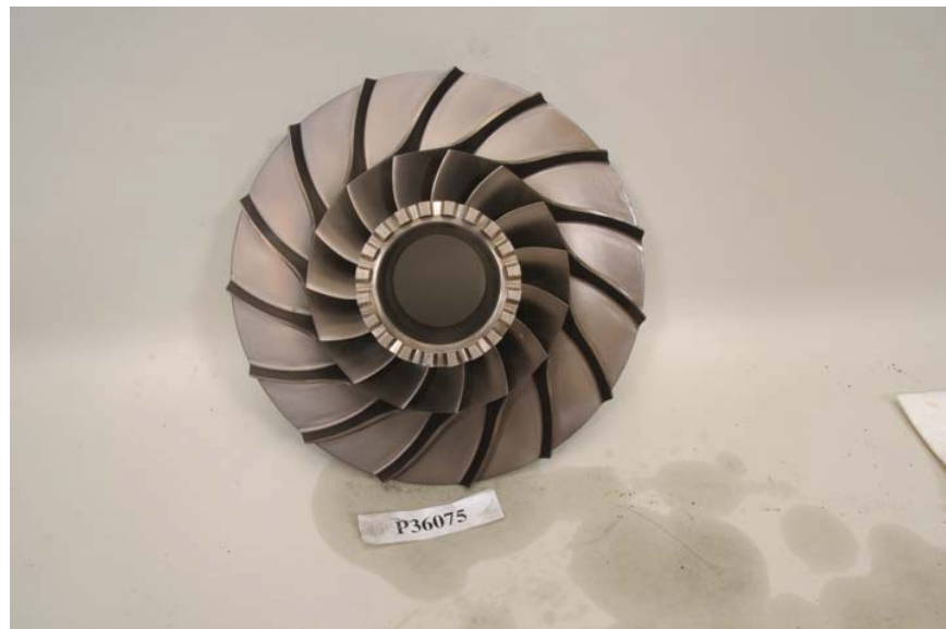
Figure 124. Second-Stage Compressor Impeller
