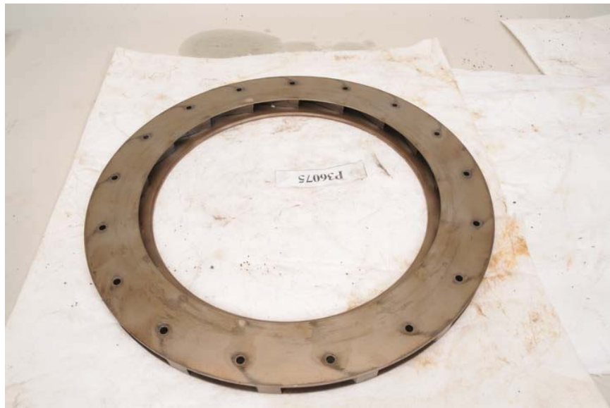
Figure 129. Second-Stage Compressor Diffuser Vane Assembly
