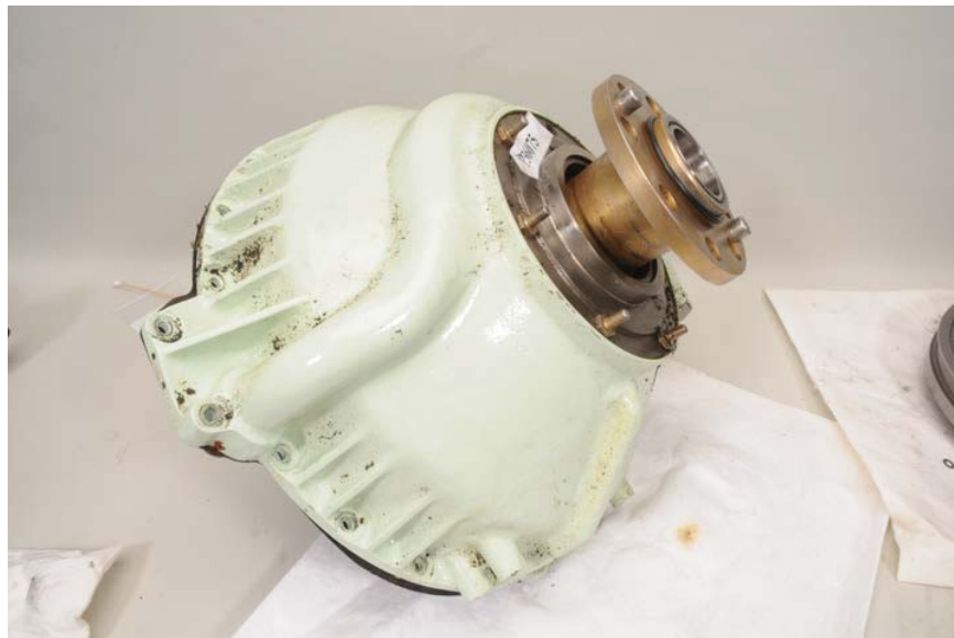
Figure 23. Nose Cone Housing
