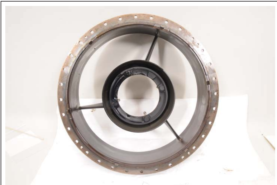
Figure 169. Turbine Bearing Support
