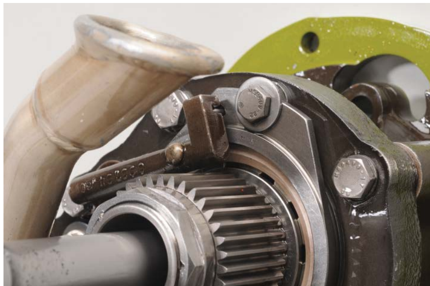
Figure 52. High-Speed Pinion (HSP)
