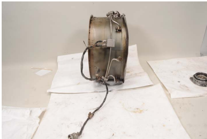
Figure 166. Engine Exhaust Duct
