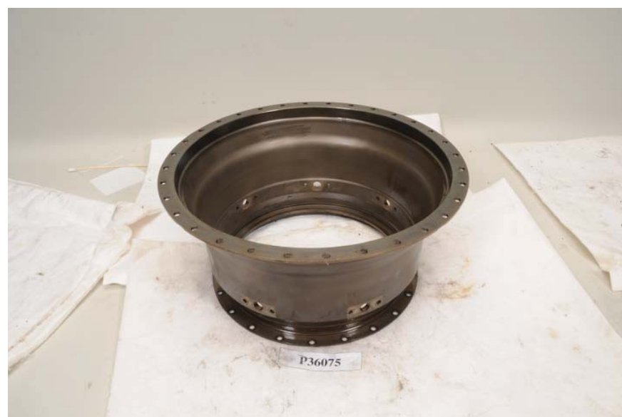
Figure 139. Turbine Stator Housing
