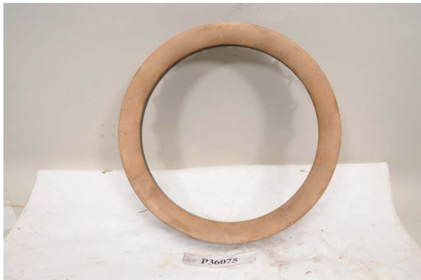
Figure 134. Inner Transition Liner
