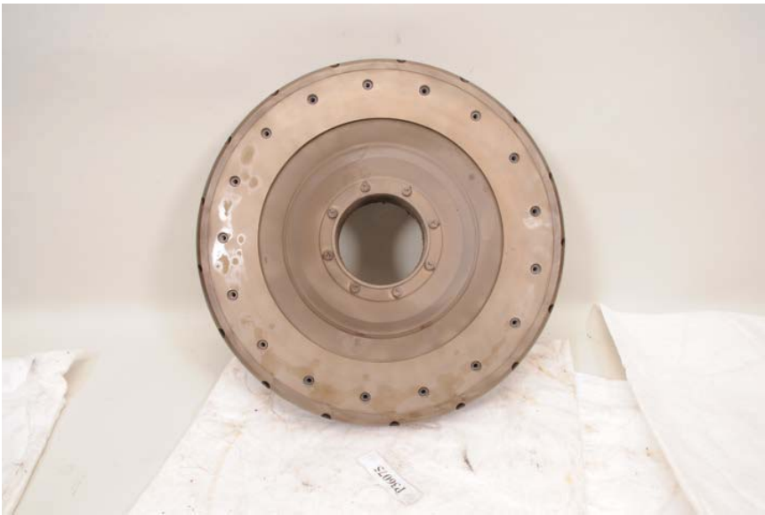
Figure 132. Outer Transition Liner
