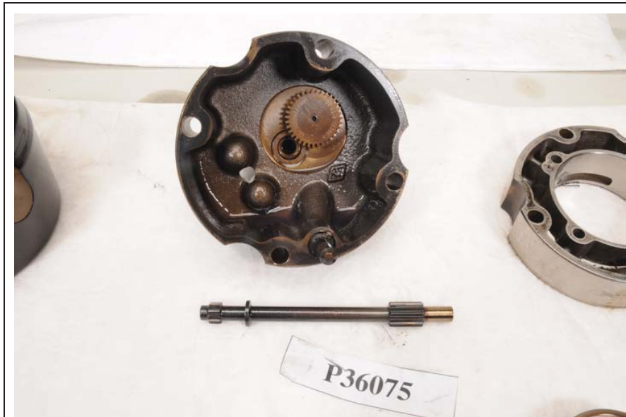
Figure 175. Turbine Oil-Scavenge Pump and Drive Shaft
