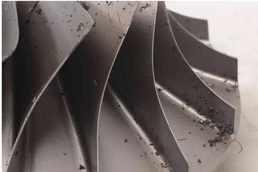
Figure 117. First-Stage Compressor Impeller
