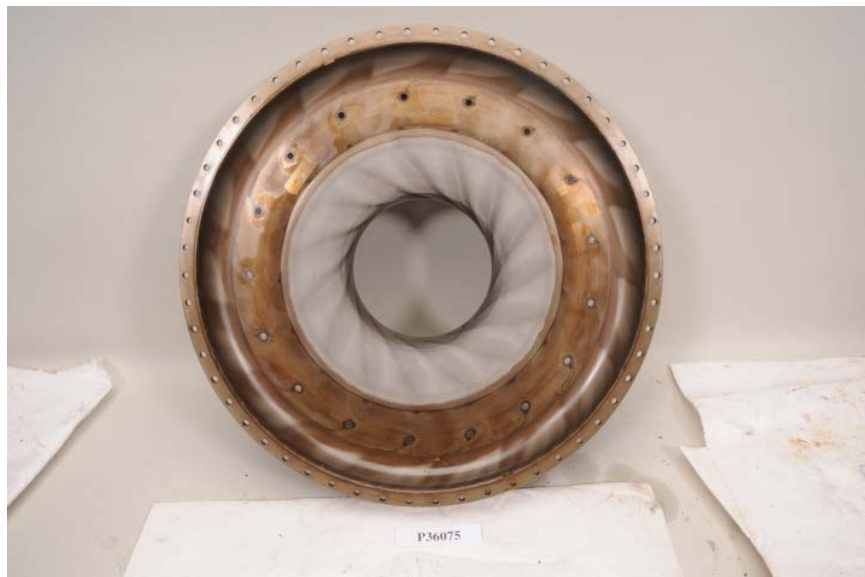
Figure 122. Second-Stage Compressor Housing
