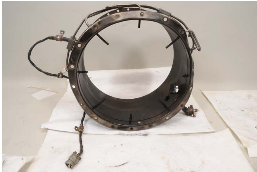
Figure 165. Engine Exhaust Duct
