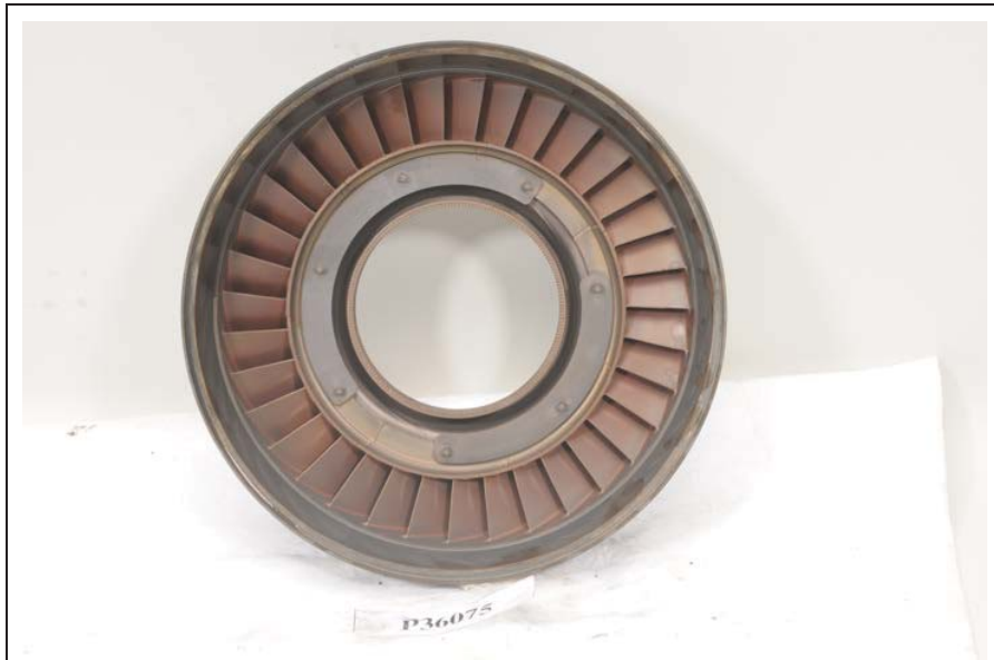
Figure 149. Second-Stage Turbine Stator
