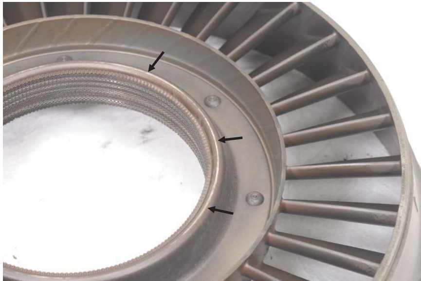
Figure 160. Third-Stage Turbine Stator
