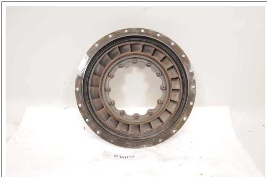
Figure 141. First-Stage Turbine Stator Assembly
