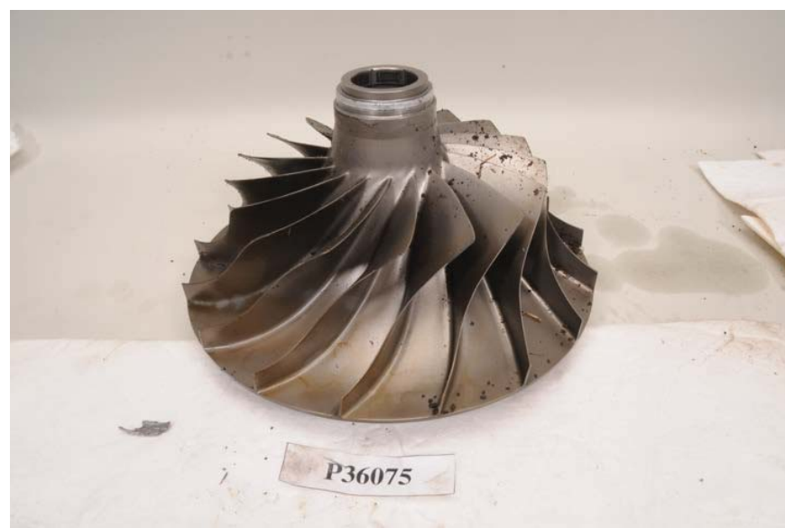
Figure 115. First-Stage Compressor Impeller
