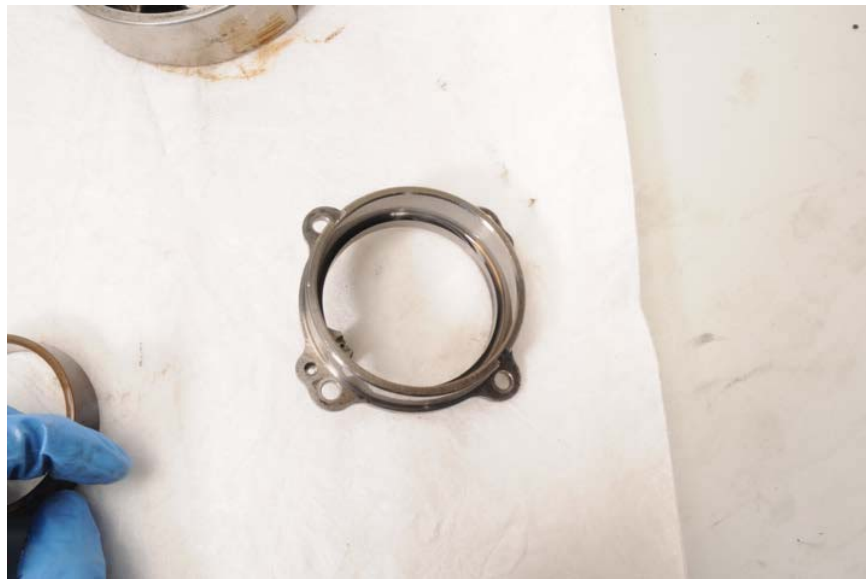
Figure 173. Turbine Bearing Retainer
