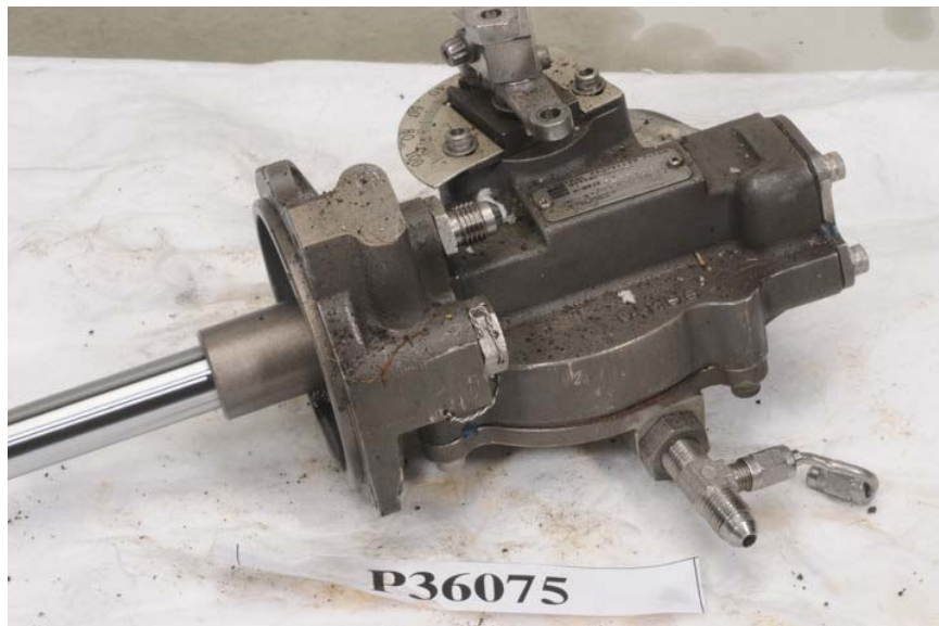
Figure 192. Propeller Pitch Control
