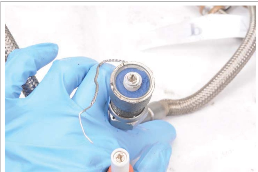
Figure 201. Exciter to Ignitor Lead Assemblies
