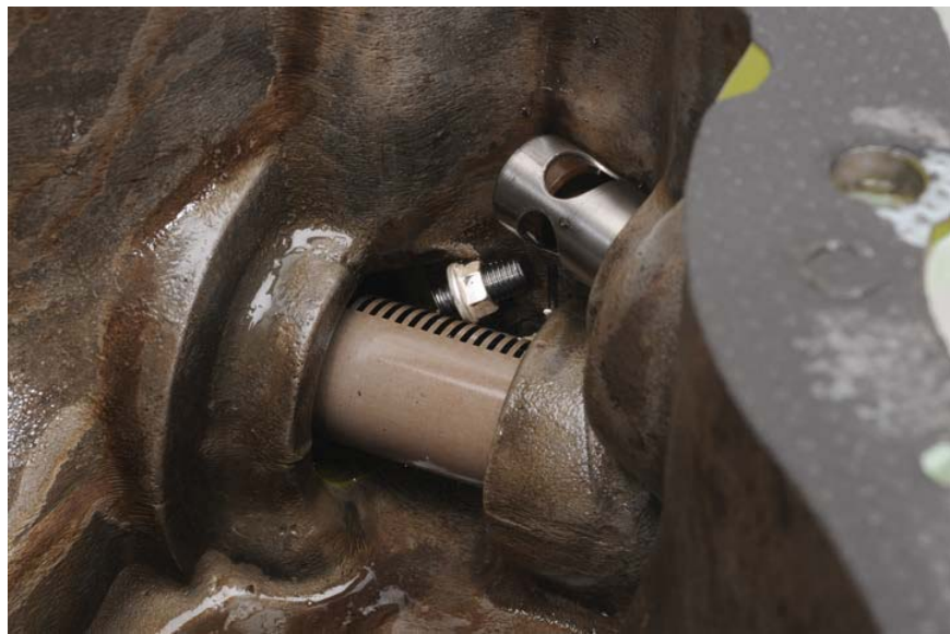
Figure 30. Forward Propeller Shaft Bearing Mount Bolts
