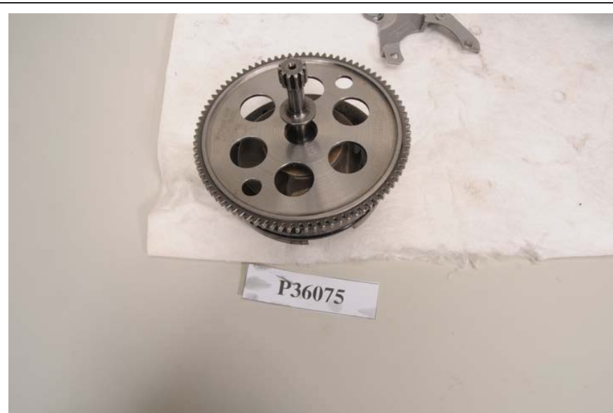
Figure 65. Gearcase Oil-Scavenge Pump Drive Idler Gear and Drive Shaft
