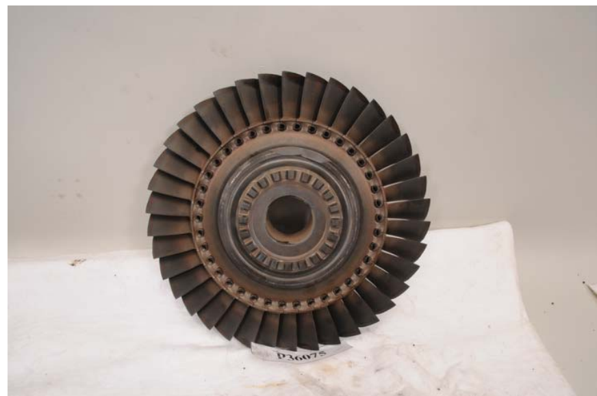
Figure 154. Second-Stage Turbine Rotor
