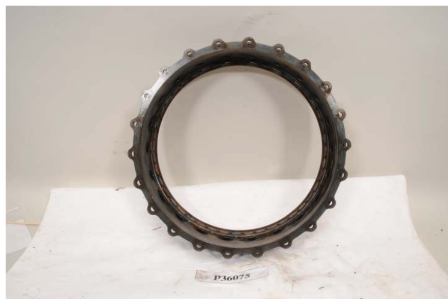
Figure 135. Inner Transition Liner
