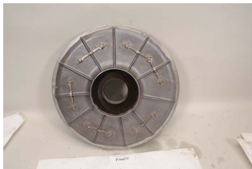
Figure 119. First-Stage Compressor Diffuser (Crossover Duct)
