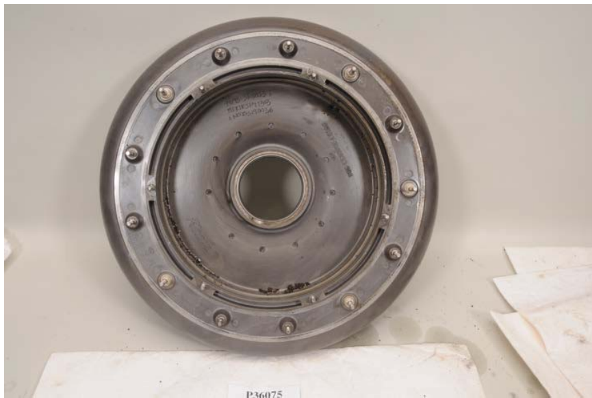
Figure 118. First-Stage Compressor Diffuser (Crossover Duct)
