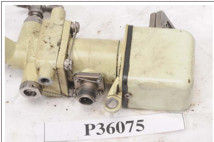
Figure 181. Fuel Shutoff Valve
