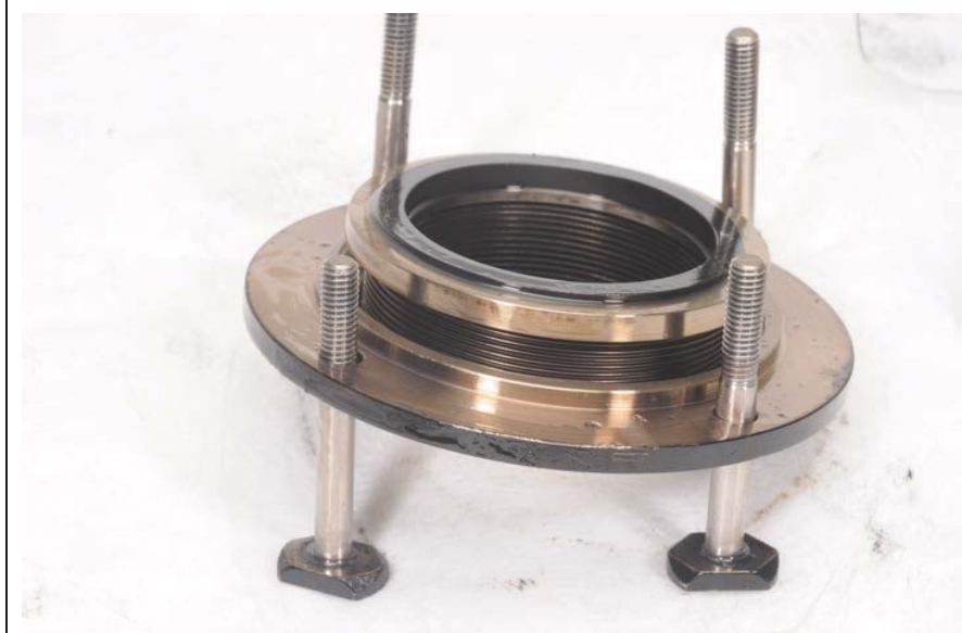
Figure 176. Turbine Air/Oil Carbon Seal
