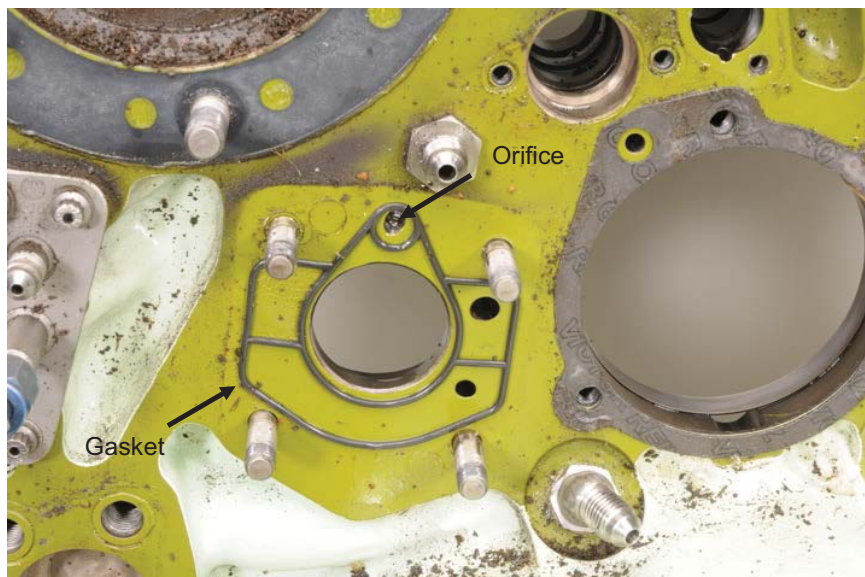
Figure 92. Propeller Governor "Spider" Gasket and "Lee" Check Valve and Orifice Assembly
