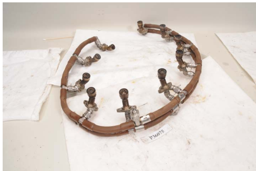
Figure 210. Fuel Manifold and Nozzle Assembly
