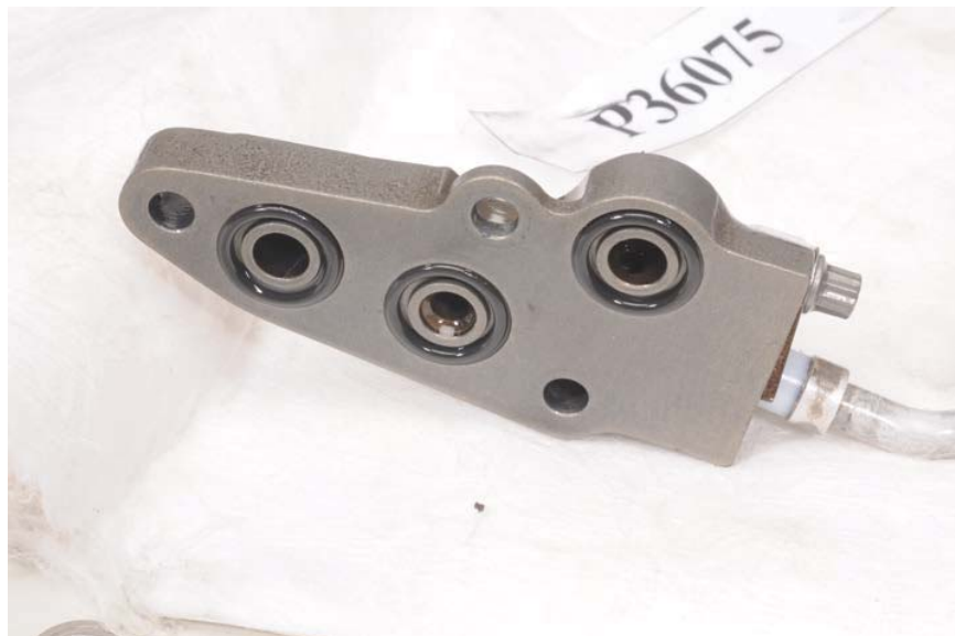
Figure 102. Hydraulic Oil Torque Sensor Output
