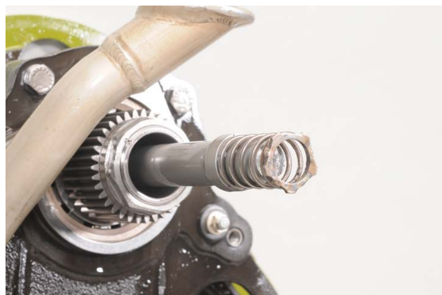
Figure 55. HSP-to-Power Section Coupling Shaft
