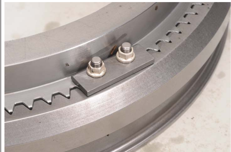
Figure 42. Ring Gear Retainers
