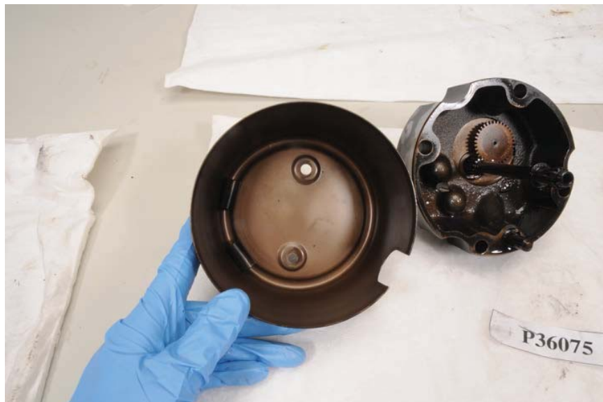
Figure 174. Turbine Sump Cover
