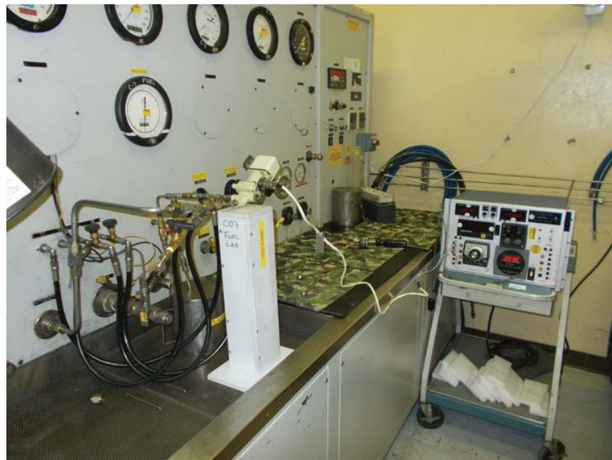
Figure 214. Functional Testing of Fuel Shutoff Valve
