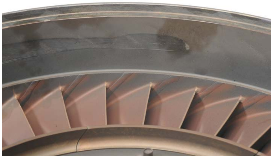
Figure 150. Second-Stage Turbine Stator
