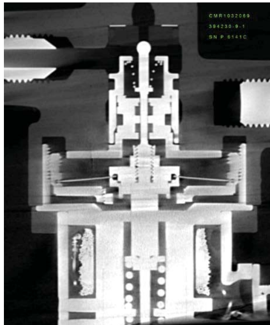
Figure 215. Fuel Shutoff Valve CT Scan
