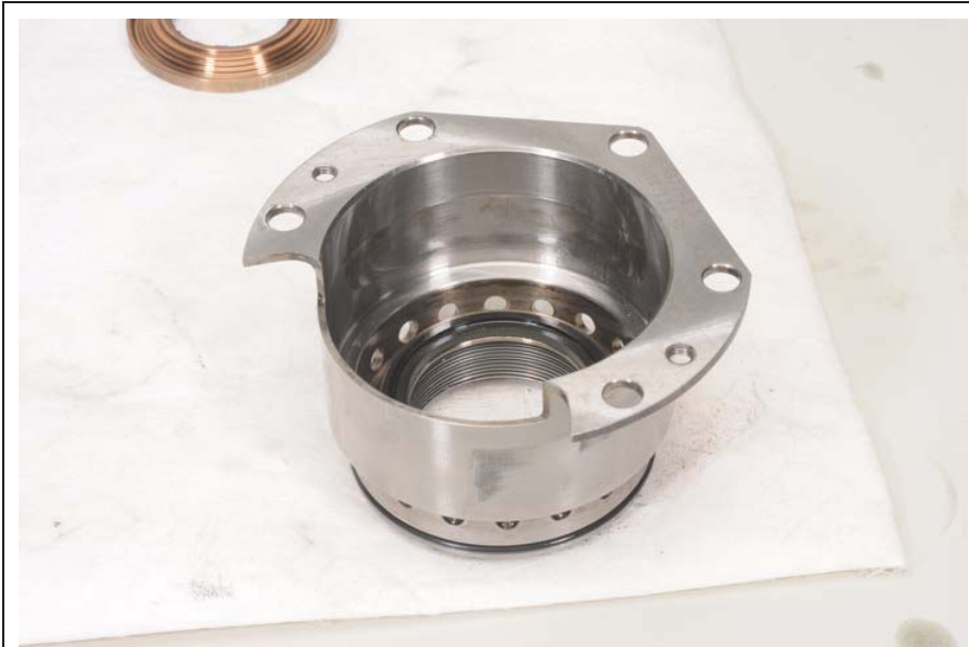
Figure 83. Compressor Air/Oil Carbon Seal
