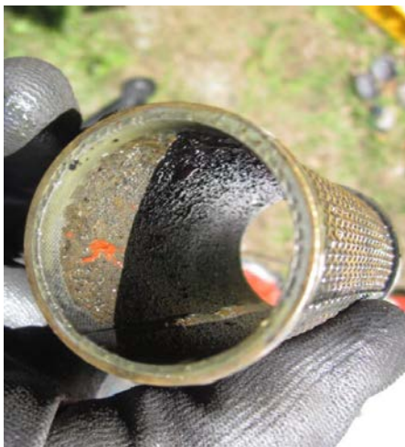
Figure 7 - view of oil screen
