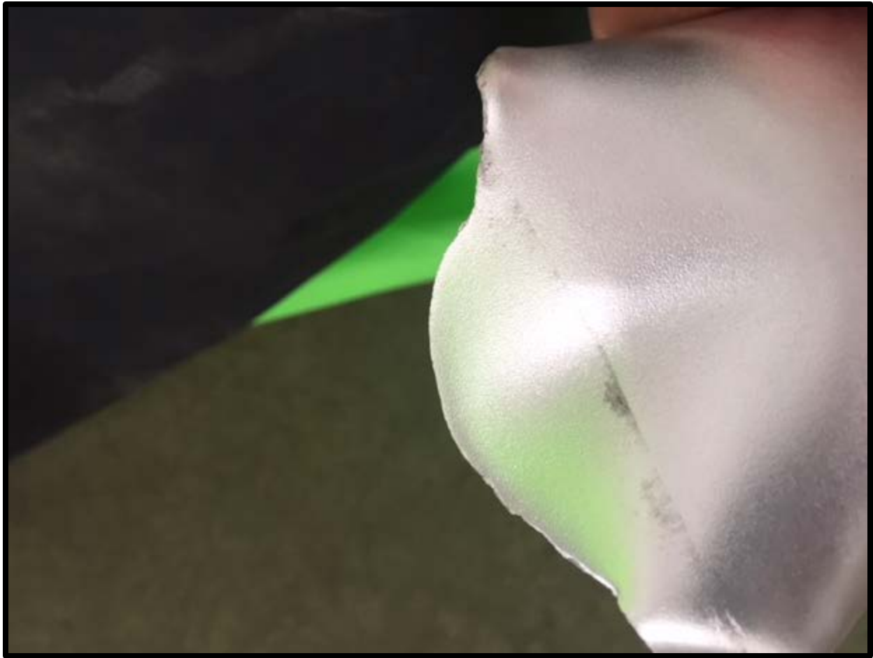
Figure 3: Fracture Upper Surface
