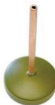
WAG AERO fuel cap E-476-200 Vent tube to be bent facing forward.
