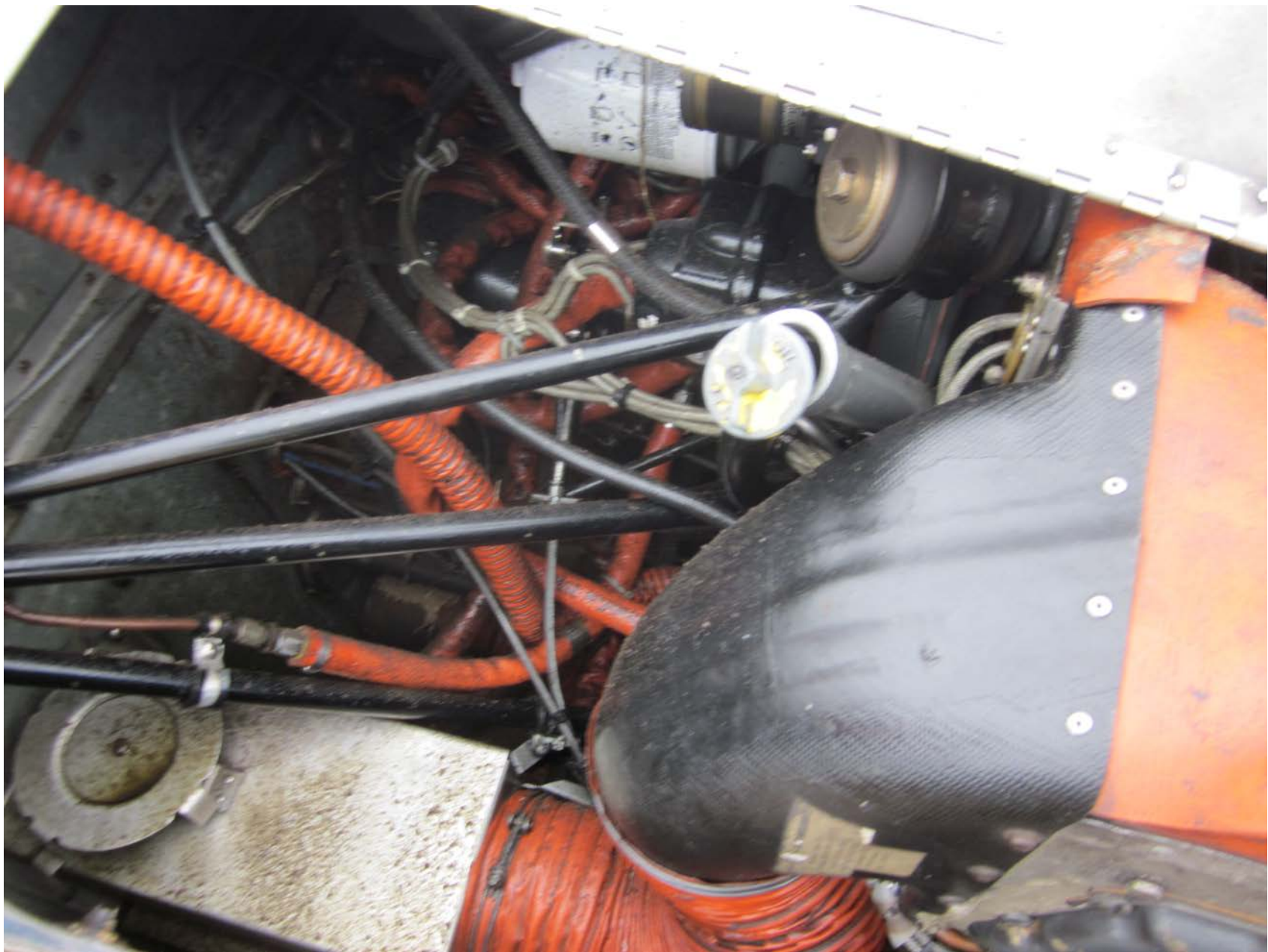
Photo 3 – Oil splattered around the engine
