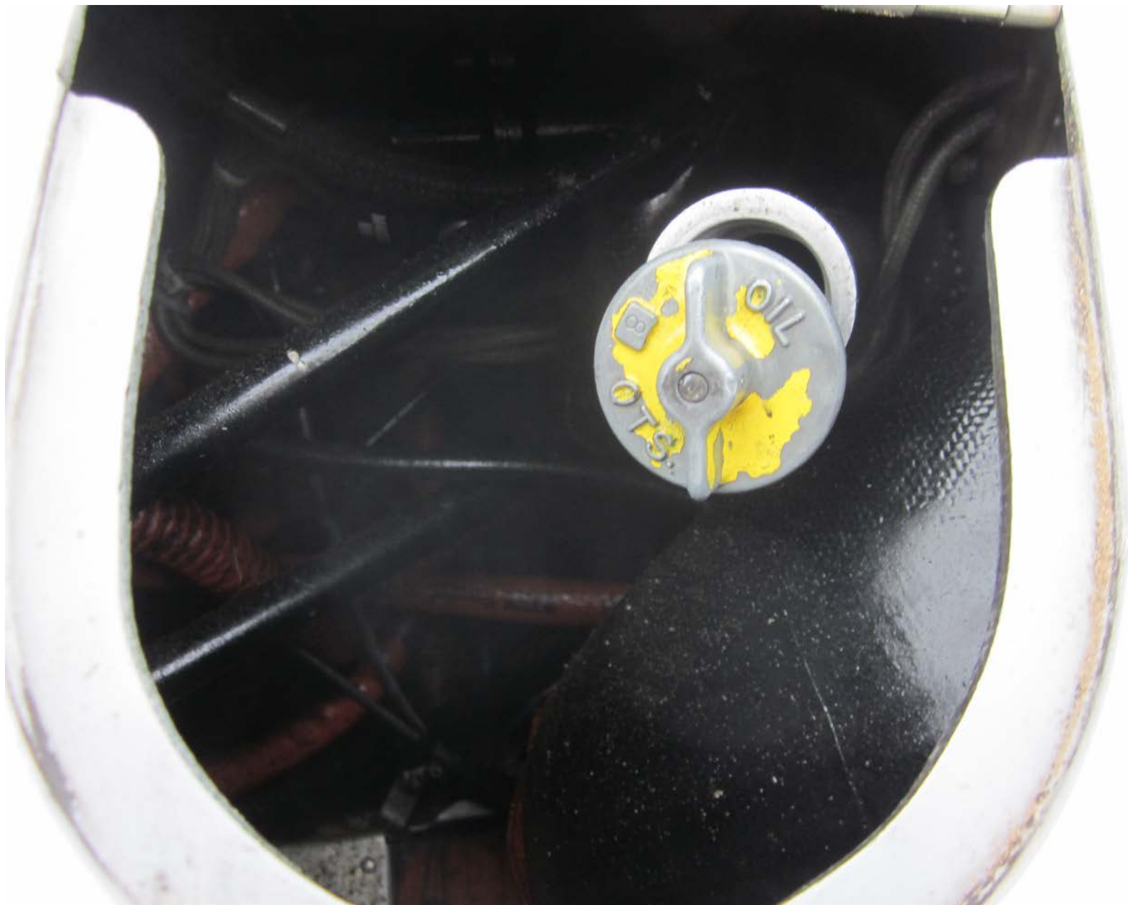
Photo 1 – Loose oil cap seen through the access door on the engine cowling
