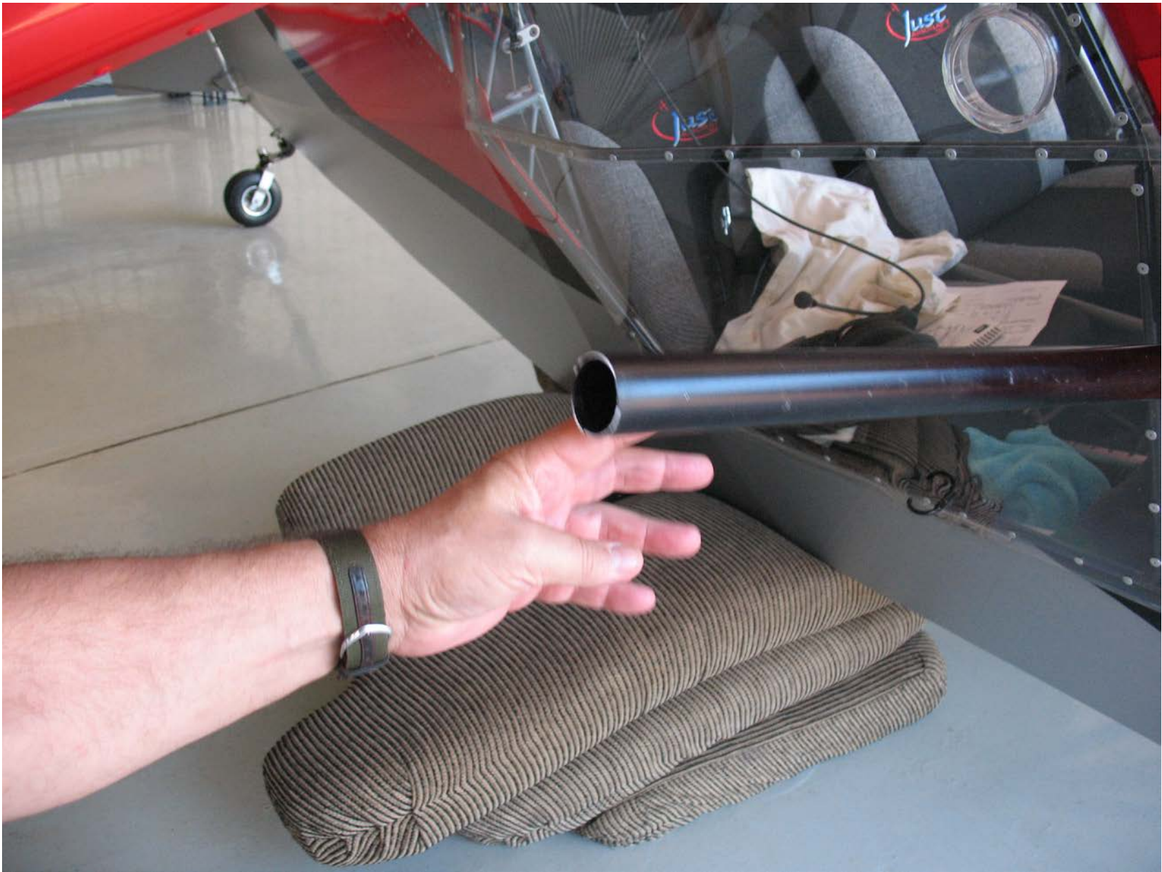
Photo 2 – Fractured right strut
