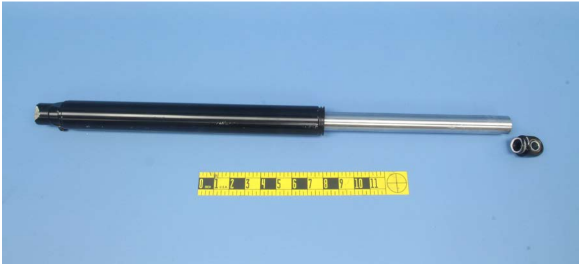
Figure 1: Left landing gear strut as received.
