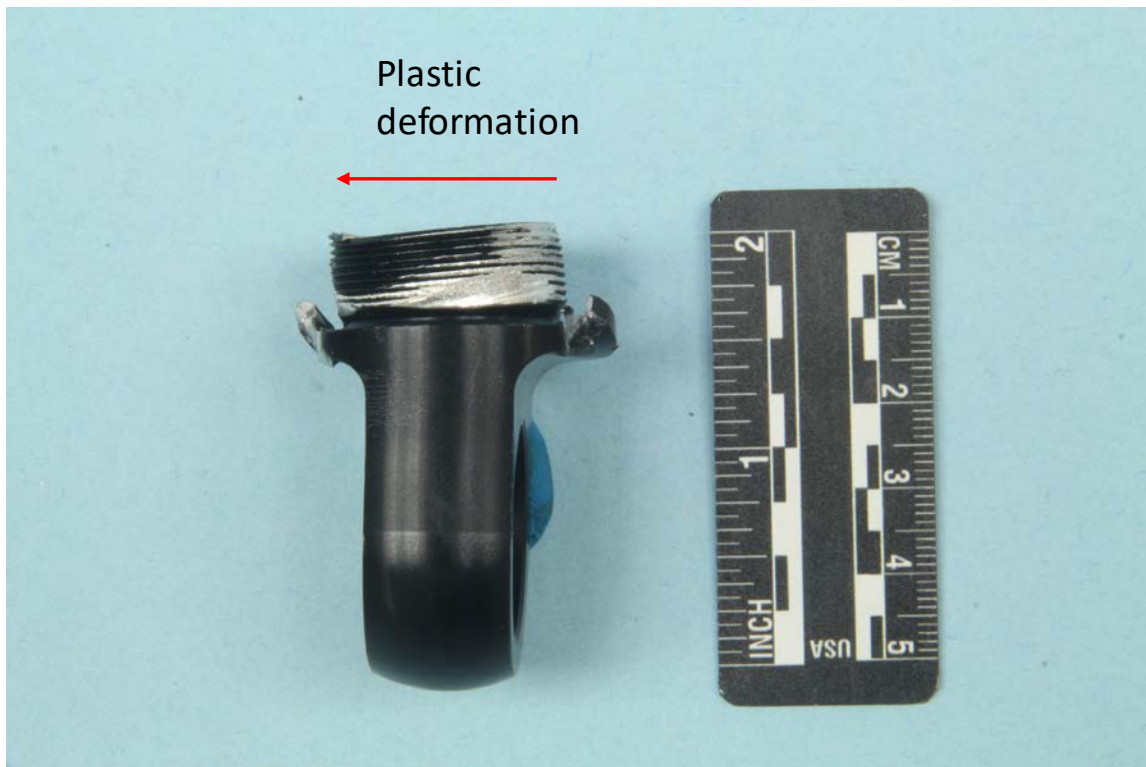
Figure 3: Portion of the end fitting exhibiting plastic deformation.
