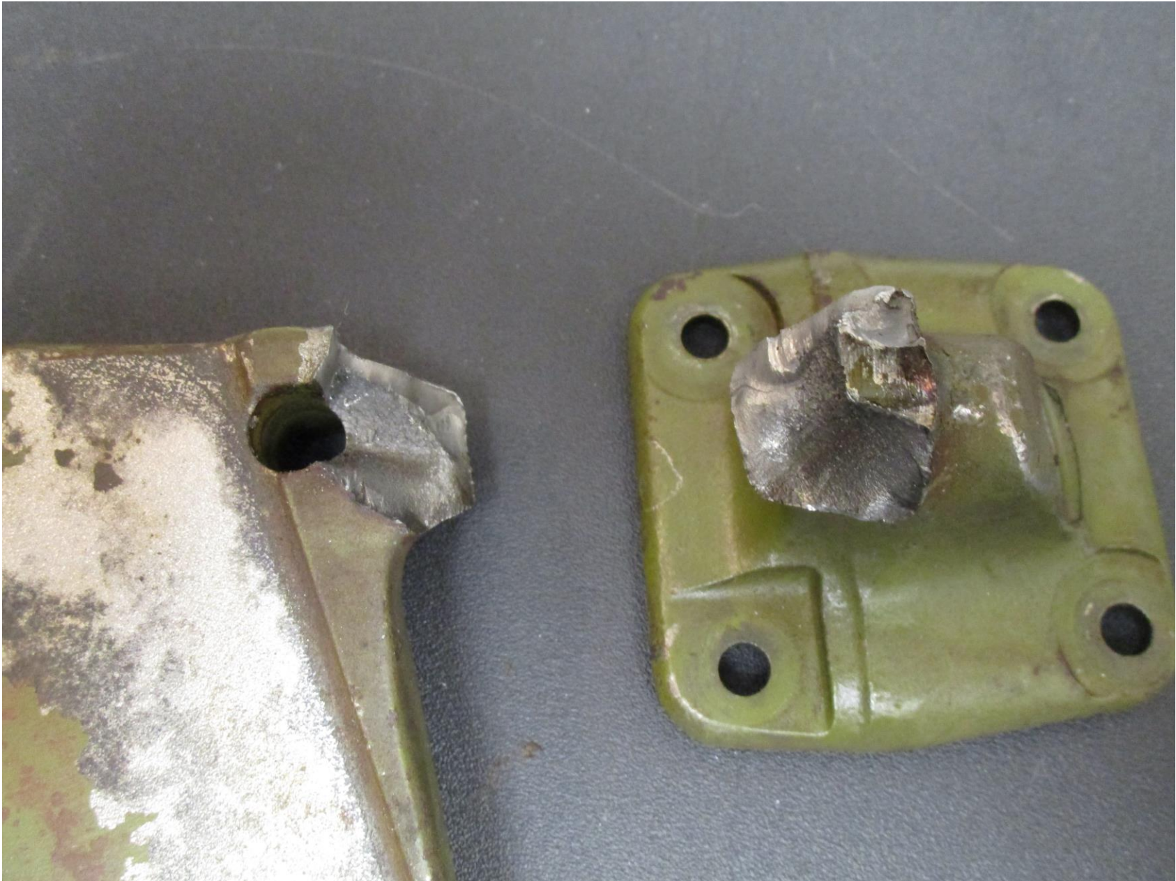
Photo 3 - View of broken left landing gear saddle after removal (photo courtesy of the FAA).
