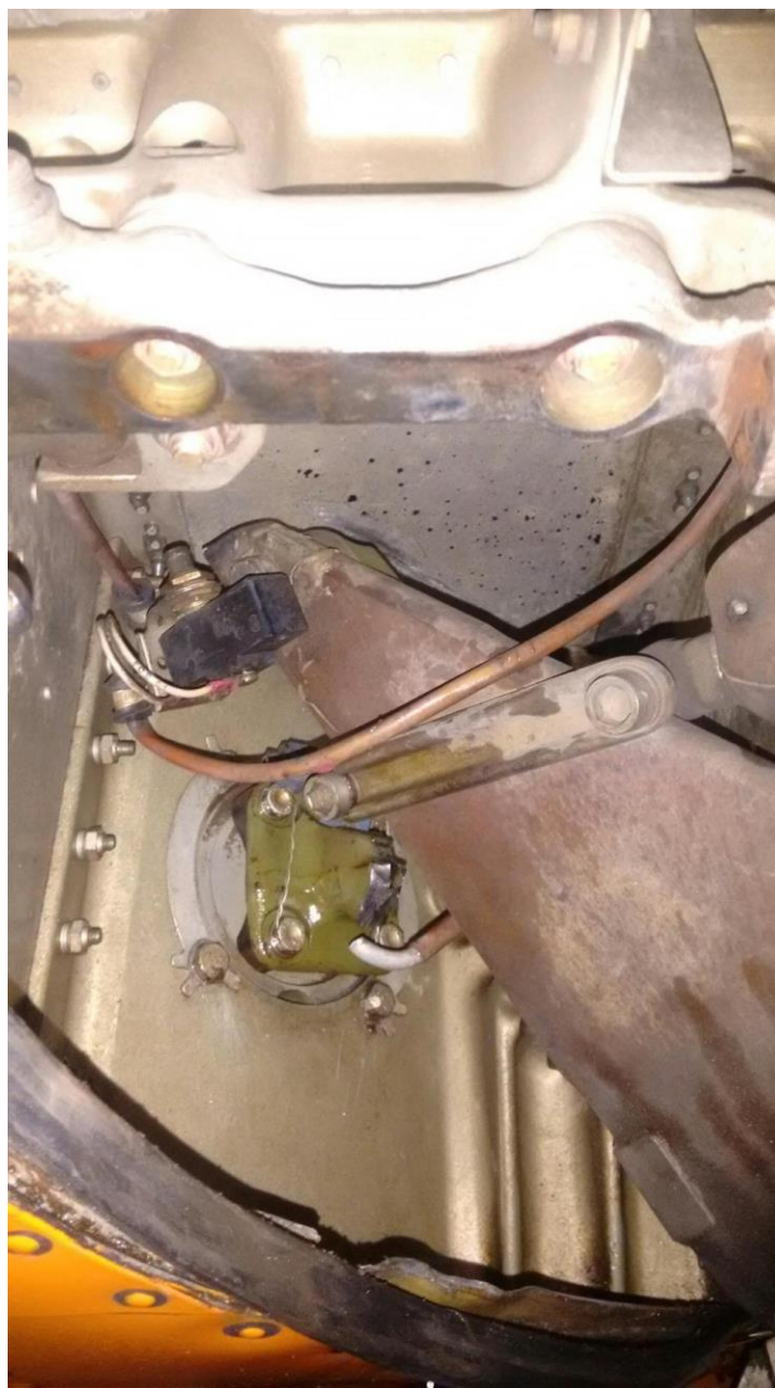
Photo 2 - View of broken left landing gear saddle (photo courtesy of the FAA).
