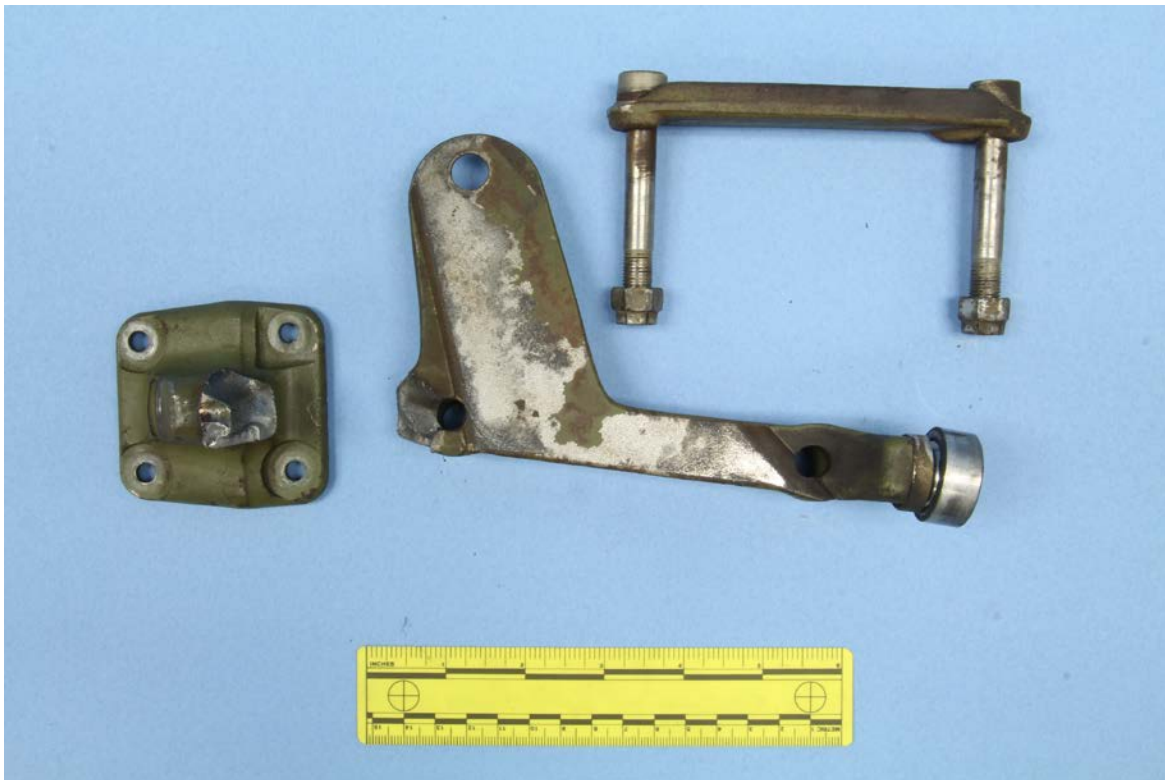
Figure 1: Main landing gear saddle assembly as received.
