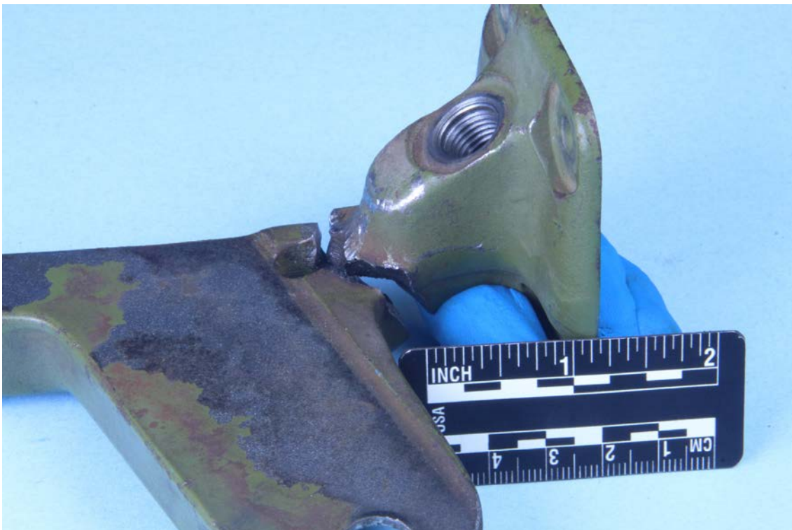
Figure 2: Portions of the saddle assembly showing the orientation of the fracture.
