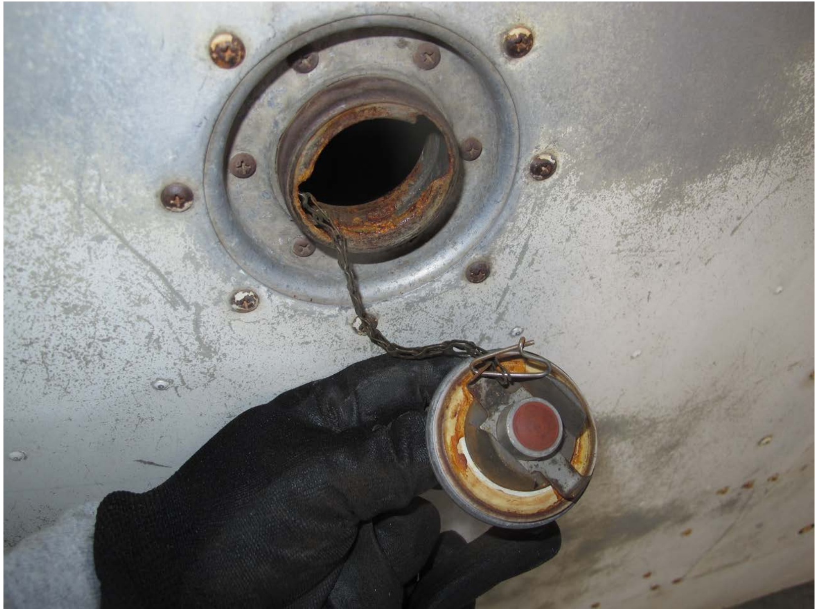
Photo 6 – Right Fuel Tank Cap (Courtesy of Textron Aviation)
