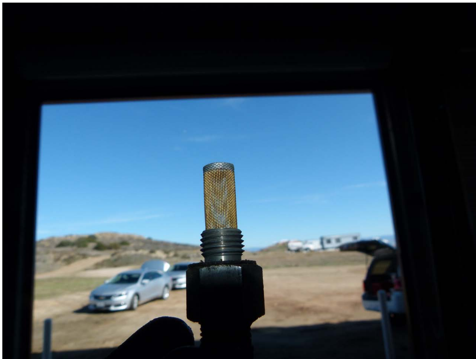
Photo 5 – Carburetor Fuel Inlet Screen (Courtesy of Continental Motors)
