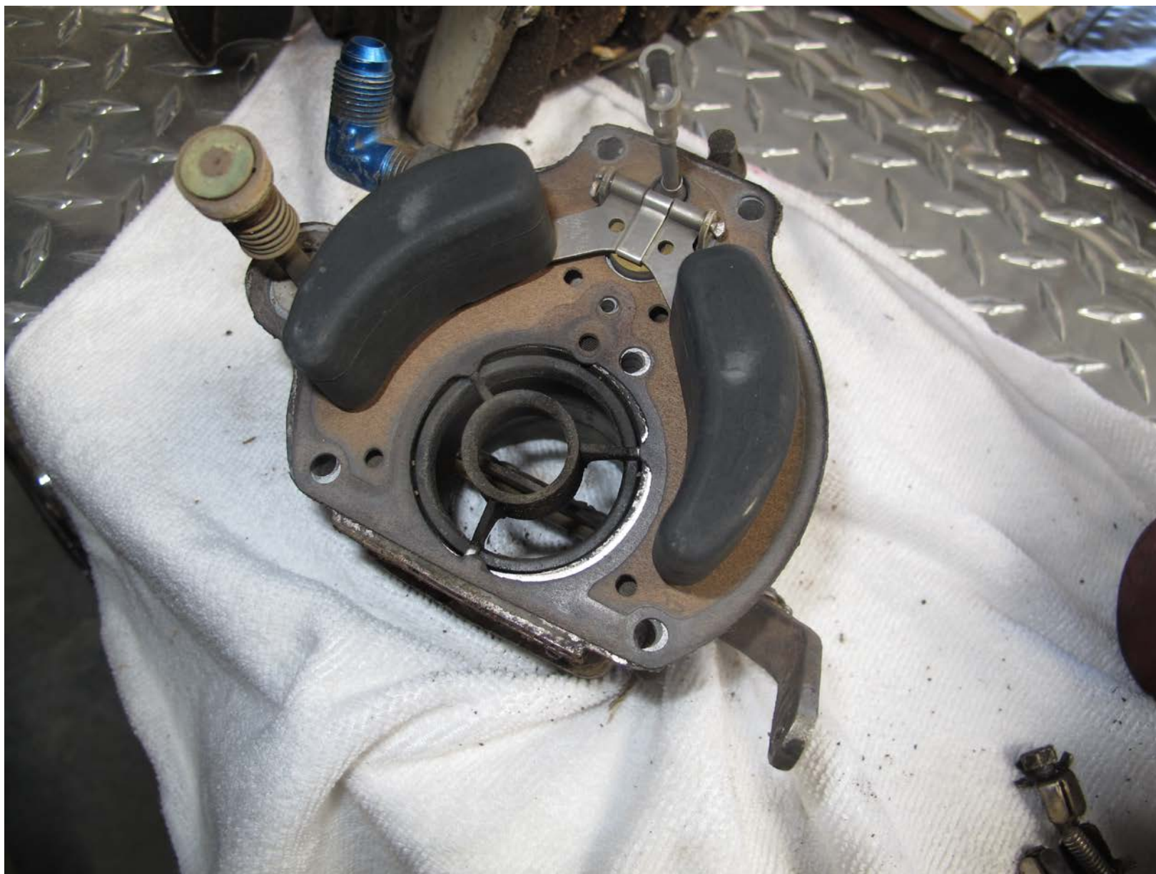
Photo 7 – View of Carburetor Floats and Accelerator Pump (Courtesy of Textron Aviation)
