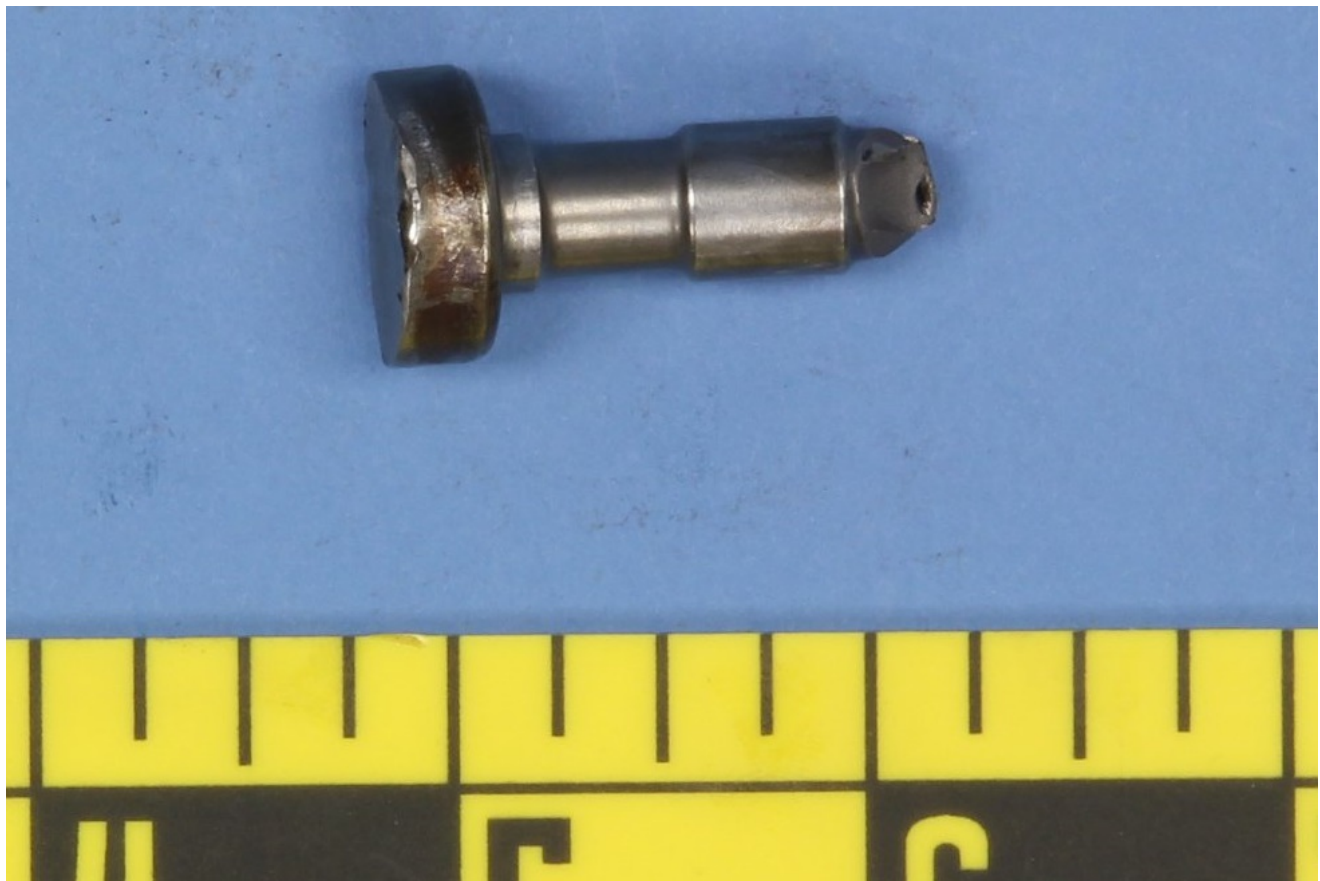
Figure 5 – Side view of the fractured connecting rod bolt, as received.
