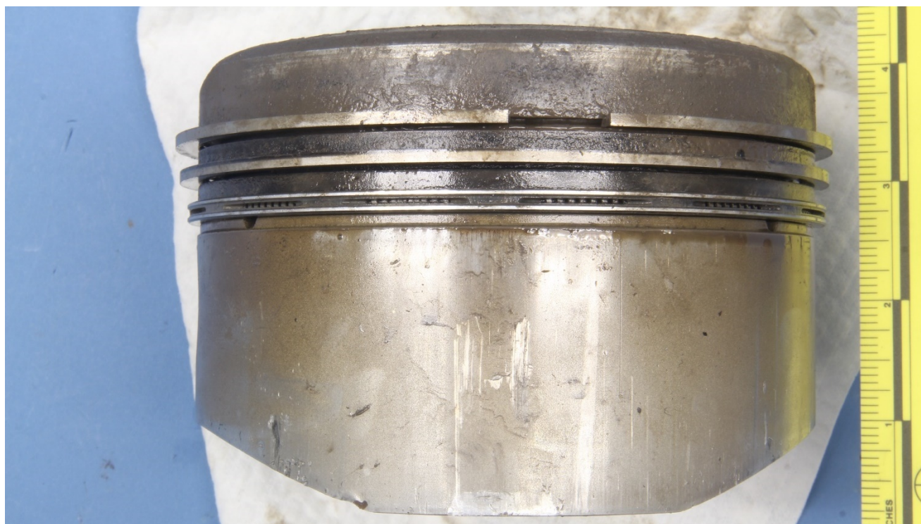
Figure 11 – The side of the piston, after disassembly, showing the scraper and oil rings, and vertical scuff marks on the piston skirt.
