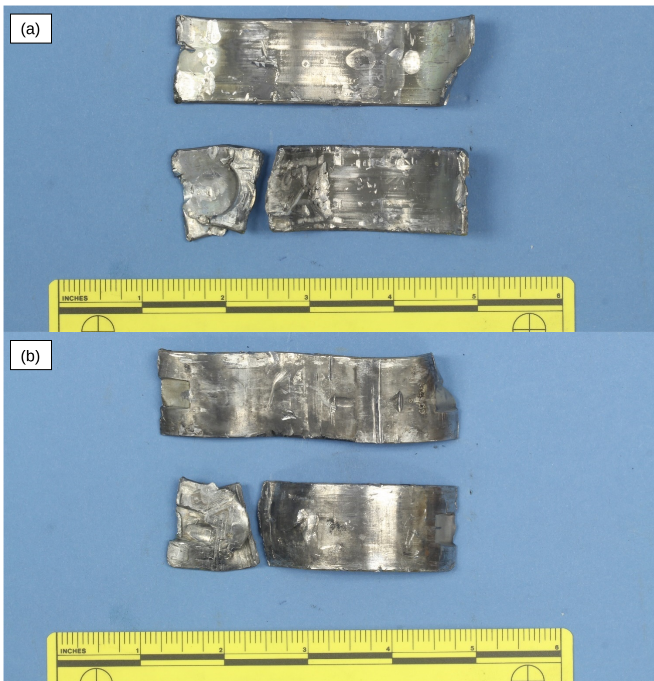
Figure 1 – The pieces of both halves of the connecting rod bearing, as received, from the (a) inner bearing surface and (b) outer bearing surface.
