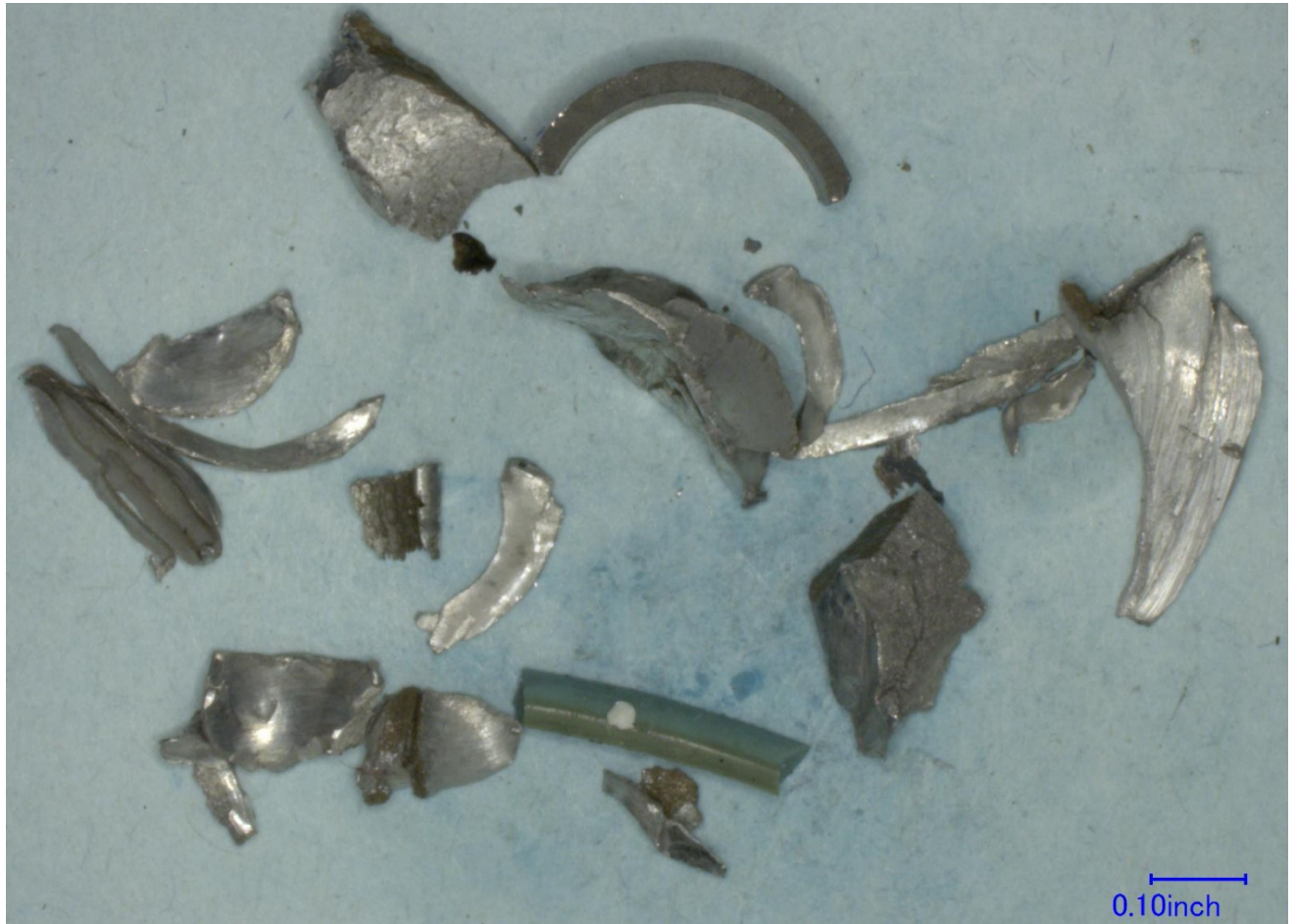
Figure 21 – View of the fragments from the bag of debris, shown after cleaning with acetone.
