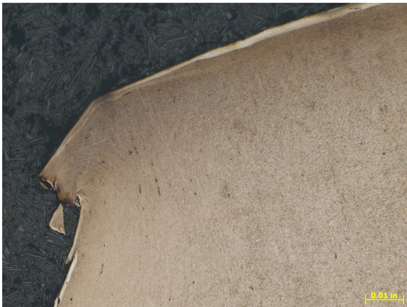
Figure 16 – Bright field (BF) optical micrograph of the cross section in Figure 15, showing grain flow from severe deformation, and a surface white layer (~50X, etched 2% Nital).
