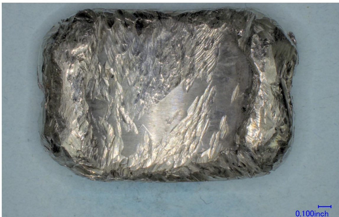
Figure 14 – View of the battered fracture surface of the connecting rod from the bearing surface.
