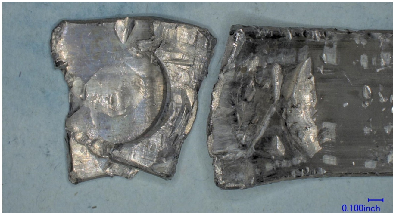
Figure 3 – The mating fracture faces of the fractured bearing half, showing a circular impact imprint.
