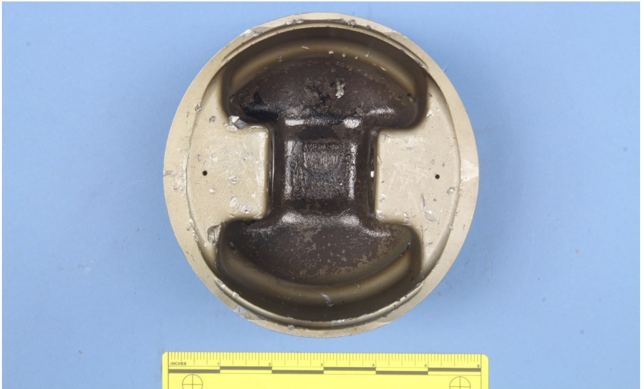
Figure 9 – Underside of the piston, after disassembly.
