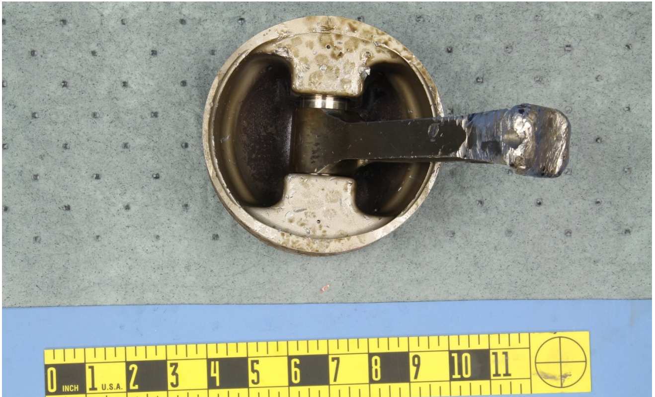
Figure 7 – The underside of the piston assembly, with the connecting rod fragment still attached via the piston pin.
