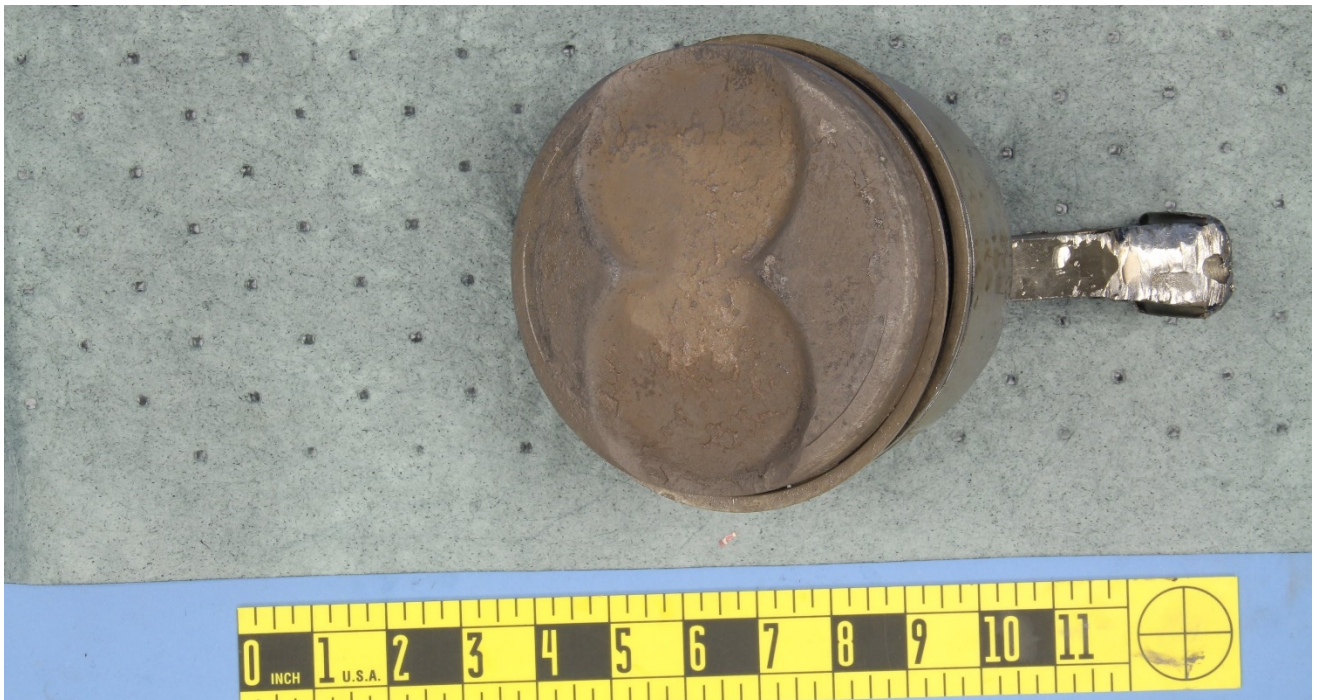
Figure 8 – Reverse view of Figure 7, showing the crown of the piston and the other batter damage to the connecting rod.
