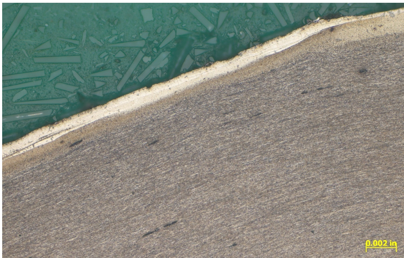
Figure 17 – BF micrograph showing the surface in Figure 17, showing grain flow perpendicular to the forging direction of the connecting rod, and white layer consistent with untampered martensite (~200X, etched 2% Nital).
