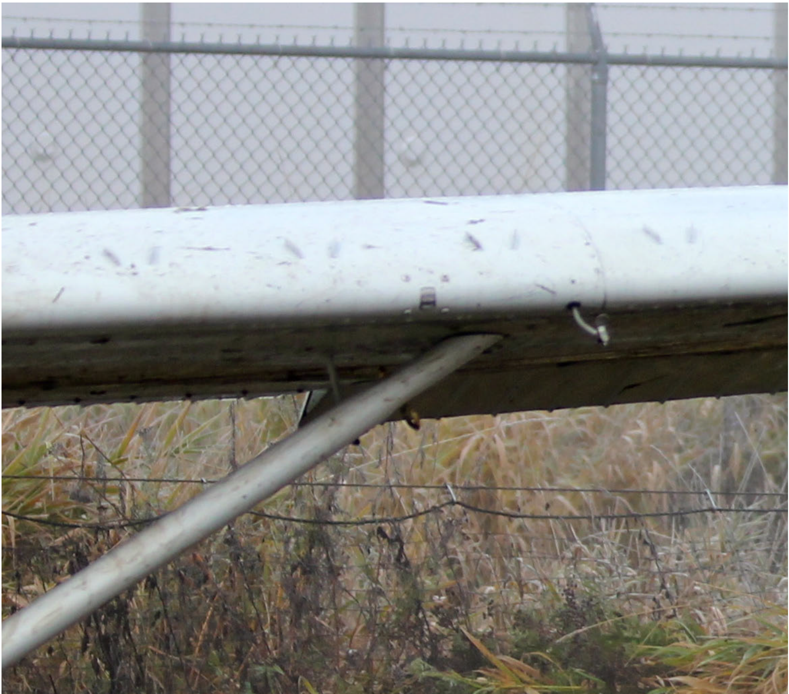
ILLUSTRATION # 4 b – Left wing. Magnification of inner edge of aileron relative to flap trailing edge
