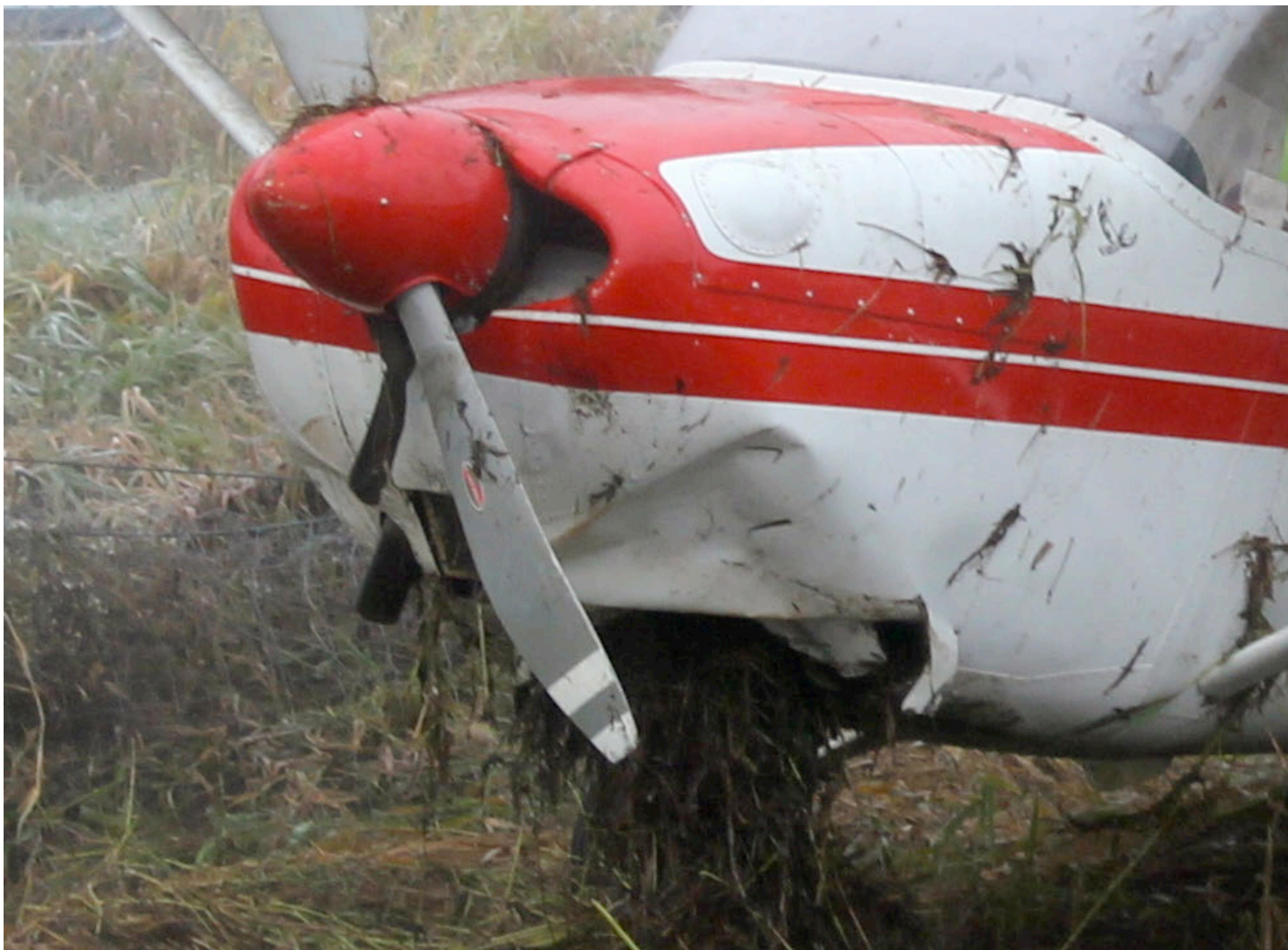
Illustration # 3 – Front of firewall damage.
