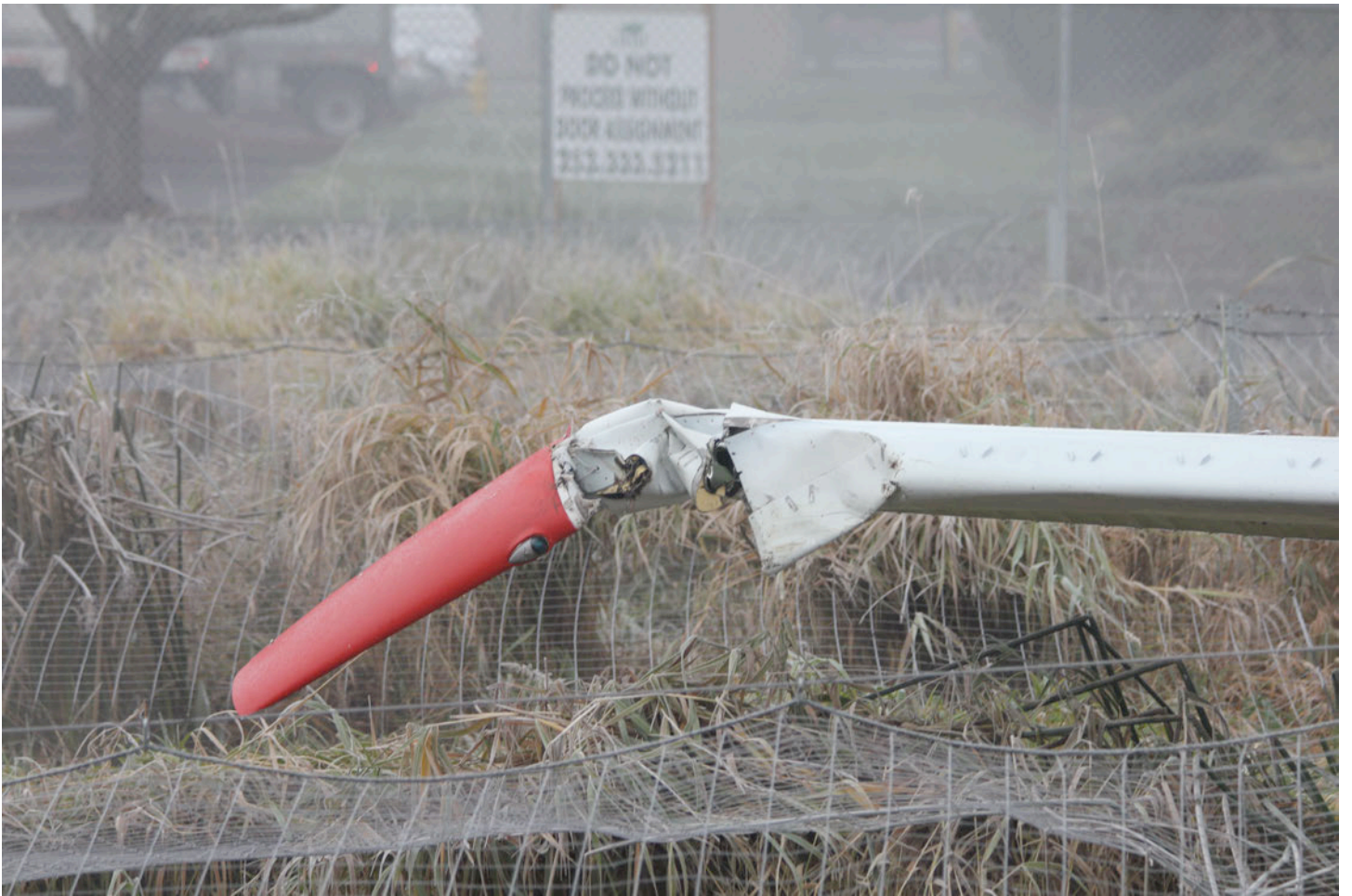
Illustration #4 – Right Wing tip broken
