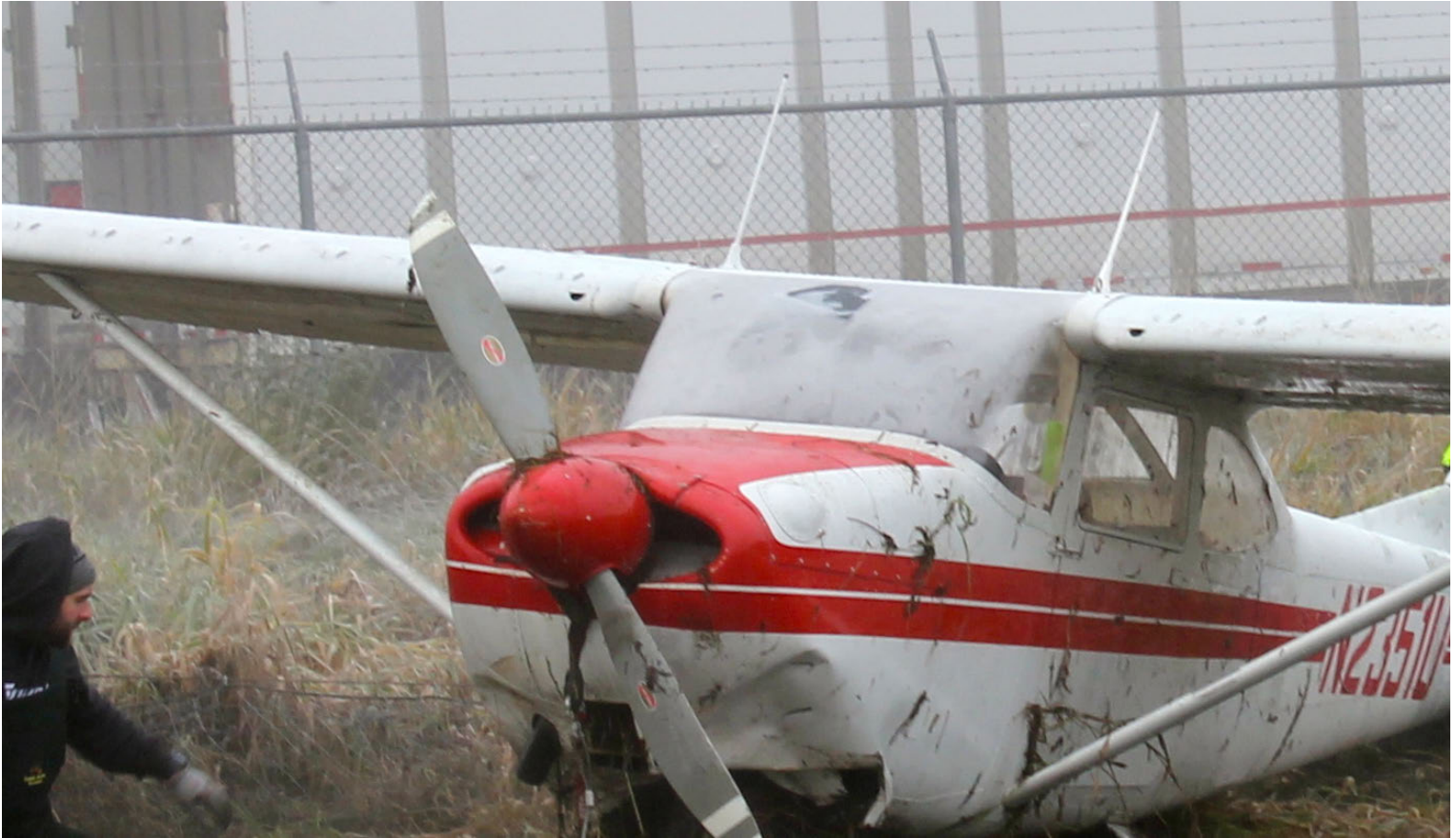
ILLUSTRATION # 3 – Frontal view; trailing edge of right flap noticeably below the left flap trailing edge. Flap Setting at 0 degrees.
