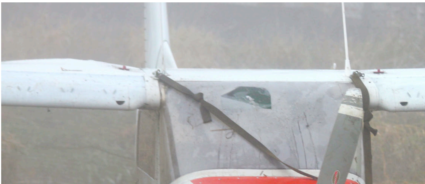
Illustration #2 – Severe buckling of right wing at root. Note the fuel tank cap on right side
