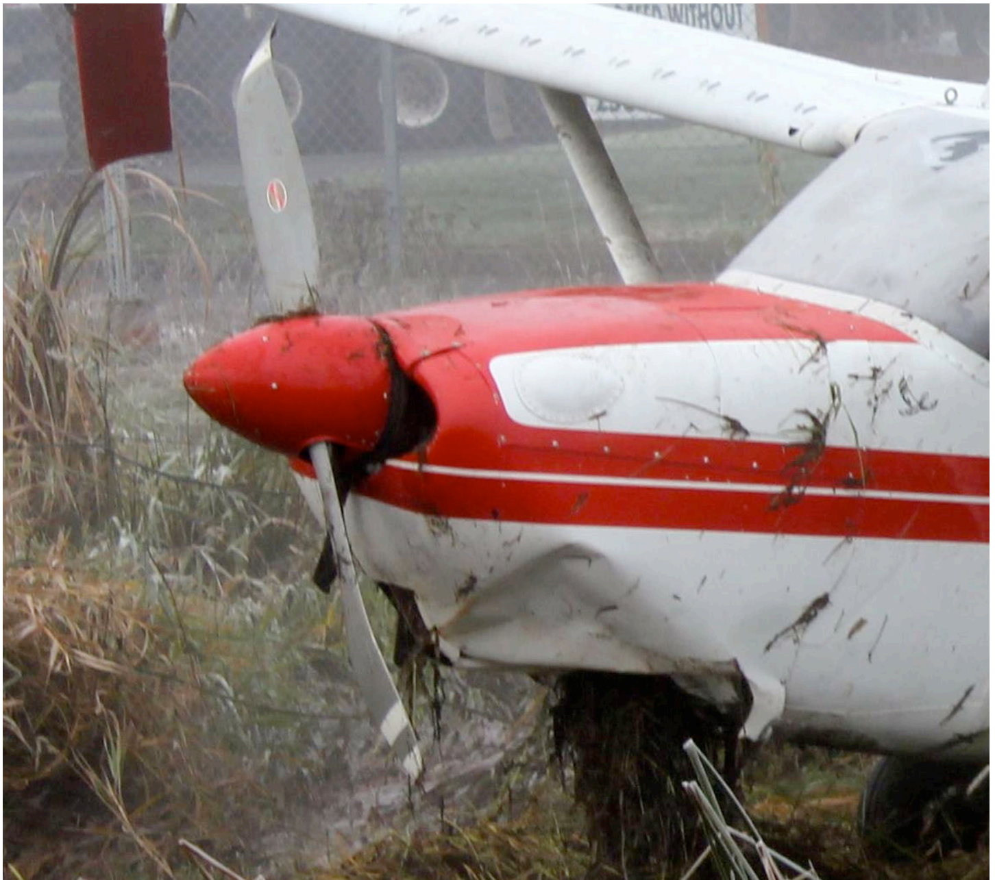
ILLUSTRATION #1 – Prop Strike -Propeller Blades bent
