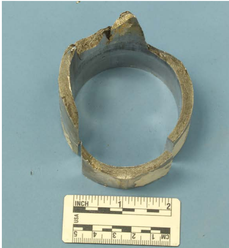
Figure 3: A sample containing the flat fracture area was cut from the remainder of the fracture surface.
