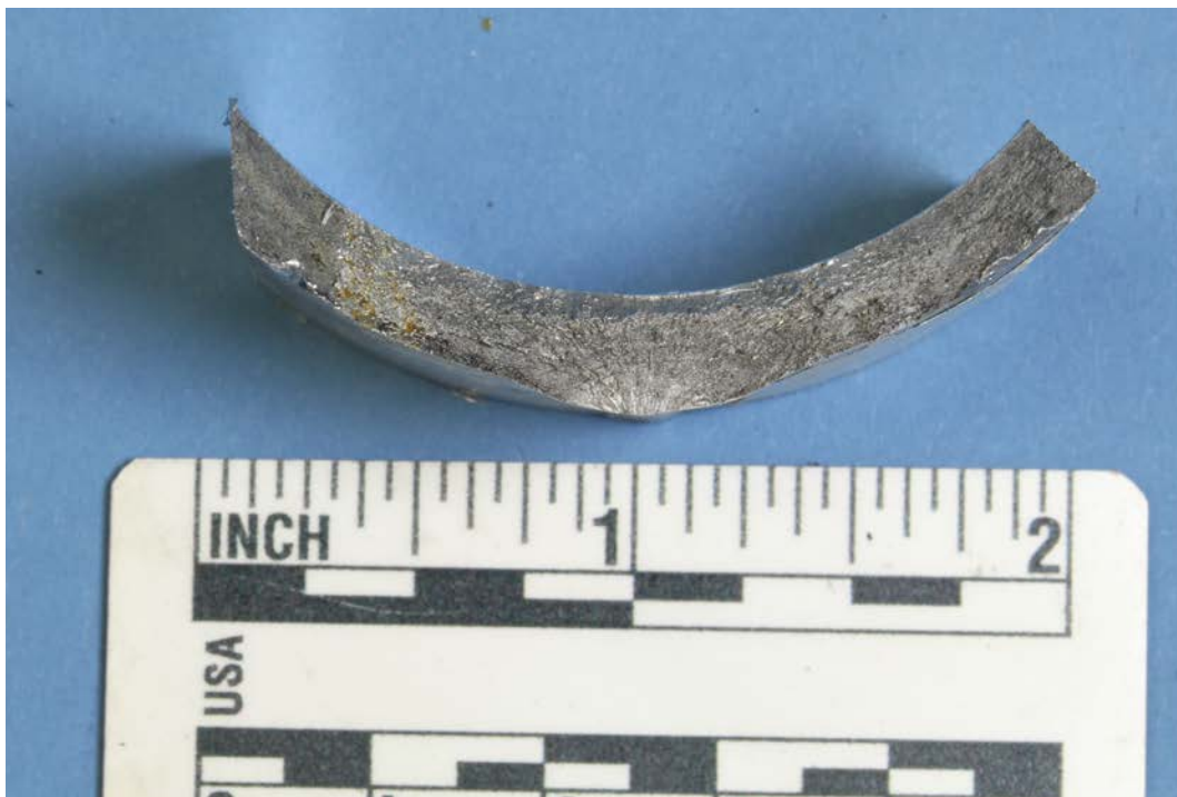
Figure 4: close-up of the sample containing the flat fracture area.
