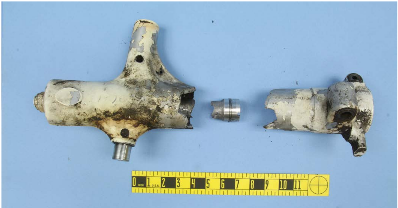
Figure 1: Portions of the left landing gear strut as received.
