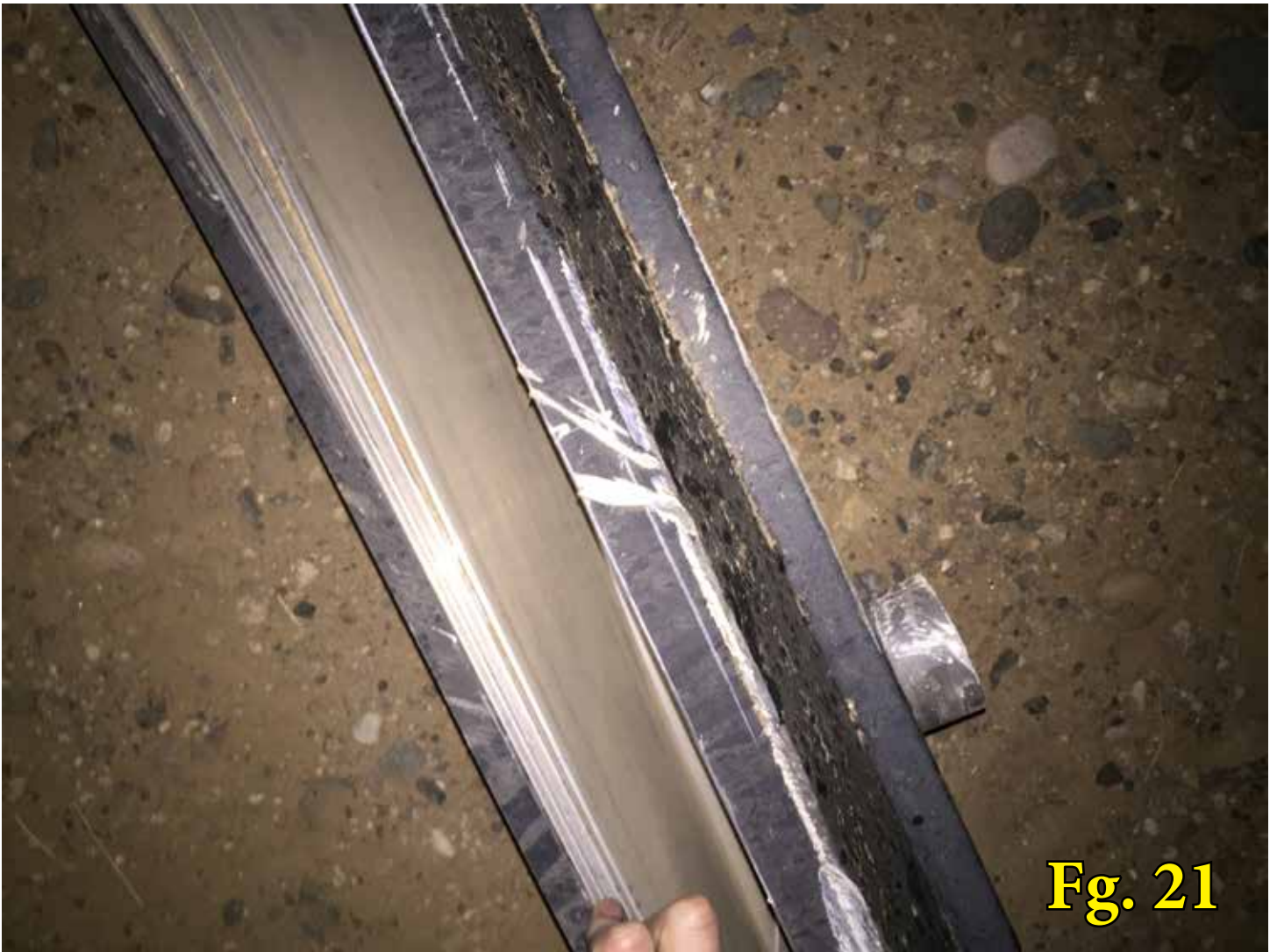
Prop strike damage to the runway sign which clearly shows that there was not gear failure at this point of the incident.
