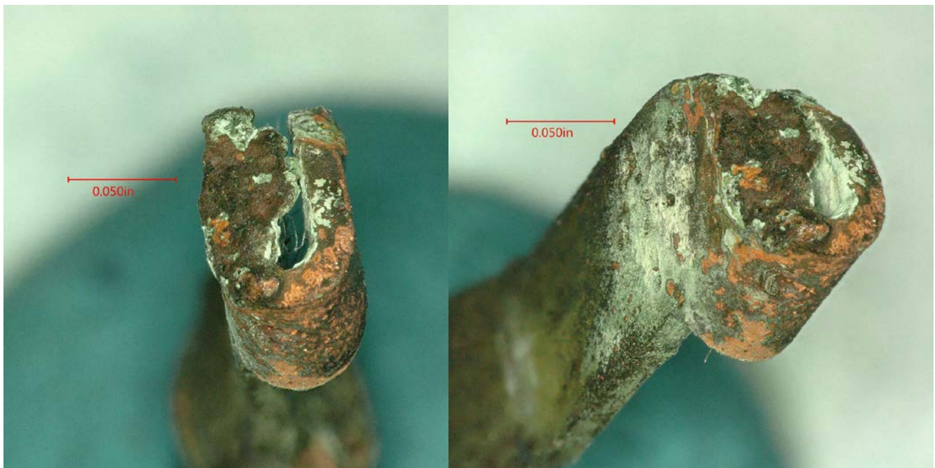
Figure 7: Terminal connector exhibiting electrical arc erosion.
