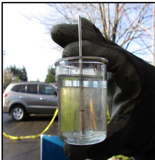
Figure 1: Fuel drained from the main strainer.
