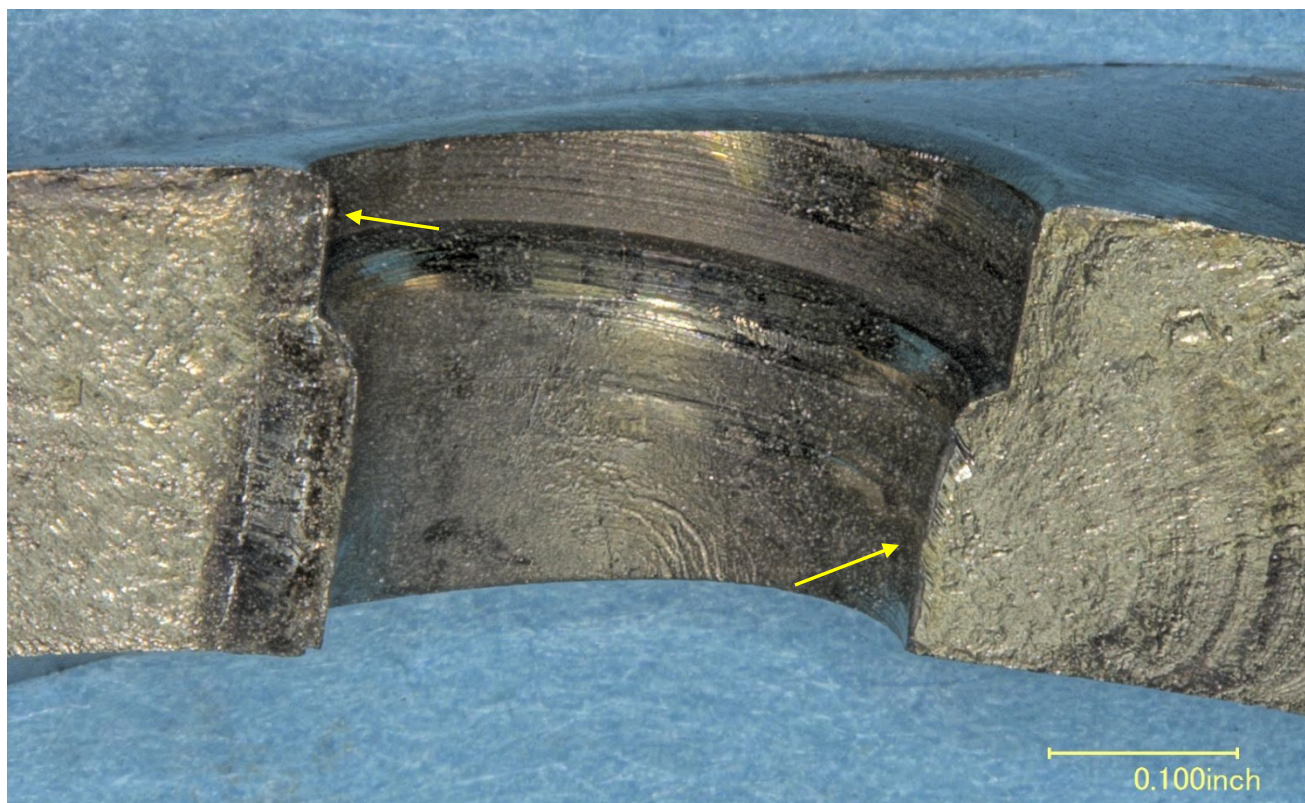
Figure 10 – The crack initiation sites of the main journal fracture at the lubrication hole in Figure 9. The two arrows depict the fatigue crack initiation sites.
