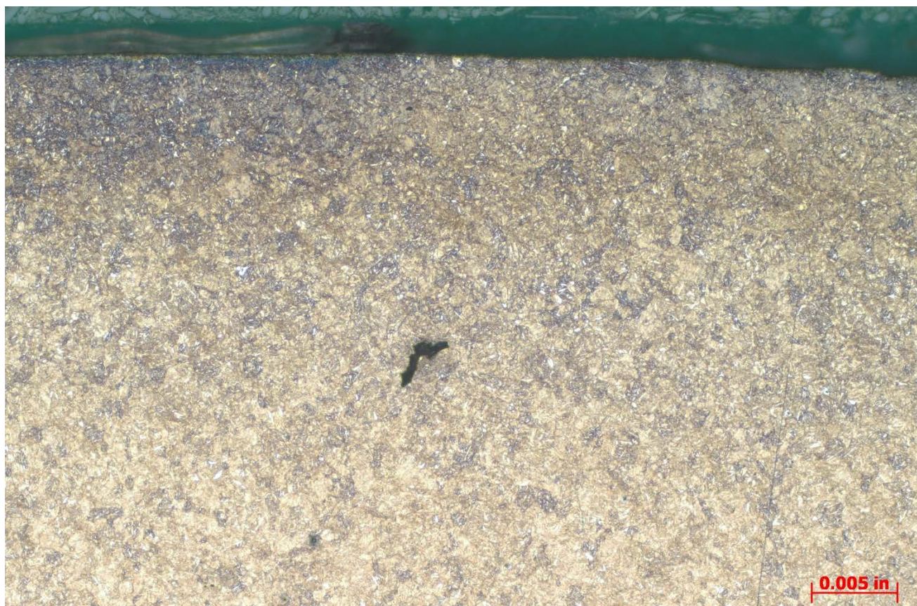
Figure 15 – Bright-field (BF) optical micrograph of the crankshaft main journal surface (~100X, etched 2% Nital).
