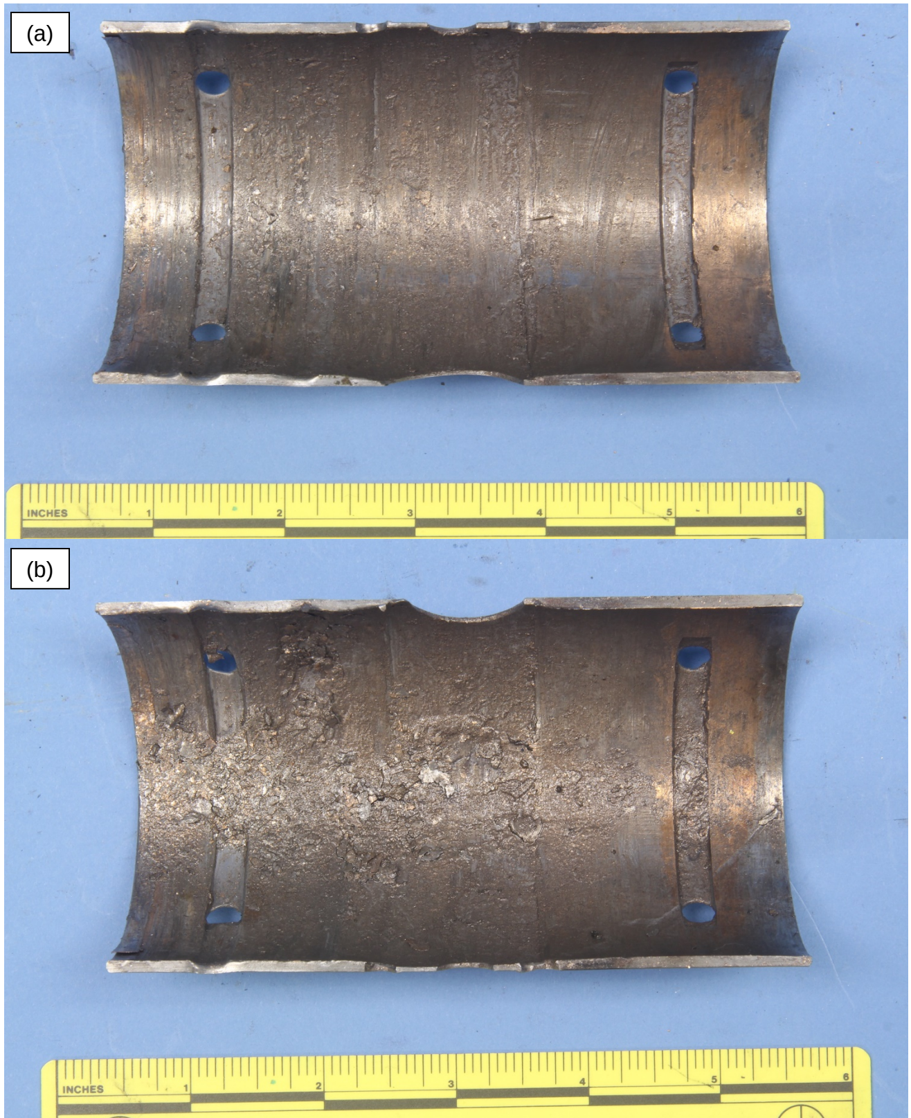
Figure 18 – The main journal bearings, viewed from the inside bearing surface which exhibited wear and material spalling.
