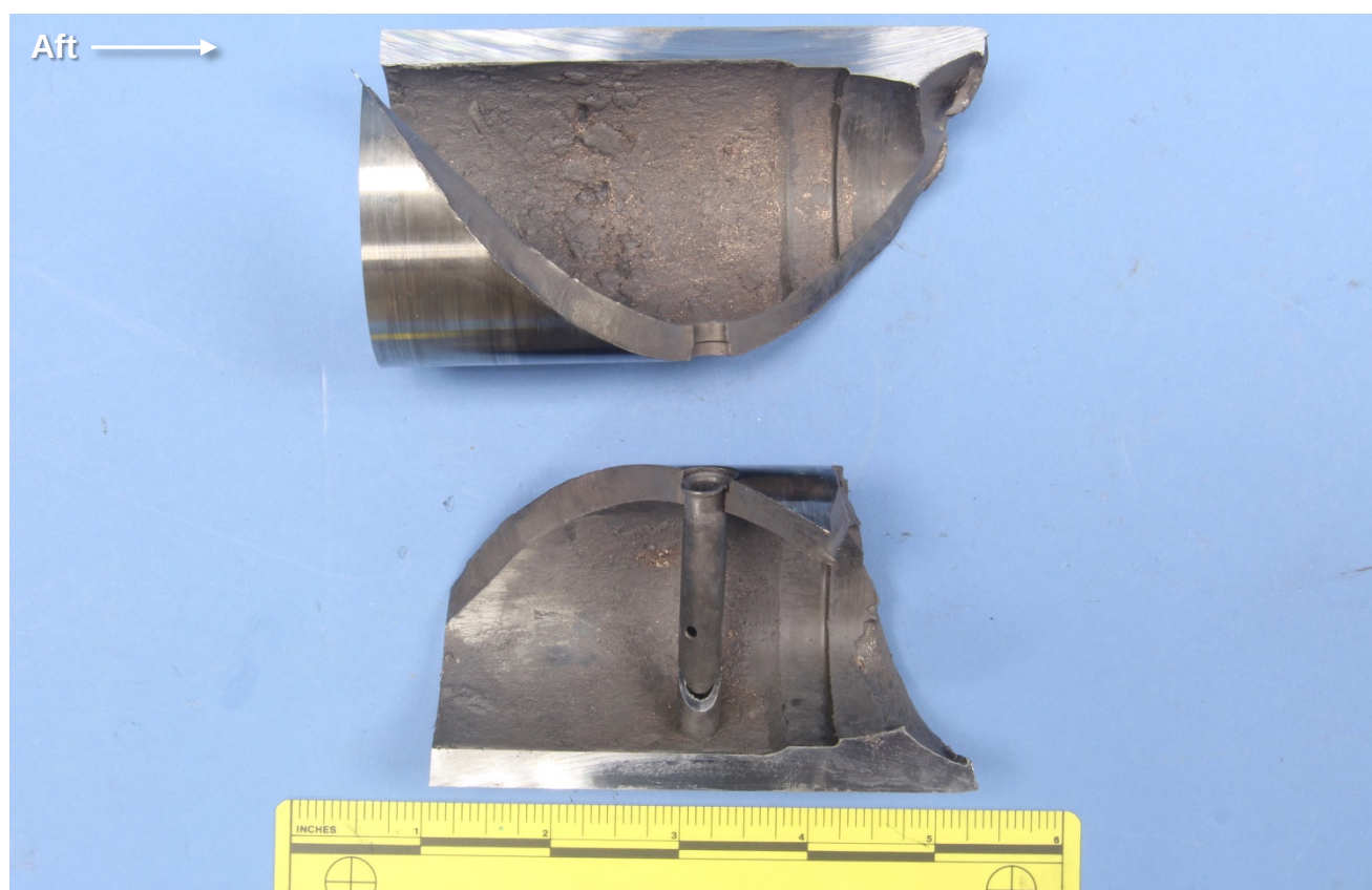
Figure 6 – The crankshaft journal in Figure 5, after opening to expose the spiral fracture. The sludge tube is on the bottom section, with a small cut artifact from the crankshaft sectioning.
