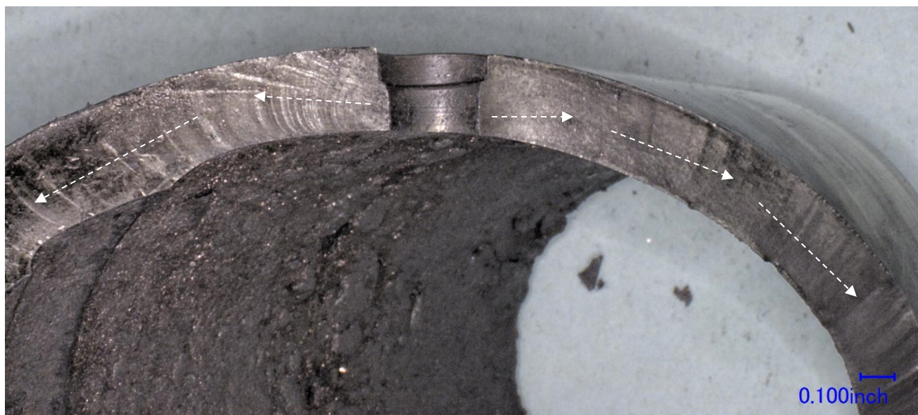
Figure 7 – The fracture surface from the upper section in Figure 6, showing crack arrest marks emanating from the lubrication hole. Dashed white arrows depict the crack propagation direction from the oil hole.
