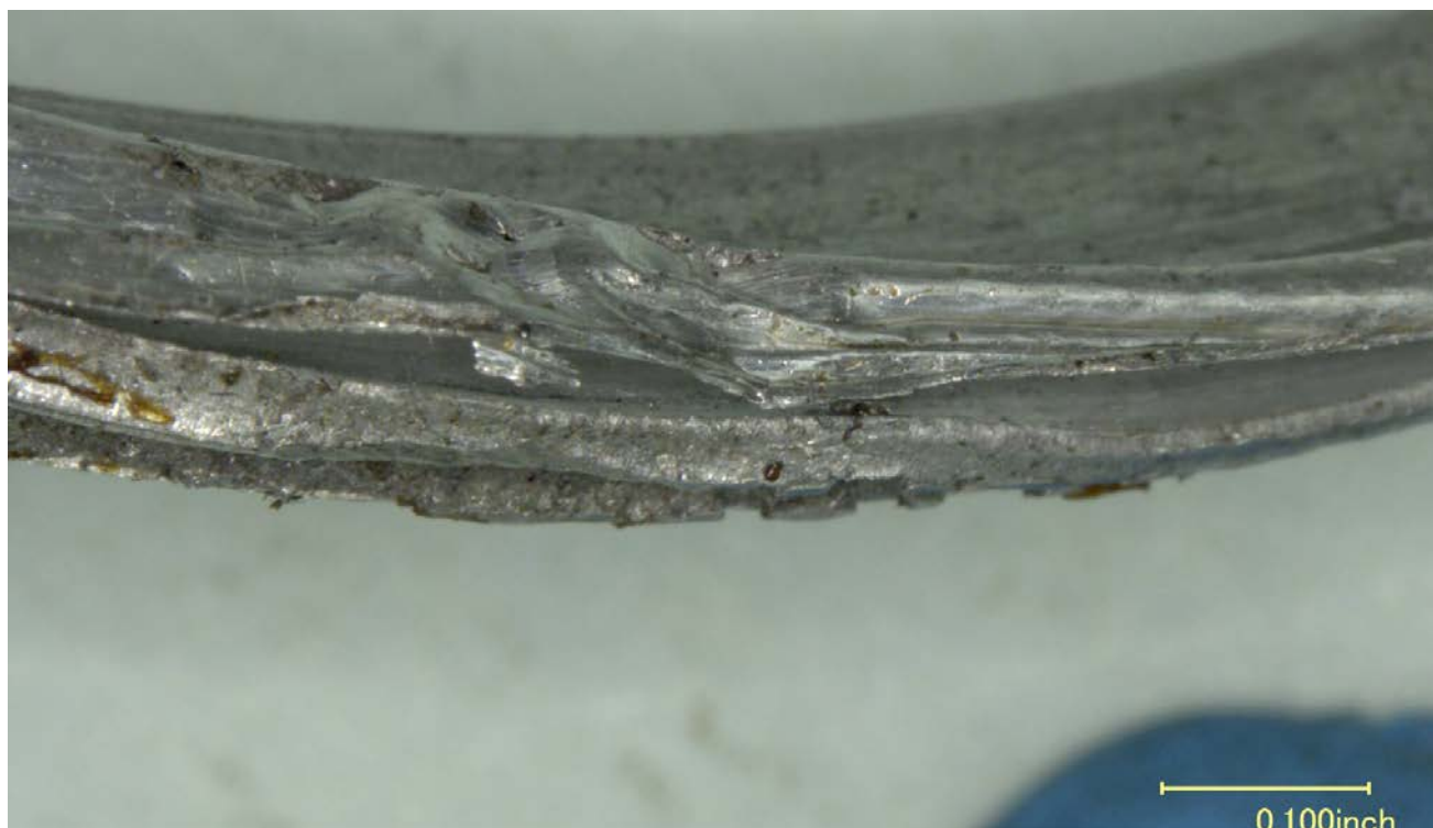
Figure 22 – Damage on the edge of one of the flanges.
