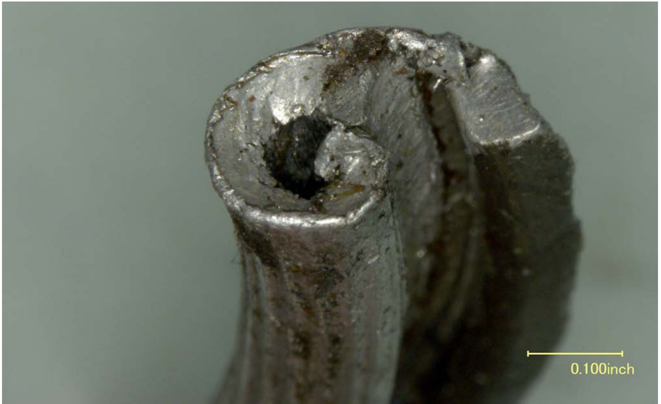
Figure 23 – Deformation on one of the flanges severe enough to curl over on an edge.
