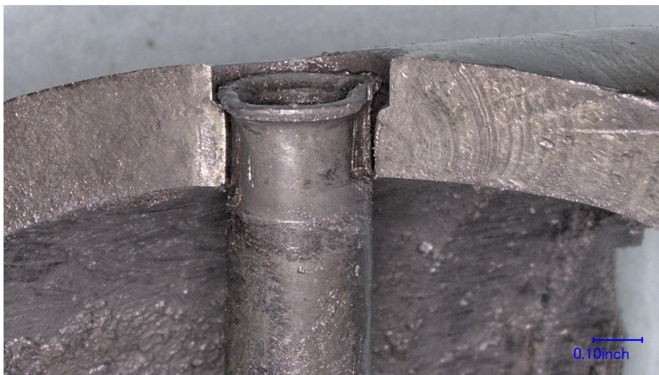
Figure 8 – The fracture surface from the lower section in Figure 6, showing crack arrest marks emanating from the lubrication hole, which still had the oil tube in place.
