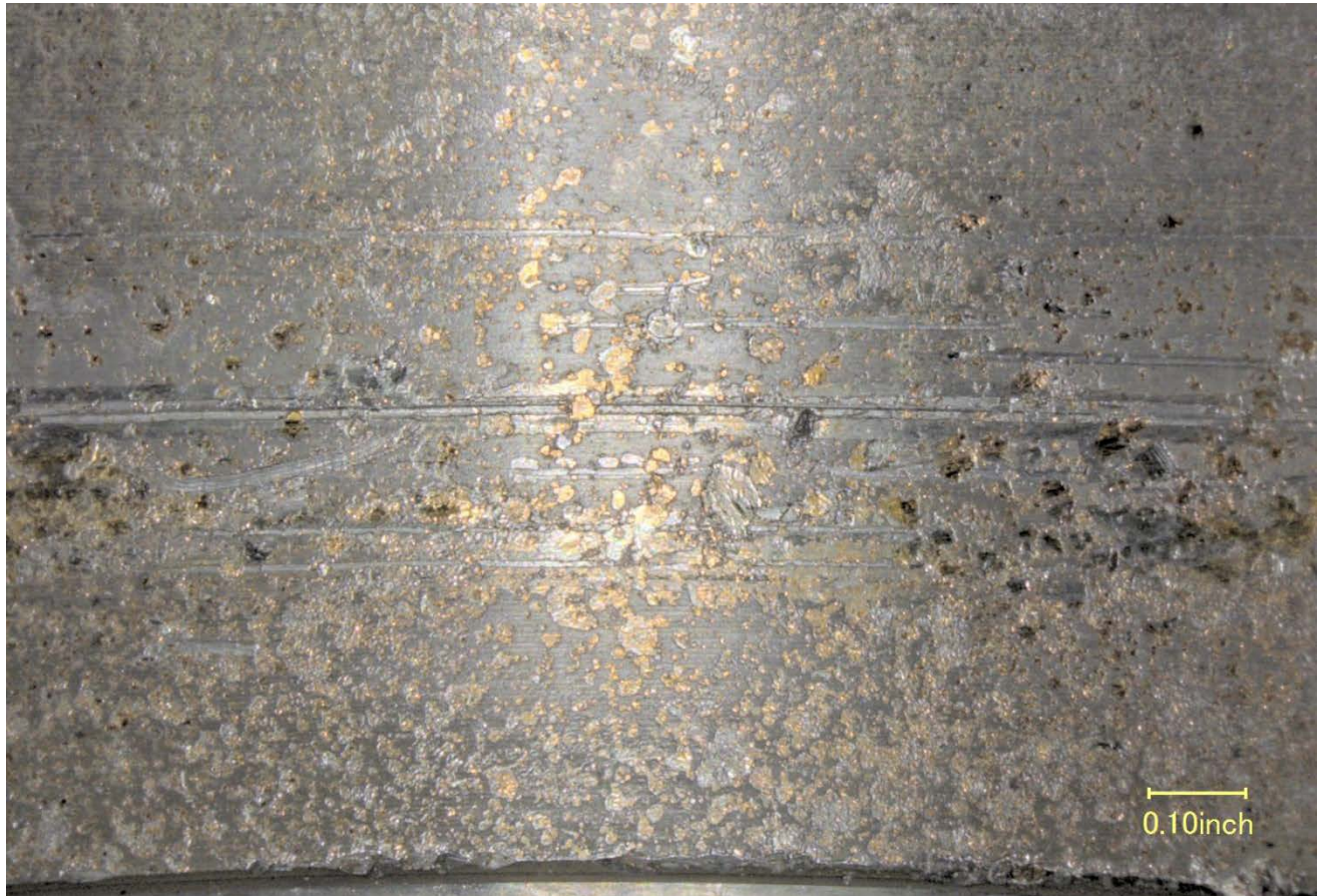
Figure 25 – The inner bearing surface of the connecting rod cap, showing scrape marks and material spalling.
