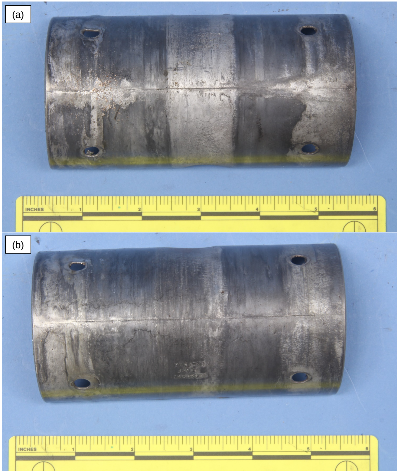
Figure 19 – View of the outer surface of the main journal bearings, showing circumferential wear marks.
