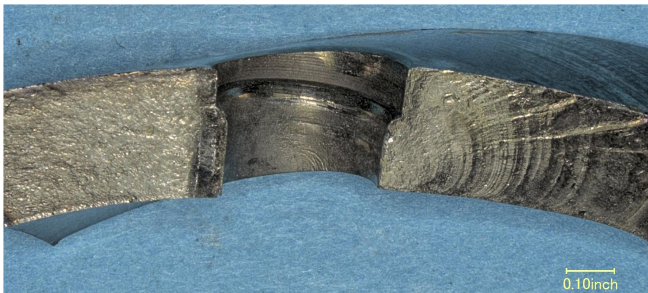
Figure 9 – The sectioned and cleaned portion of the journal fracture surface in Figure 8.
