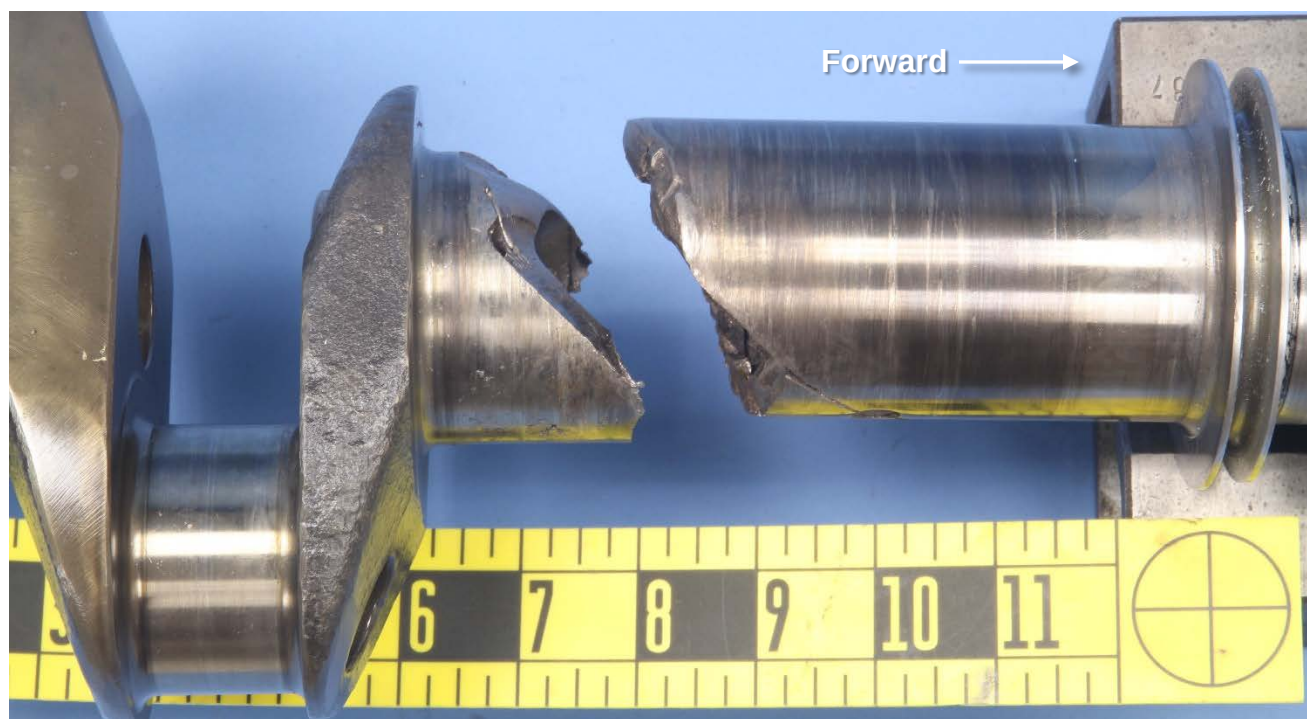
Figure 3 – View of the fractured portion of the crankshaft main journal, rotated 90° from Figure 2.
