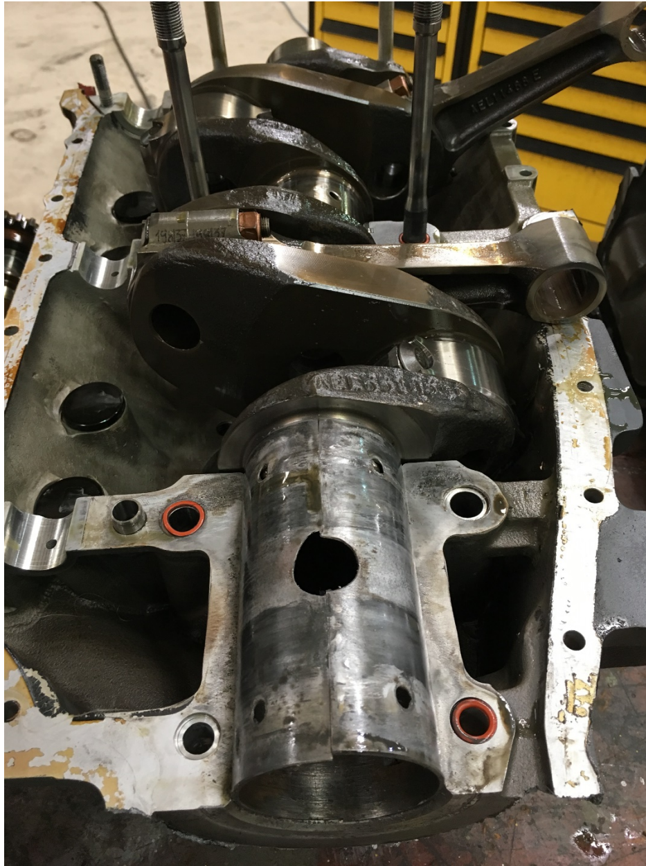
Figure 4: Split engine case with crankshaft (NTSB)
