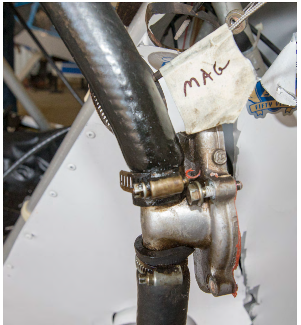
Figure: 4 Hose leak at Water Pump Housing
