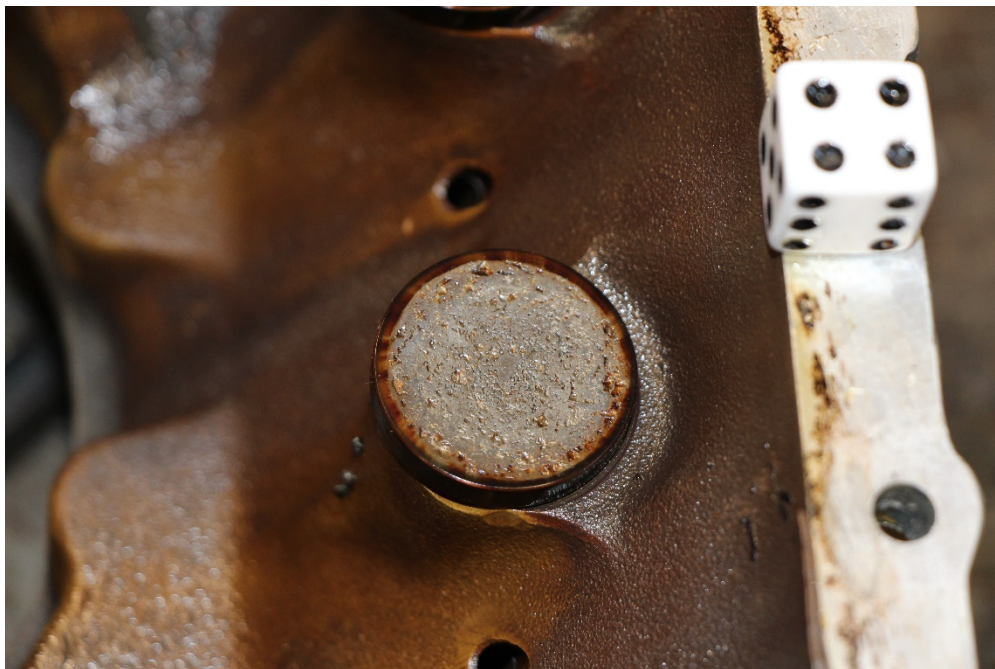
Photograph 13: View of Cam Lifter to Cylinder No. 4 Intake Valve (note spalling)
