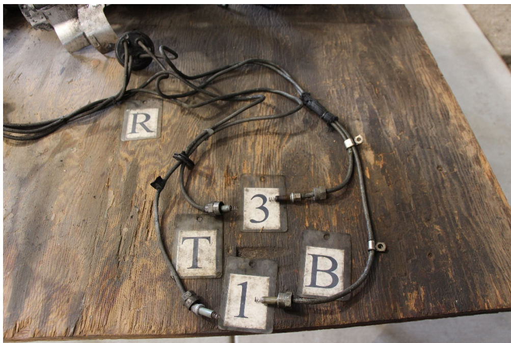
Photograph 5: Top and Bottom Ignition Leads for Cylinder Nos. 1 and 3
