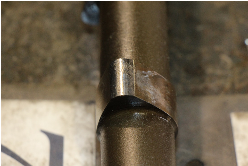
Photograph 12: View of Intake Valve Cam Lobe to Cylinder No. 3 and 4 (note some pitting and wear)
