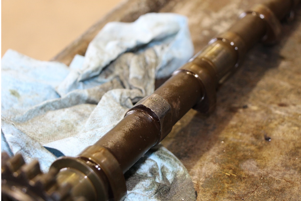
Photograph 10: View of Camshaft and Intake Valve Cam Lobe to Cylinder No. 3 and 4 (note pitting and wear)
