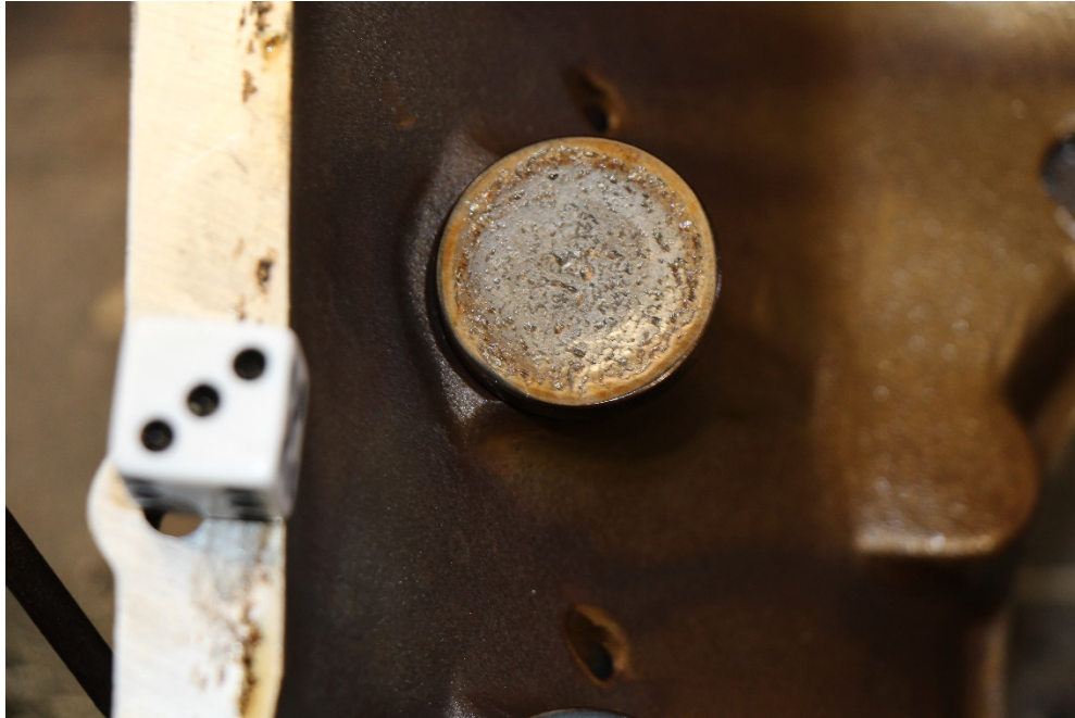
Photograph 14: View of Cam Lifter to Cylinder No. 3 Intake Valve (note spalling and wear)
