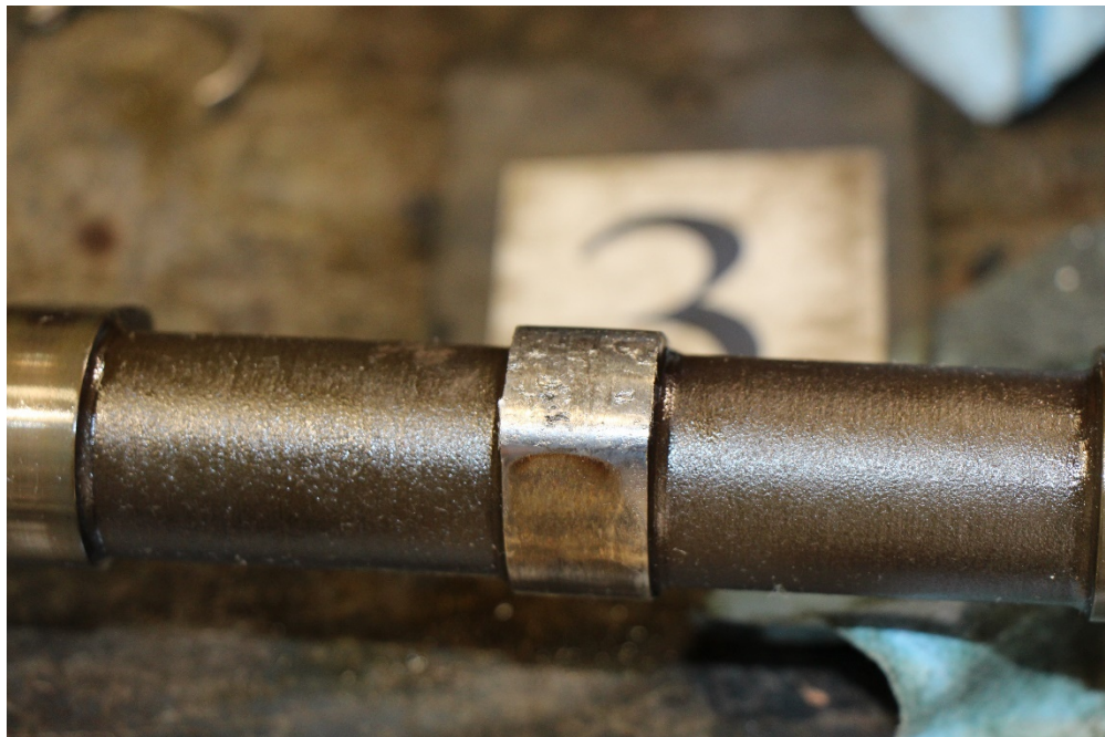
Photograph 11: View of Intake Valve Cam Lobe to Cylinder No. 3 and 4 (note pitting and wear)
