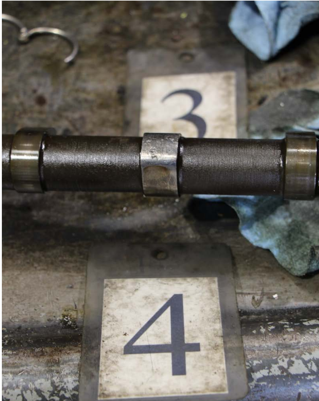
Photo 4 – Camshaft Intake Camlobe for Cylinder Nos. 3 and 4
