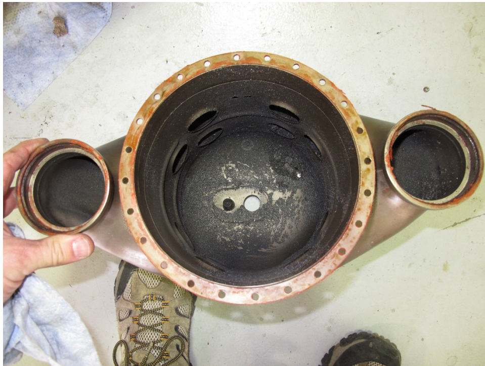
Figure 11: Black debris in Outer Combustion Case
