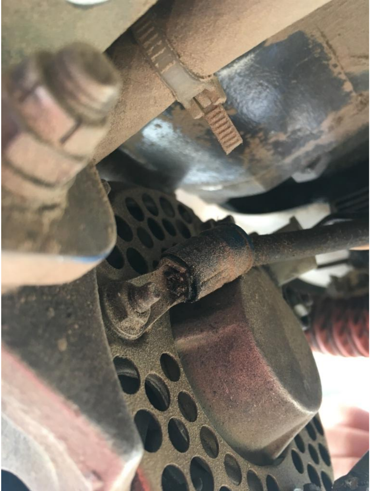
Figure 9 - Alternator Ground Cable Crimp
