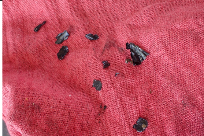
Bearing material found in oil sump
