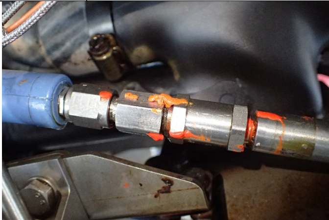
Right turbocharger check valve with loose B-nut
