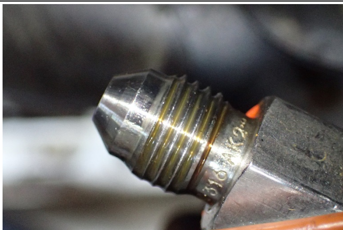
Check valve inlet fitting threads
