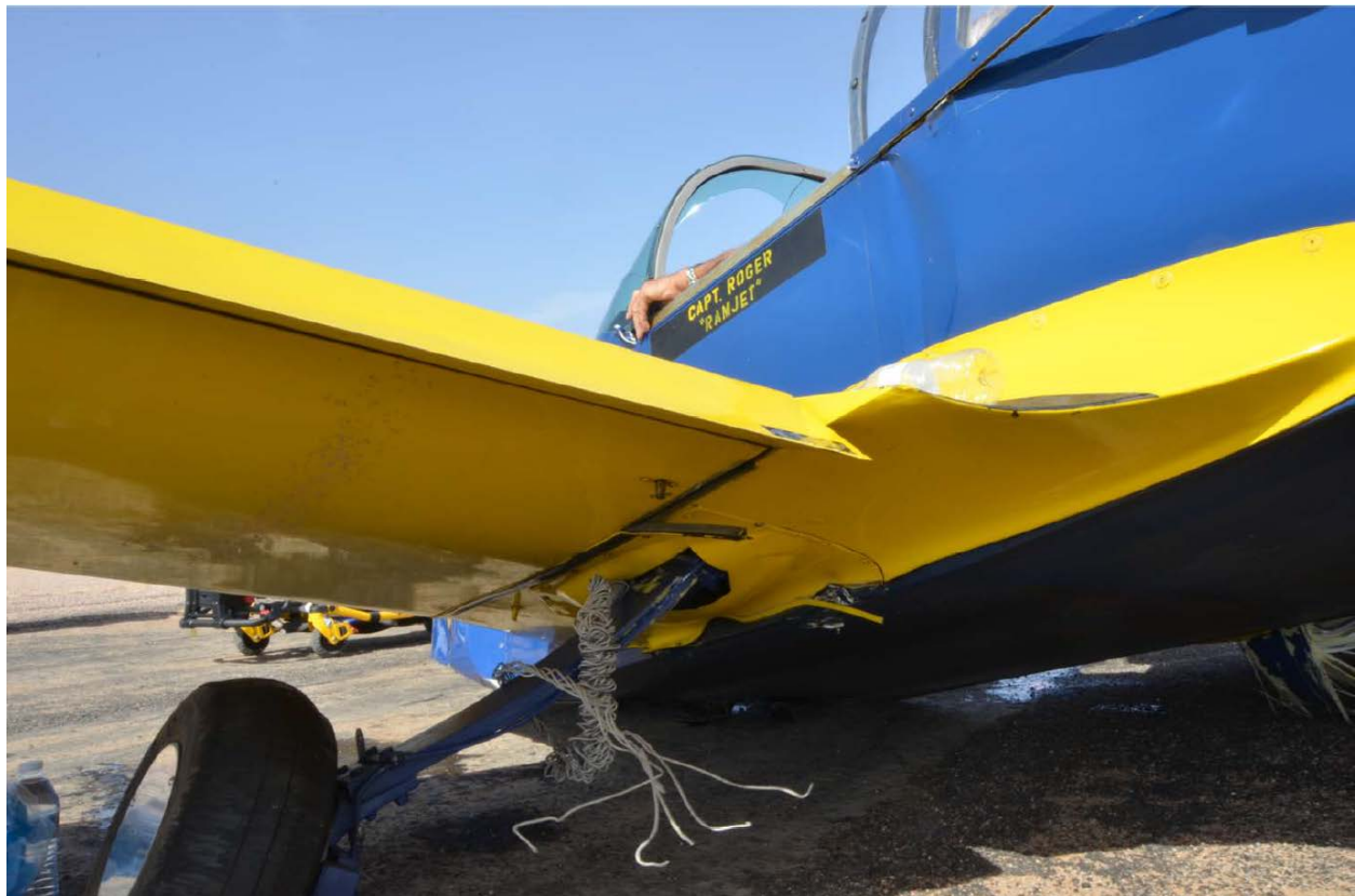
Figure 4: Electrical Wire was found Wrapped around the Main Landing Gear
